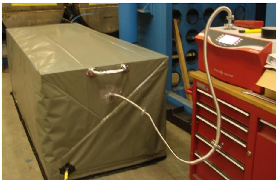
**Figure: Helium cage around the cylinder**
