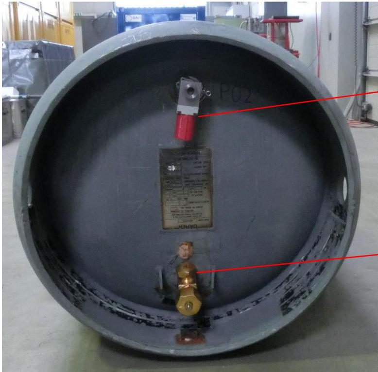
3<sup>rd</sup> orifice for leakage testing (shown with attached vacuum valve)
