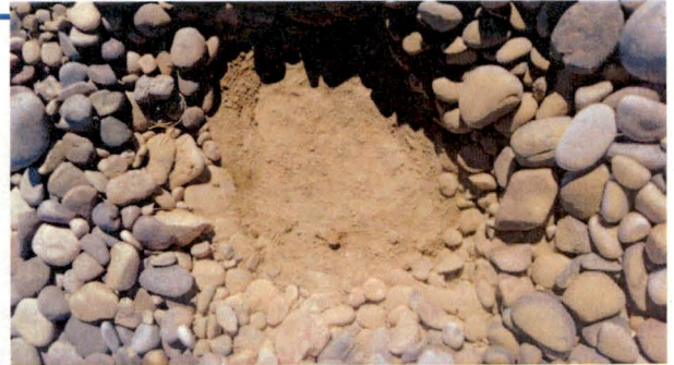
Photograph 14. Compacted Radon Barrier at Location 206B
