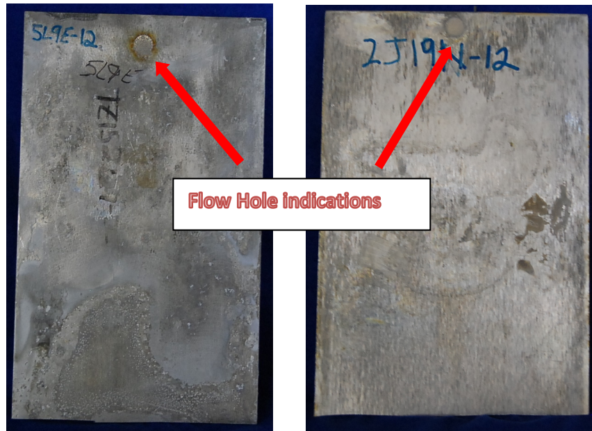
Figure 2 Example of Flow hole indication on Panels 2J19L and 5L19E
