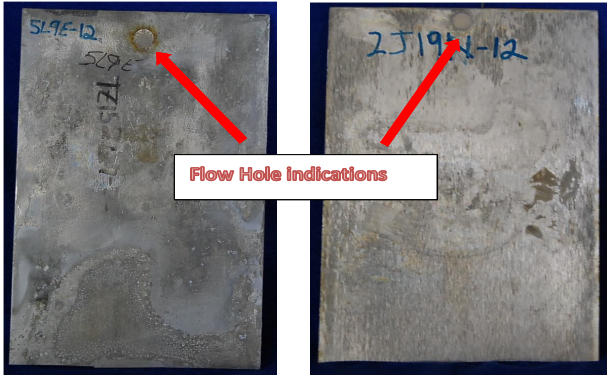
Figure 13. Example of Flow Hole Indications on Panels 2J19L and 5L19 E
