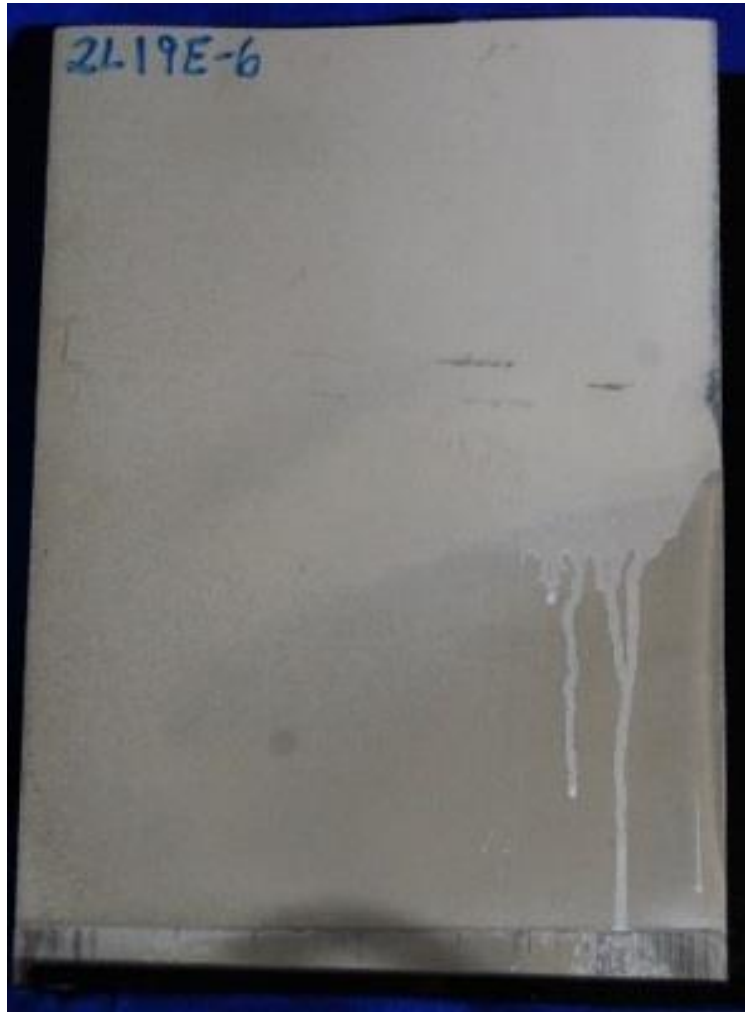
Figure 12. Front of Panel 2L19E-6, an example of a worst-case condition of encapsulation paint coverage
