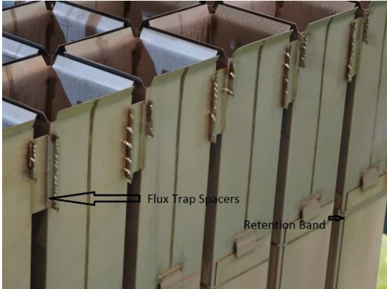
Figure 5. Module B (Region 1) section from Zion SFP during initial cutting of module for removal of Boral® panels at Alaron (photo courtesy of M. Harris, NETCO [1])
