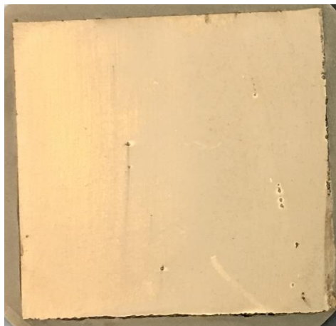
Figure 44 Picture of surface of specimen immersed in Solution 4 (BWR base) after 6 weeks before XRD analysis
