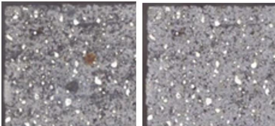
Figure 53. High Magnification Pictures of Sample 5L9S-4 (top left corner) before (left) and after (right) the 12 Days of Exposure
