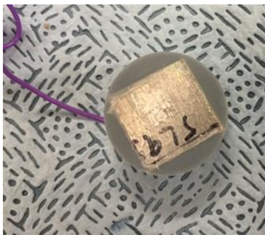
Figure 9. Picture of Region 2 sample connected with purple coated wire and mounted in acrylic
