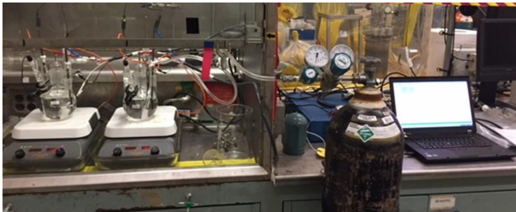
Figure 10. Two separate electrochemical tests in progress in the radiological hood. The cells are connected to a potentiostat and computer. Nitrogen gas was adapted for running ASTM G5 experiments.
