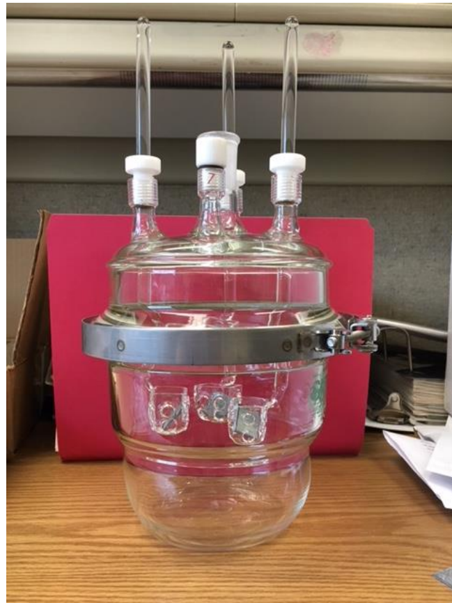
Figure 11. Setup for Immersion Test
