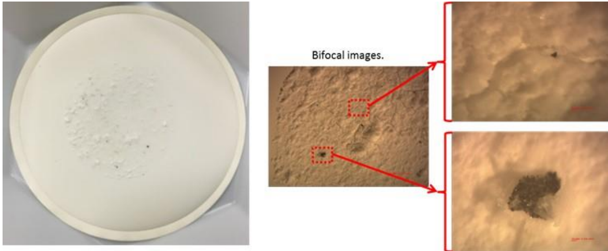
Figure 54. Filter cake resulting from filtration of the solution charge after 3 days exposure and agitation on the surface oxide of a declad Boral® coupon.
