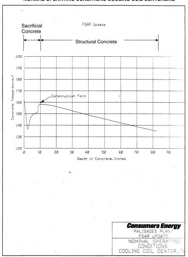
NORMAL OPERATING CONDITIONS COOLING COIL CENTERLINE
