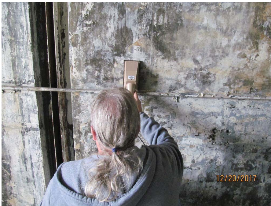
Photograph 11: Static measurement with LM43-93 probe.
