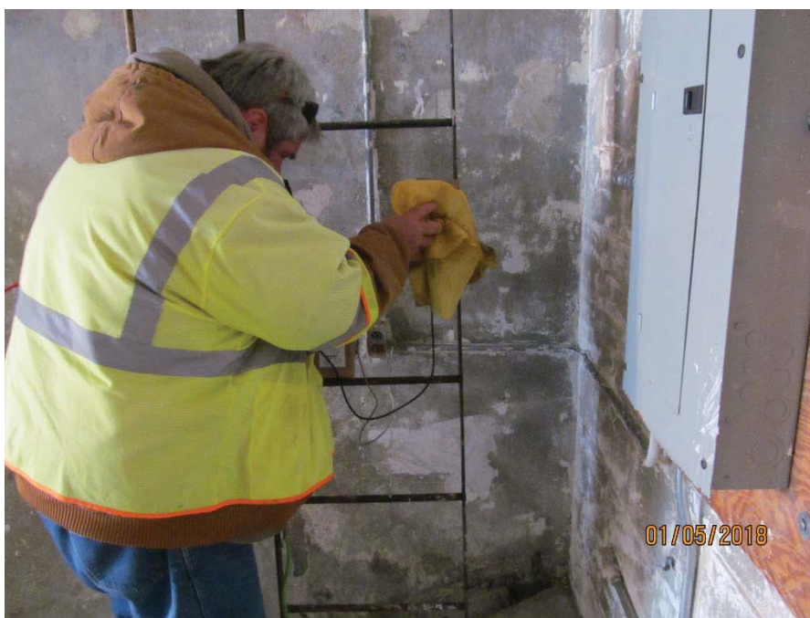
Photograph 20: Measurement of large area wipe (LAW) in Room 6A1.
