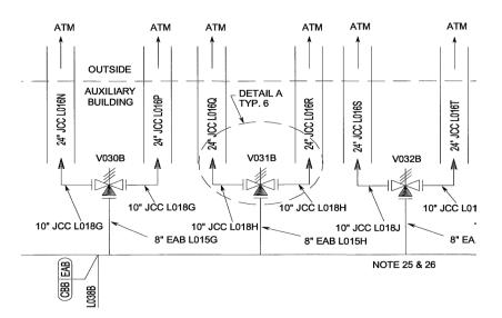
Figure 2.2.4-1 (Sheet 2 of 3) Steam Generator System
