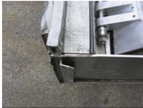
Figure 2-59 - Cracked bottom weld
