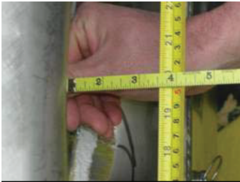
Figure 2-78 - CTU3 puncture depth measurement
