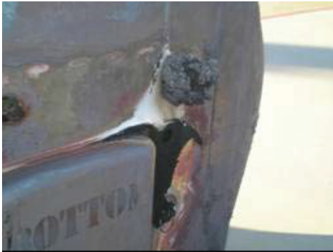
Figure 2-87 - Foam char in lock pin area Figure 2-88 - CTU3 lid removal
