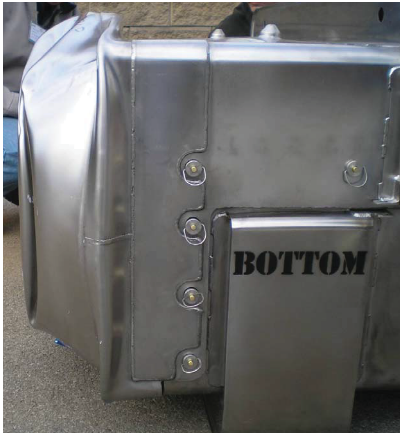
Figure 2-6 – Side View of Impact Limiter Damage
