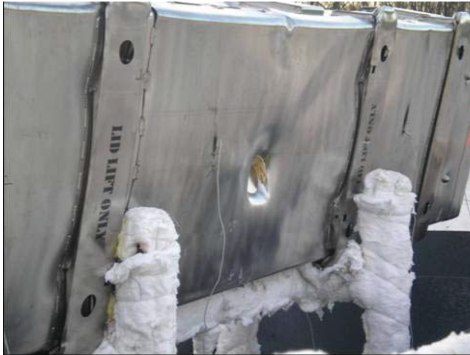
Figure 3-7 – Close-up of MAP CTU 3 on Test Stand Showing Puncture Bar Damage
