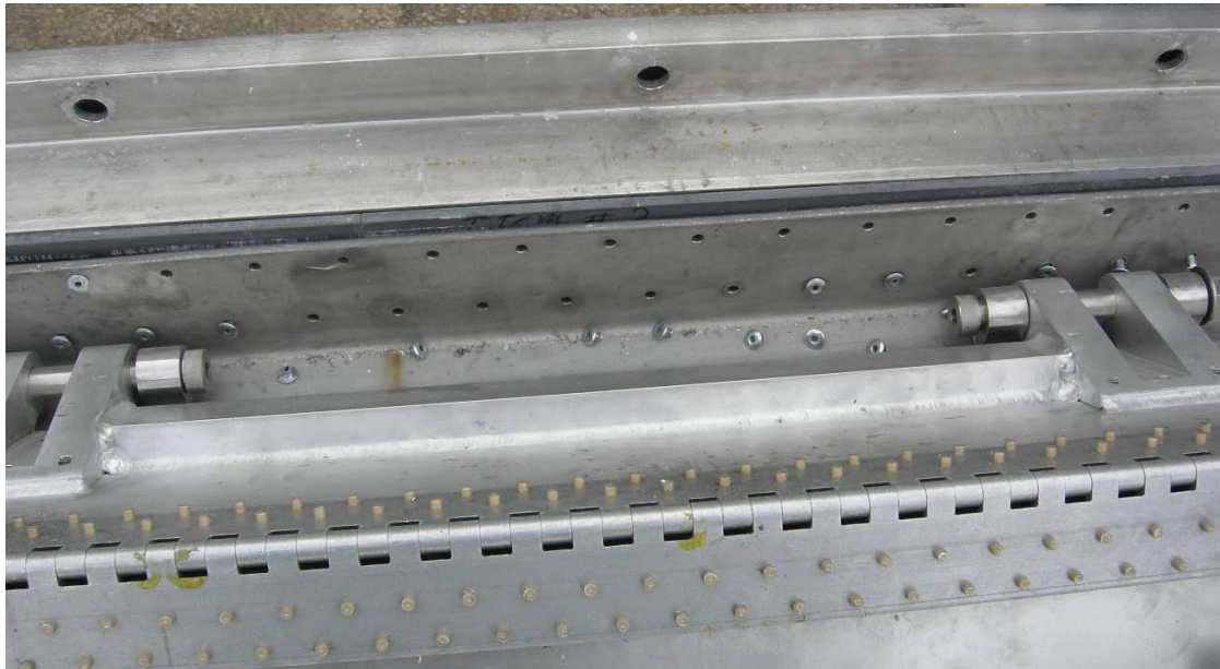
Figure 2-22 – Sheared Base Assembly Rivets
