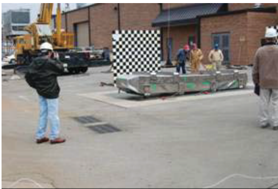
Figure 2-45 - CTU1 after impact
