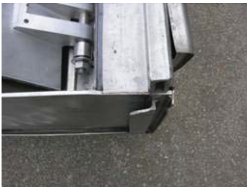
Figure 2-60 - No damage to bottom closure
