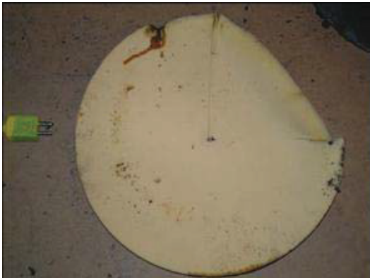
Figure 3-29 – Remaining 6 lb/ft 3 foam, backside fiber paper
