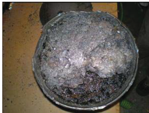
Figure 3-30 – Foam char under ceramic fiber paper
