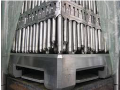
Figure 2-62 - Slight rod movement (bottom) Figure 2-63 - Bottom end fitting
