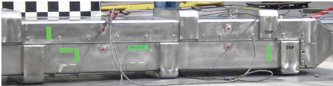
Figure 2-3 – Secondary Impact Stiffener Damage
