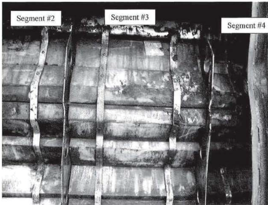
Figure 2-103 - Nylon 6,6 Segments #2, #3, and #4. Foam char is still visible on segment #3.
