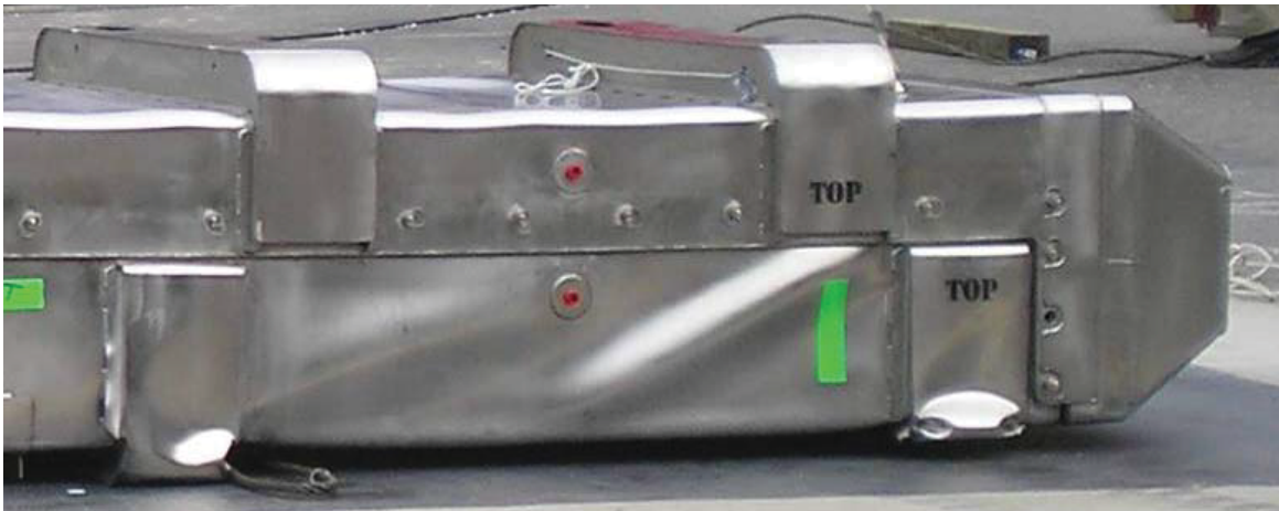
Figure 2-9 – Secondary Impact End Damage
