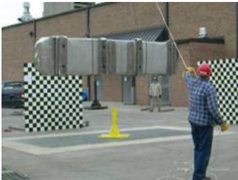
Figure 2-52 - CTU1 side puncture test
