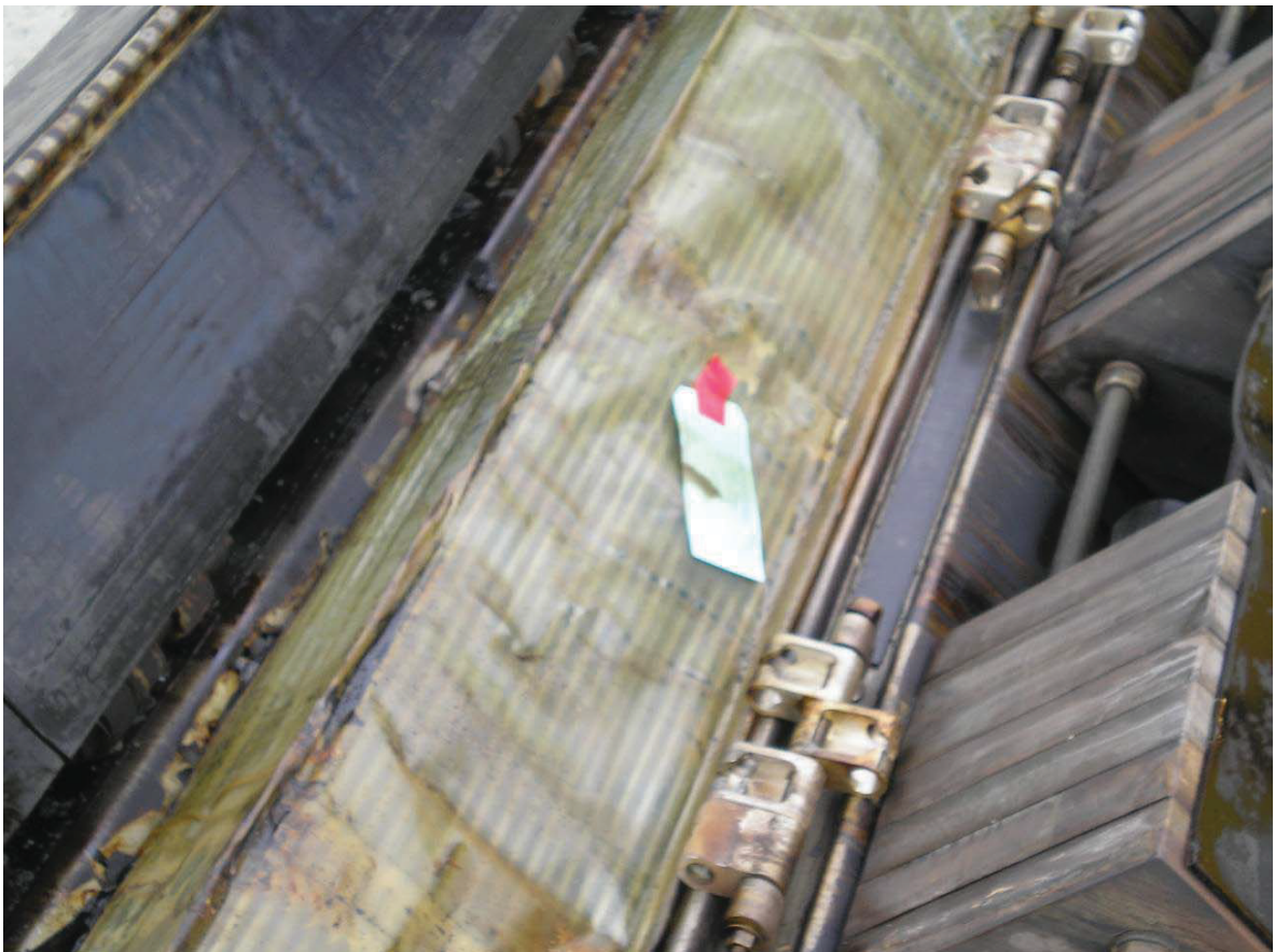
Figure 2-29 – Fuel Assembly with Bag and Tag Intact after Fire Test
