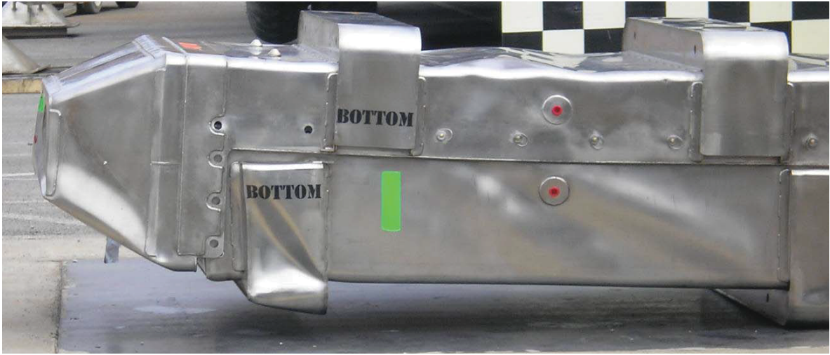
Figure 2-8 – Primary Impact End Damage
