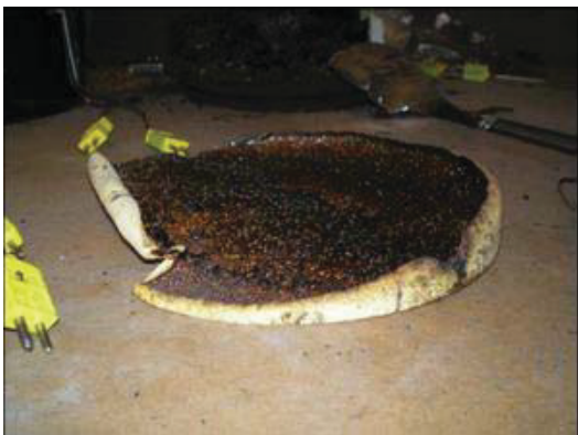
Figure 3-31 – Remaining 6 lb/ft 3 foam
