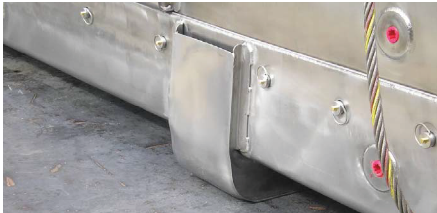
Figure 2-4 – Typical Stiffener after Drop
