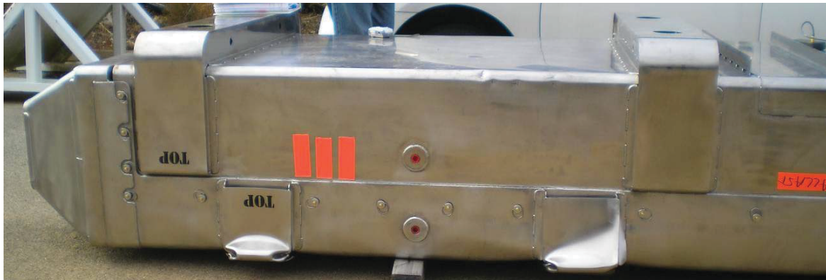
Figure 2-10 – Global Package Damage after Test CD5
