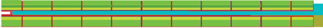
Figure 6-22 – View of the side of the package (y-z plane) where assemblies have been shifted axially where 15 cm (5.906 inches) of the assemblies are outside of the flux trap region
