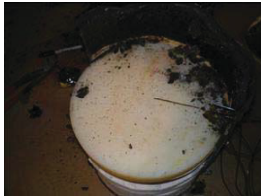
Figure 3-32 – Moderator surface, flame side
