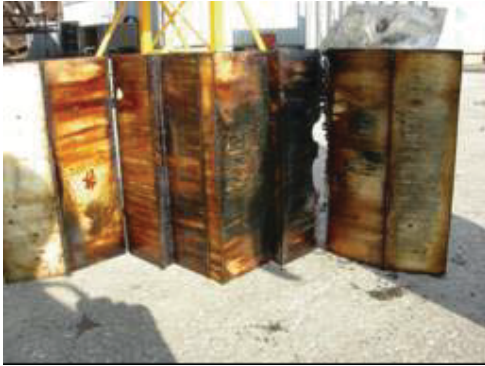
Figure 2-107 - Segment #5 after cleaning
