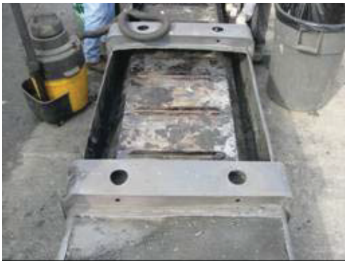
Figure 2-110 - Base liner with foam char removed
