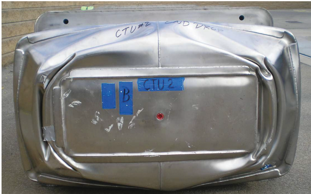
Figure 2-5 – Front View of Impact Limiter Damage
