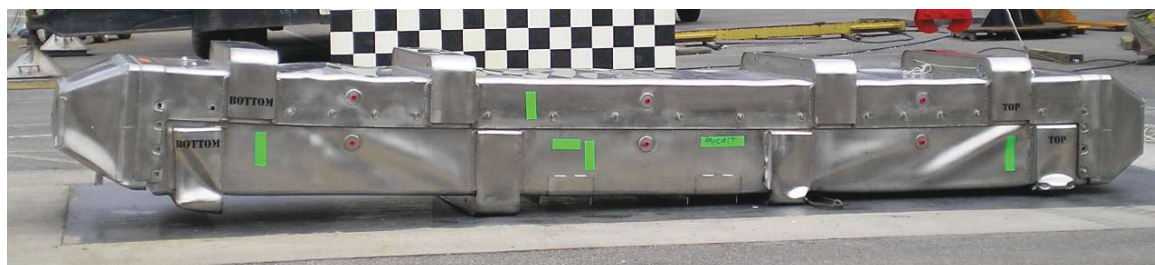
Figure 2-7 – Global Package Damage after Test CD3
