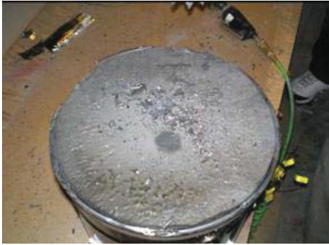
Figure 3-27 – Intact ceramic fiber following test bucket
