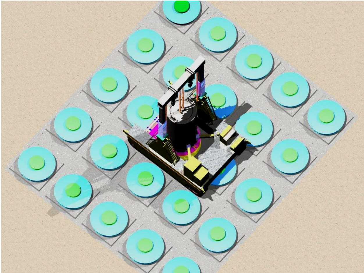
Figure 3.I.4; Cask Transporter on the ISFSI Positioned to Transfer MPC in the Central Cavity in the 5x5 VVM Array (illustrative analysis case)
