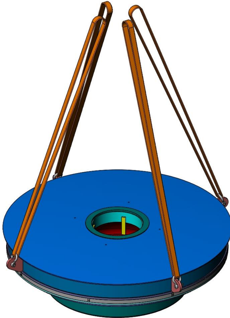
FIGURE 8.I.3: EXAMPLE RIGGING CONFIGURATION FOR THE HI-STORM 100U* VVM LID
