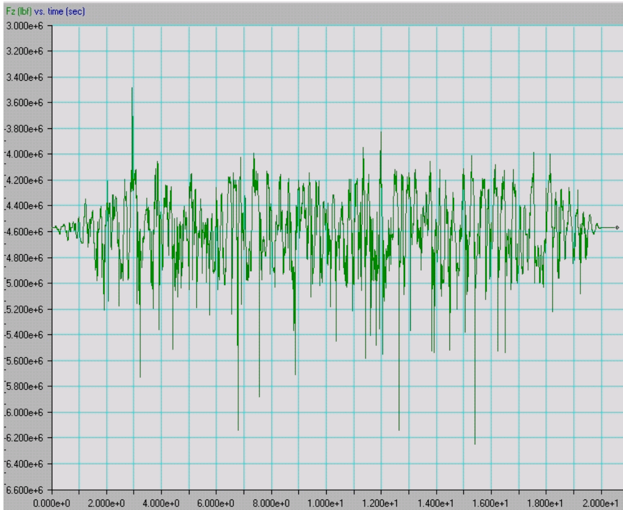
FIGURE 3.4.44: VARIATION OF FOUNDATION RESISTANCE FORCE VS. TIME FOR REG. GUIDE 1.60 SEISMIC INPUT
