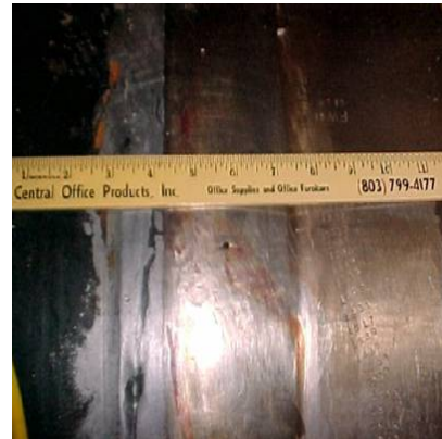
V.C. Sumner (Fall 2000): Leaking PWR CRDM Head Crack in a hot leg nozzle to Penetrations pipe weld
