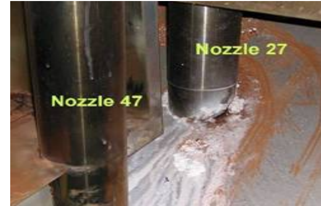
V.C. Sumner (Fall 2000): Leaking PWR CRDM Head Crack in a hot leg nozzle to Penetrations pipe weld
