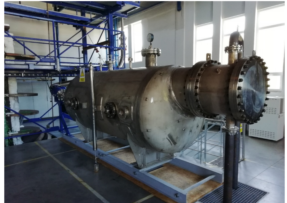
View of the condenser and upper part of the cooling channel
