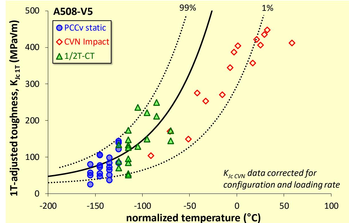
Correction for difference in geometry and test conditions.
