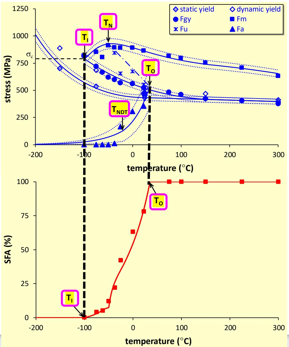
$T_I$  : brittle fracture temperature (SFA=0%)
