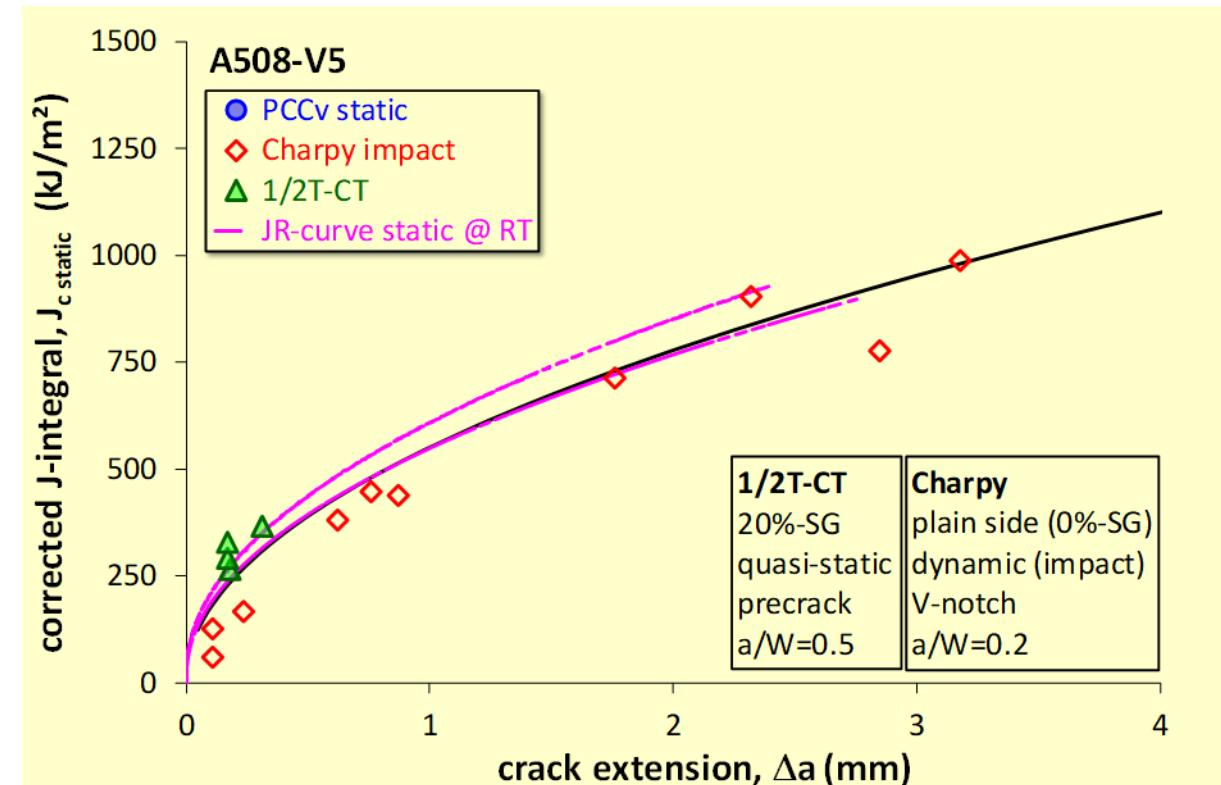
Correction of  $J_R^{\text{CVN impact}}$  to obtain  $J_R^{\text{static}}$  accounting for effects of geometry and loading conditions
