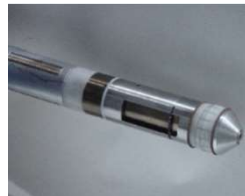
Step 1 Cutting and Removal of Thermal Sleeve
