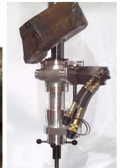
Step 3 Adapter boring, weld Prep Machining and manual PT
