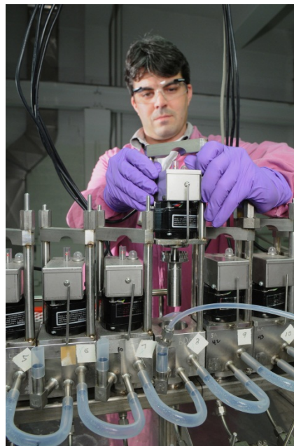
Researcher preparing new centrifugal contactor bank for use in aqueous separations process evaluation
