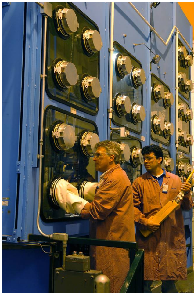
Engineering-scale electrorefining facility for demonstrating electrochemical separations
