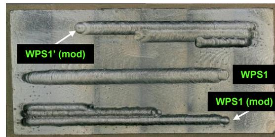
Welds performed at WEC on irradiated sample 3E3A (~8 appm He)
