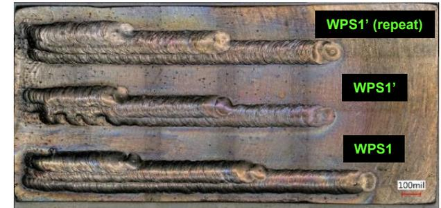
Welds performed at WEC on front side of irradiated sample 5D2 (0.2 appm He)
