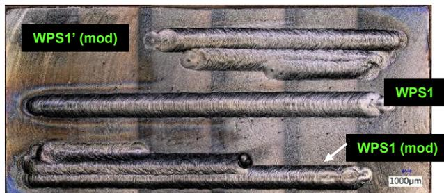
Welds performed at WEC on irradiated sample 3A2A (~3 appm He)
