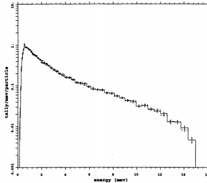
Fig. 2: bremsstrahlung X-ray energy spectrum in lead target for a beta from Y-90.
