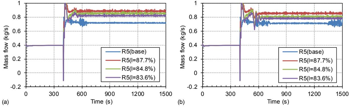
**Figure 35 Mass Flowrate Dependence on Initial Primary Coolant System Inventory for S-NC-3 Test Cases: (a) C14\_S-67.4% and (b) C15\_S-55.5%**
