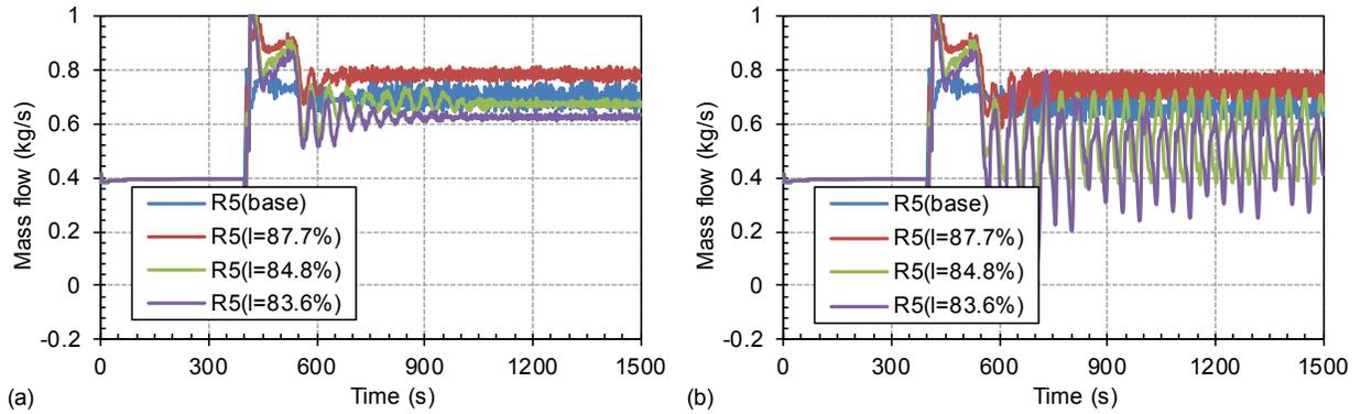
**Figure 36 Mass Flowrate Dependence on Initial Primary Coolant System Inventory for S-NC-3 Test Cases: (a) C16\_S-43.6% and (b) C17\_S-33.2%**
