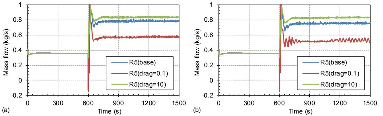
**Figure 24 Mass Flowrate Dependence on Dial Value Drag Coefficient Variation for S-NC-2 Test Cases: (a) C9\_P-84.8% and (b) C10\_P-83.6%**
