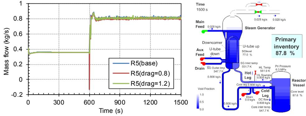
Figure 10 Mass Flowrate Dependence on 20% Drag Coefficient Variation for S-NC-2 Test Case C8\_P-87.8% (left) and Liquid Distribution at 1500 S for Base Case (right)
