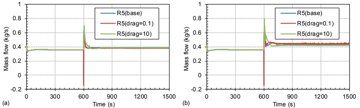
**Figure 21 Mass Flowrate Dependence on Dial Value Drag Coefficient Variation for S-NC-2 Test Cases: (a) C3\_P-96.3% and (b) C4\_P-95.2%**
