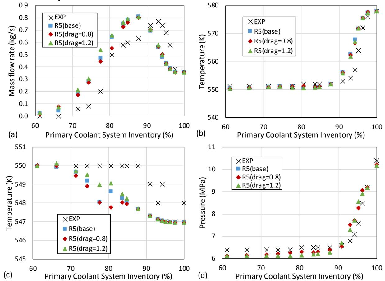
**Figure 2 Comparison between RELAP5 Sensitivity Calculations Varying Drag Coefficient (0.8 to 1.2) and Experiment for S-NC-2 Test as a Function of Primary Coolant System Inventory: (a) Primary System Mass Flowrate, (b) Hot Leg Fluid Temperature, (c) SG Outlet Temperature, (d) Primary Pressure**
