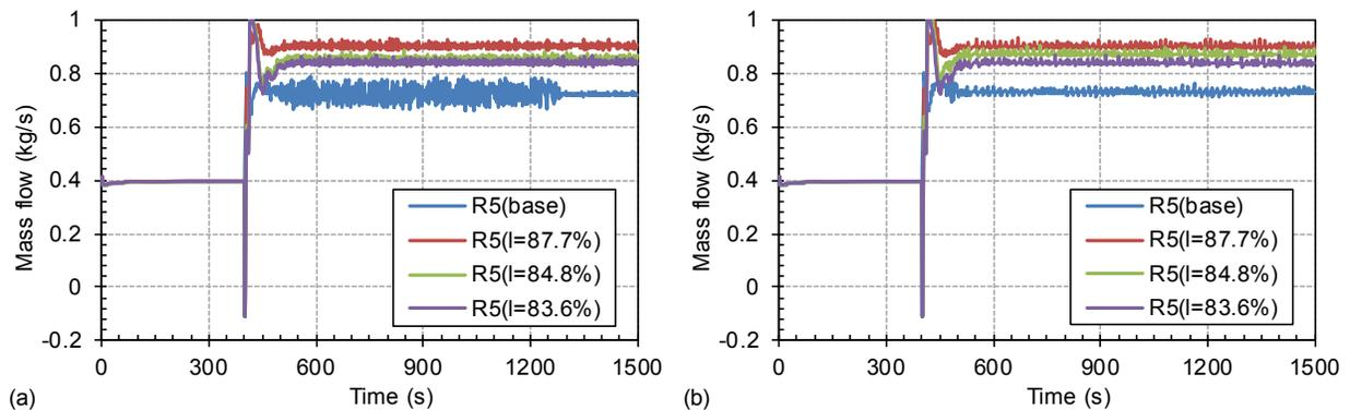
**Figure 33 Mass Flowrate Dependence on Initial Primary Coolant System Inventory for S-NC-3 Test Cases: (a) C10\_S-100.0% and (b) C11\_S99.1%**
