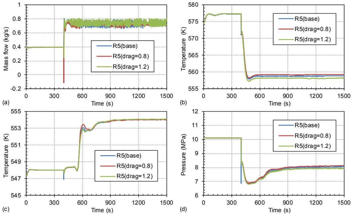
**Figure 31 Sensitivity Calculations Varying Drag Coefficient for S-NC-3 Test Case C19\_S-15.2%: (a) Primary System Mass Flowrate, (b) Hot Leg Fluid Temperature, (c) SG Outlet Temperature, (d) Primary Pressure**
