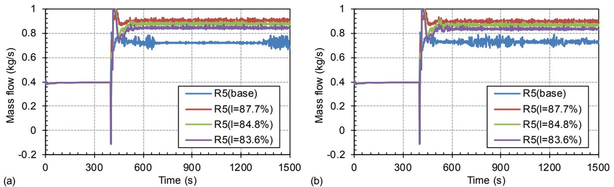
**Figure 34 Mass Flowrate Dependence on Initial Primary Coolant System Inventory for S-NC-3 Test Cases: (a) Cases C12\_S-86.9% and (b) C13\_S-75.5%**
