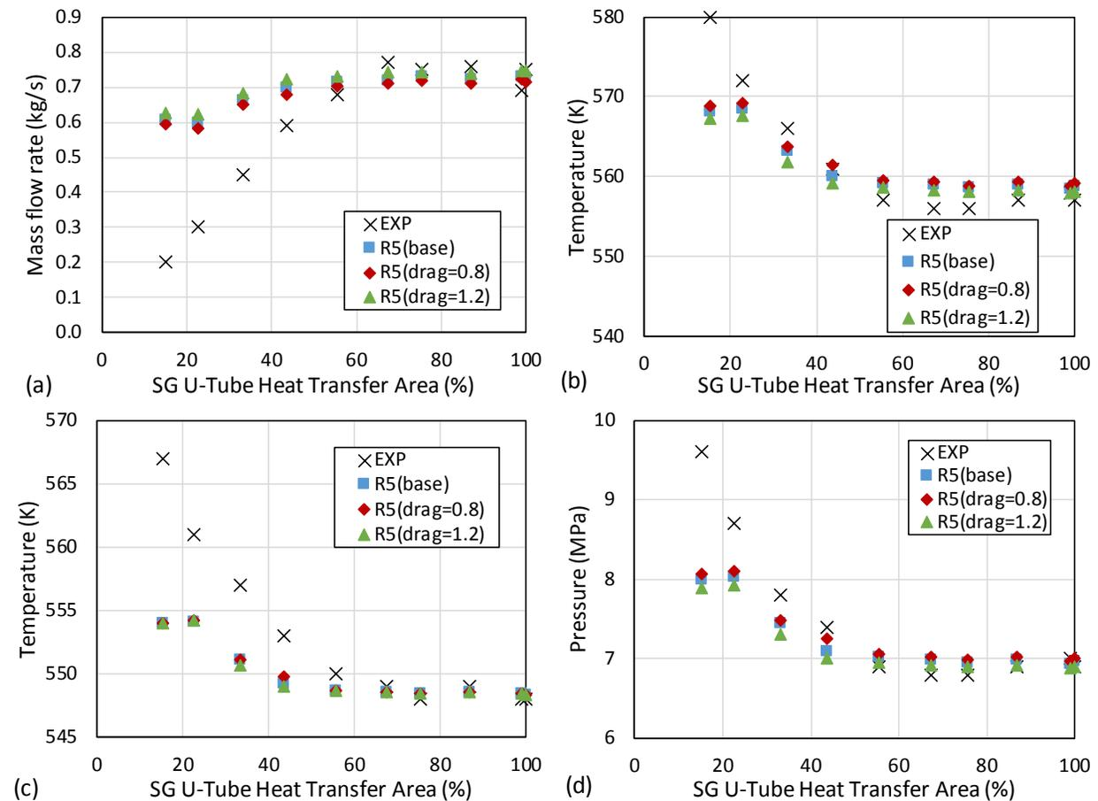
**Figure 32 Comparison Between RELAP5 Sensitivity Calculations Varying Drag Coefficient and Experiment for S-NC-3 Test as a Function of SG U-Tube Heat Transfer Area: (a) Primary System Mass Flowrate, (b) Hot Leg Fluid Temperature, (c) SG Outlet Temperature, (d) Primary Pressure**
