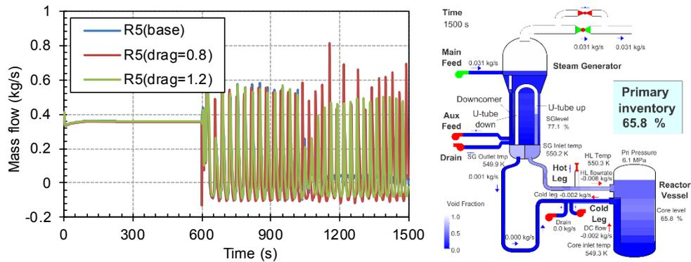
Figure 17 Mass Flowrate Dependence on 20% Drag Coefficient Variation for S-NC-2 Test Case C15\_P-66.3% (left) and Liquid Distribution at 1500 S for Base Case (right)
