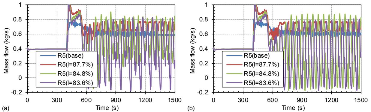
**Figure 37 Mass Flowrate Dependence on Initial Primary Coolant System Inventory for S-NC-3 Test Cases: (a) C18\_S-22.7% and (b) C19\_S-15.2%**
