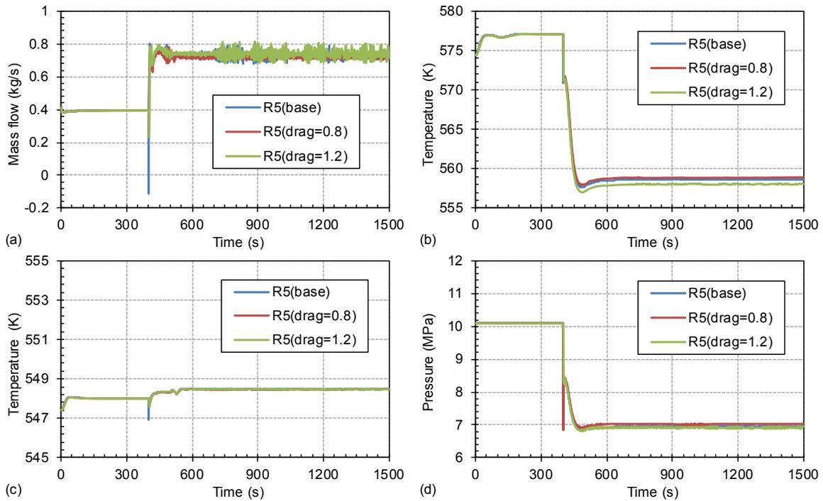
**Figure 29 Sensitivity Calculations Varying Drag Coefficient for S-NC-3 Test Case C13\_S-75.5%: (a) Primary System Mass Flowrate, (b) Hot Leg Fluid Temperature, (c) SG Outlet Temperature, (d) Primary Pressure**
