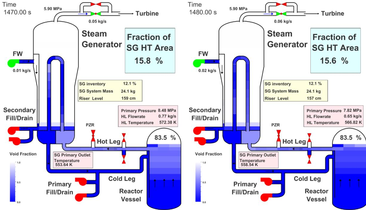
Figure 41 Animation Mask for S-NC-03 Calculated Case C19\_S-15.2% with Primary Side Filled as in S-NC-02\_P-83.6% at 1470 s (left) and 1480 s
