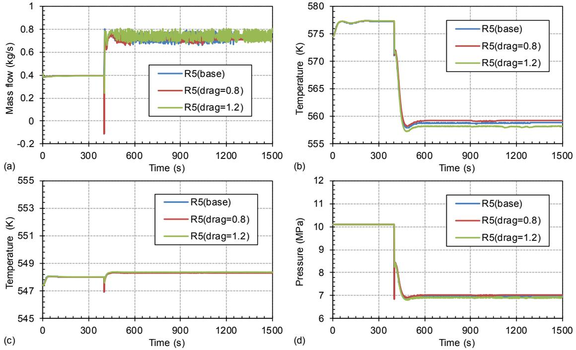
**Figure 28 Sensitivity Calculations Varying Drag Coefficient for S-NC-3 Test Case C10\_S-100.0%: (a) Primary System Mass Flowrate, (b) Hot Leg Fluid Temperature, (c) SG Outlet Temperature, (d) Primary Pressure**
