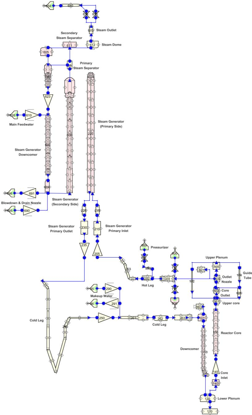
**Figure 1 RELAP5 Input Model of Semiscale Mod-2A Single Loop Represented by SNAP**
