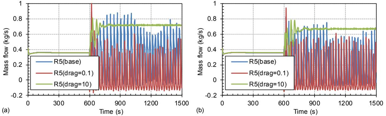
**Figure 26 Mass Flowrate Dependence on Dial Value Drag Coefficient Variation for S-NC-2 Test Cases: (a) C13\_P-74.4% and (b) C14\_P-71.4%**
