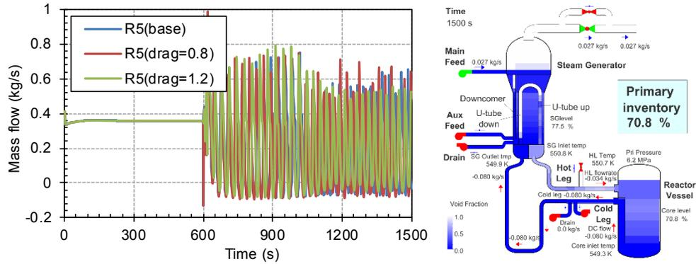
Figure 16 Mass Flowrate Dependence on 20% Drag Coefficient Variation for S-NC-2 Test Case C14\_P-71.4% (left) and Liquid Distribution at 1500 S for Base Case (right)
