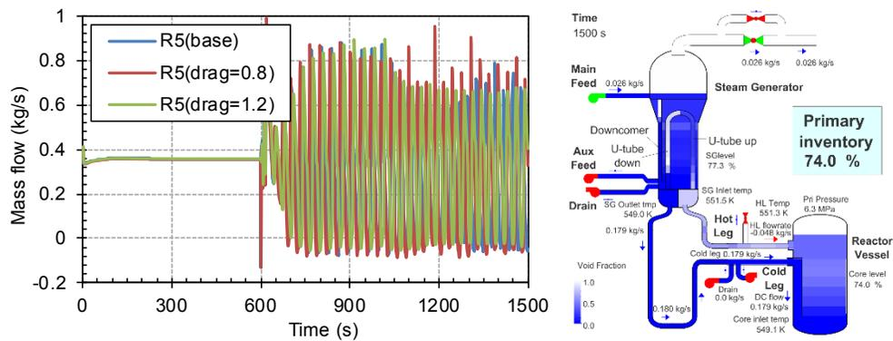
Figure 15 Mass Flowrate Dependence on 20% Drag Coefficient Variation for S-NC-2 Test Case C13\_P-74.4% (left) and Liquid Distribution at 1500 S for Base Case (right)
