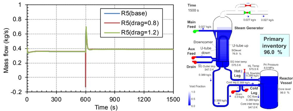
Figure 5 Mass Flowrate Dependence on 20% Drag Coefficient Variation for S-NC-2 Test Case C3\_P-96.3% (left) and Liquid Distribution at 1500 S for Base Case (right)
