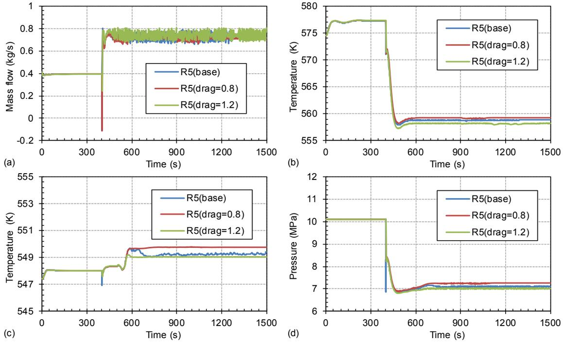
**Figure 30 Sensitivity Calculations Varying Drag Coefficient for S-NC-3 Test Case C16\_S-43.6%: (a) Primary System Mass Flowrate, (b) Hot Leg Fluid Temperature, (c) SG Outlet Temperature, (d) Primary Pressure**
