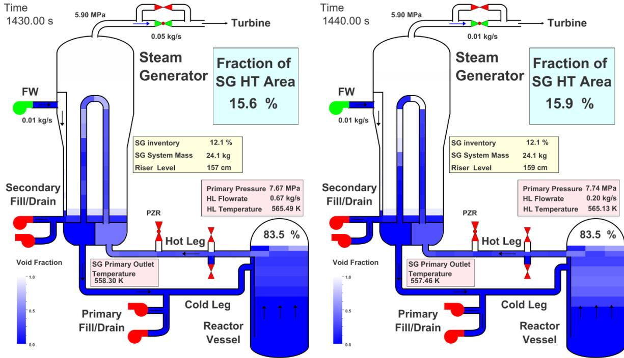
Figure 39 Animation Mask for S-NC-03 Calculated Case C19\_S-15.2% with Primary Side Filled as in S-NC-02\_P-83.6% at 1430 s (left) and 1440 s
