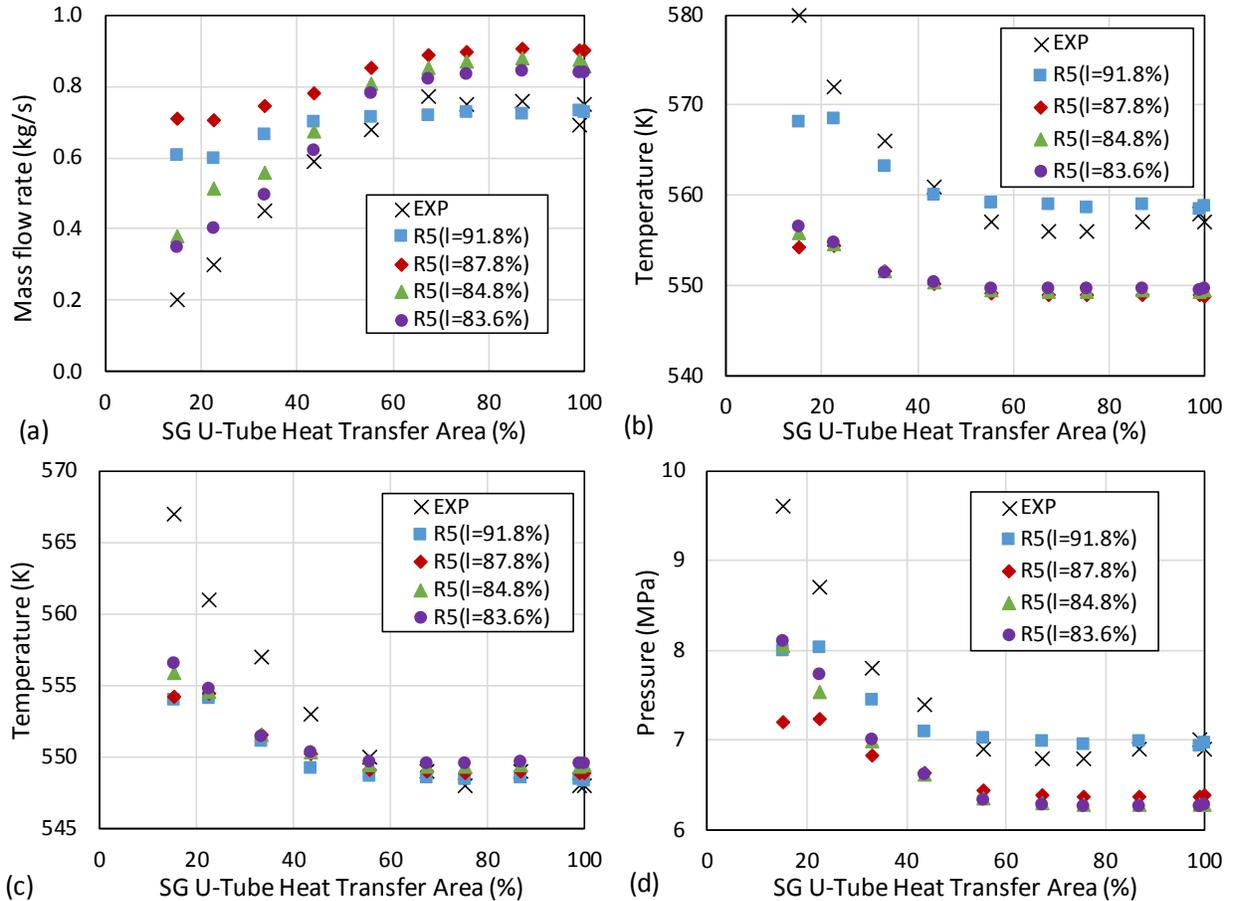
**Figure 38 Comparison Between RELAP5 Sensitivity Calculations Varying Primary Coolant System Inventory and Experiment for S-NC-3 Test as a Function of SG U-Tube Heat Transfer Area: (a) Primary System Mass Flowrate, (b) Hot Leg Fluid Temperature, (c) SG Outlet Temperature, (d) Primary Pressure**
