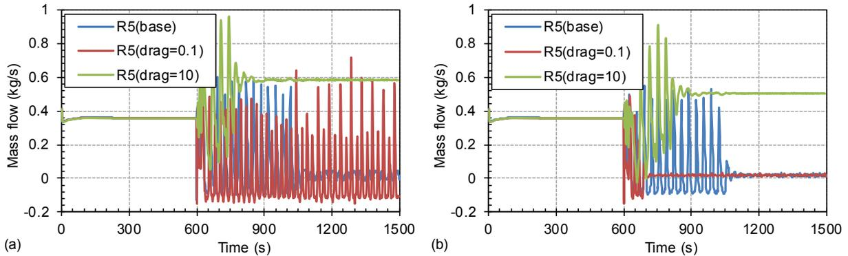
**Figure 27 Mass Flowrate Dependence on Dial Value Drag Coefficient Variation for S-NC-2 Test Cases: (a) C15\_P-66.3% and (b) C16\_P-61.2%**
