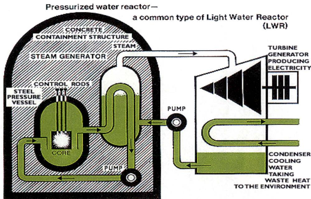
Figure 1.4-1: SIMPLIFIED DIAGRAM OF A PRESSURIZED WATER REACTOR
