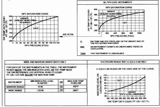
Which of the RPV level indicator(s) listed below is (are) available to trend RPV level per the TRIPs?
