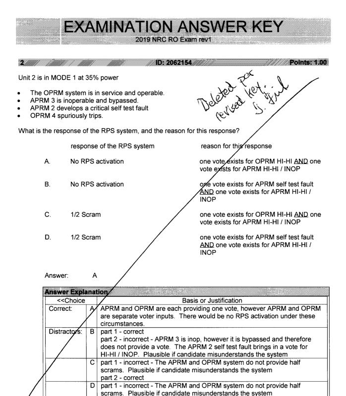
part 2 - incorrect - APRM 3 is inop, however it is bypassed and therefore does not provide a vote. The APRM 2 self test fault brings in a vote for HI-HI / INOP. Plausible if candidate misunderstands the system
