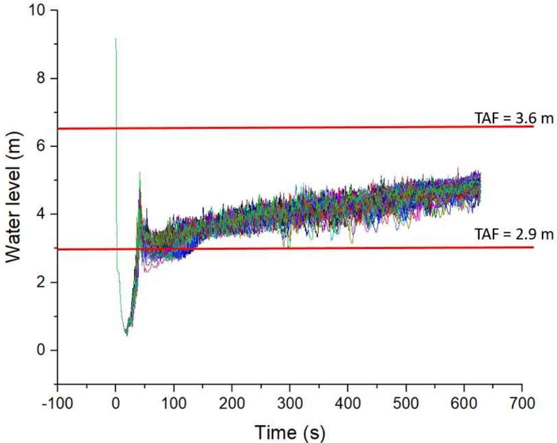
**Figure 28** Core Collapsed Water Level of 59 Cases
