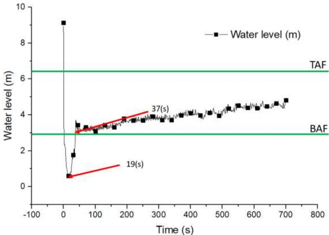
Figure 25 Core Collapsed Water Level
