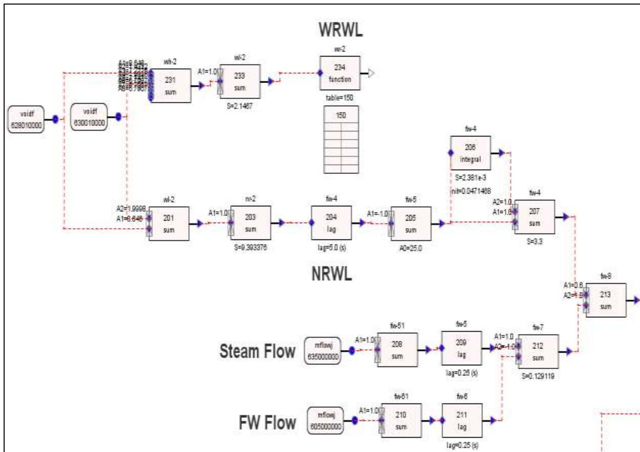
**Figure 7 Feedwater Control System in SNAP Interface**
