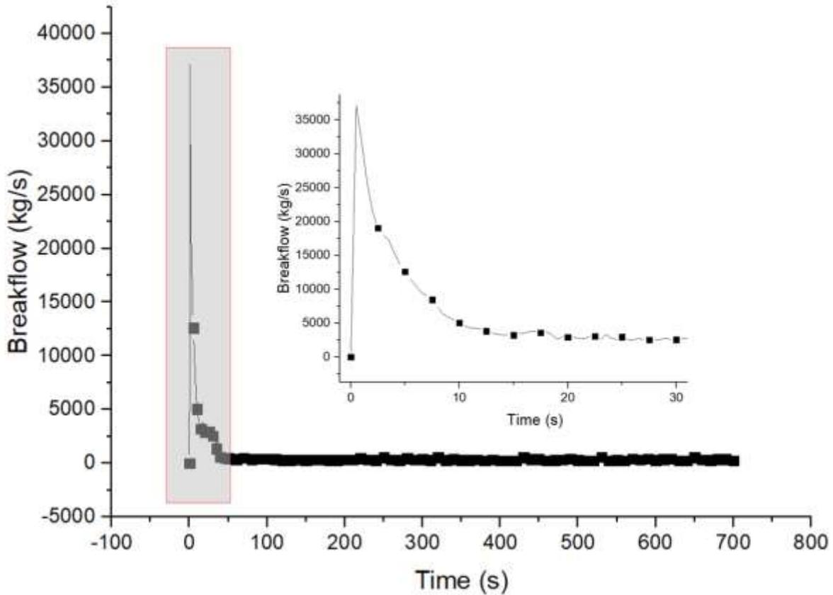
**Figure 21 LBLOCA Break Flow Rate**
