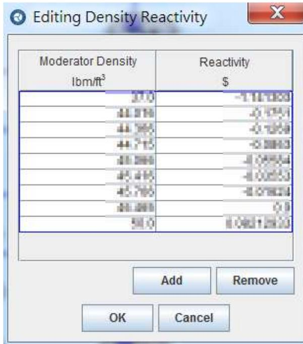
Figure 16 Density Effect Reactivity Feedback Table
