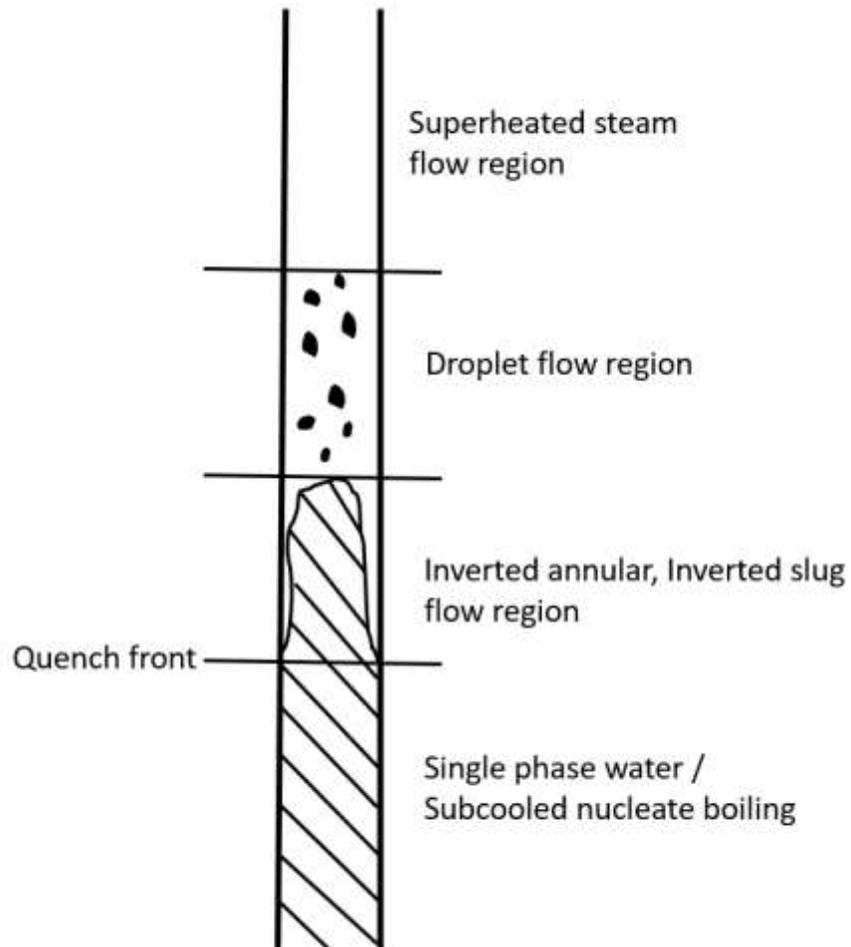
**Figure 26 Core Flow Regime during Reflooding phase**
