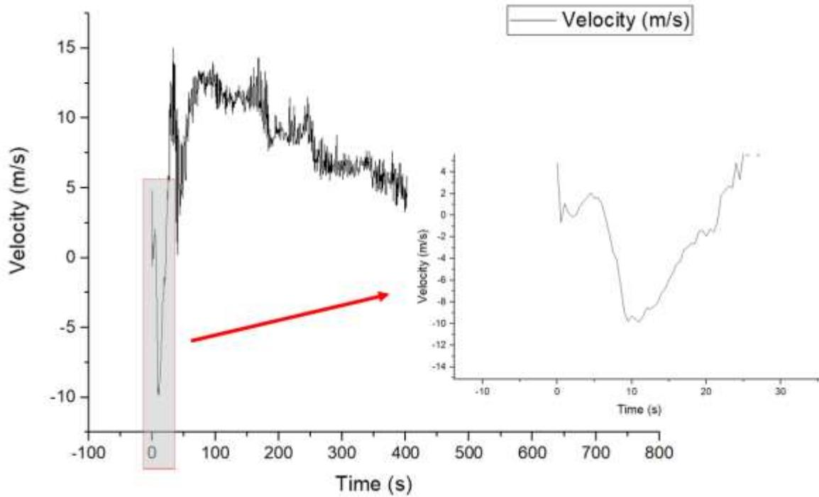
Figure 24 Core Vapor Velocity
