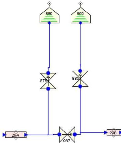
**Figure 20 RELAP5/SNAP LBLOCA Break Model**
