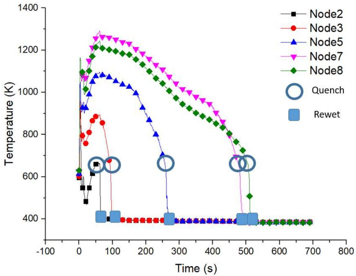
Figure 27 Cladding Temperature Axial Profile
