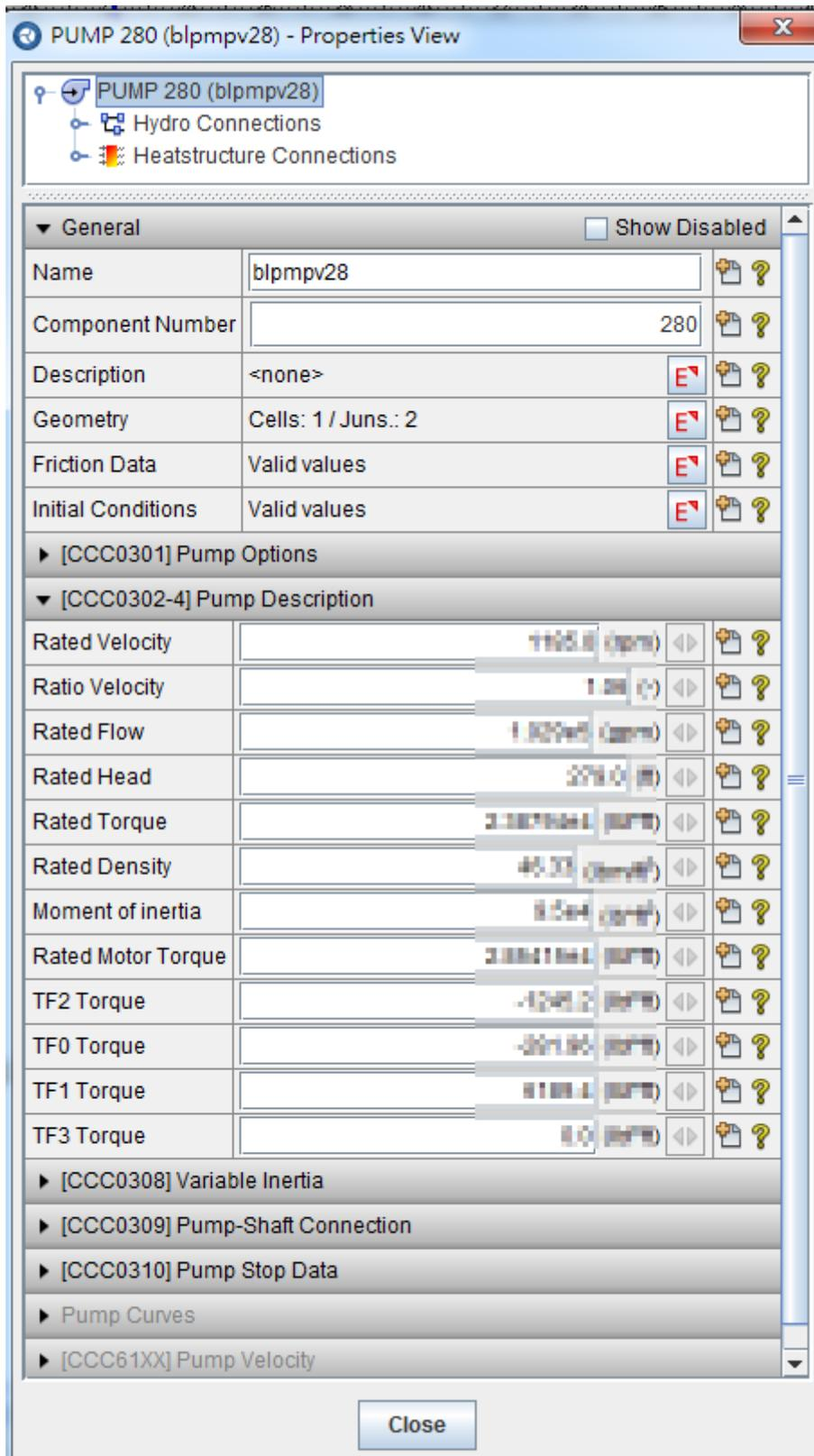
Figure 3 RCP Properties of Maanshan NPP in SNAP Interface
