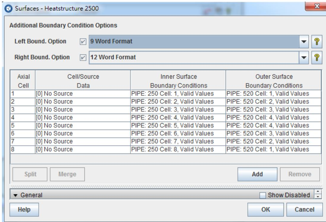
Figure 5 Heat Structure 2500 Properties in SNAP Interface
