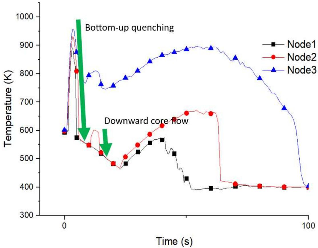
Figure 23 Cladding Temperature at the Lower Part
