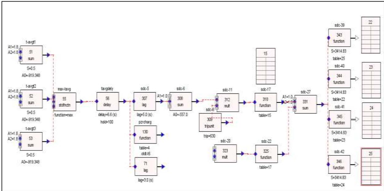
**Figure 8 Steam Dump Control System in SNAP Interface**
