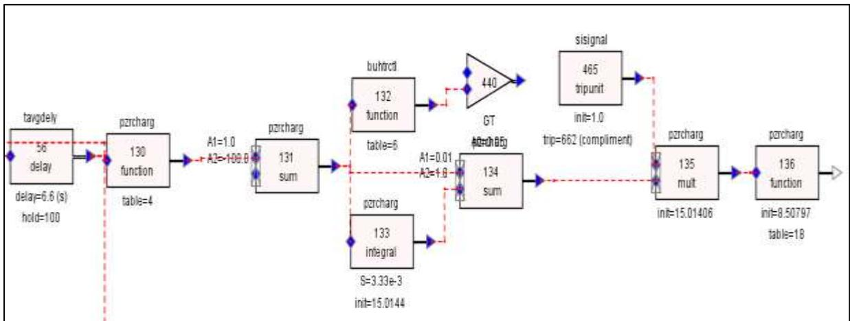
Figure 10 Pressurizer Injection Control System in SNAP Interface
