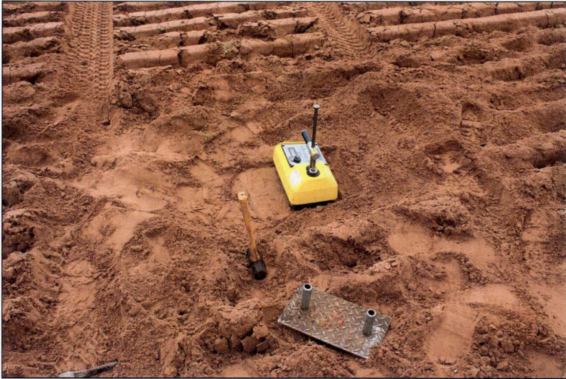
Photo 33. Moisture Density Test in Progress March 2018
