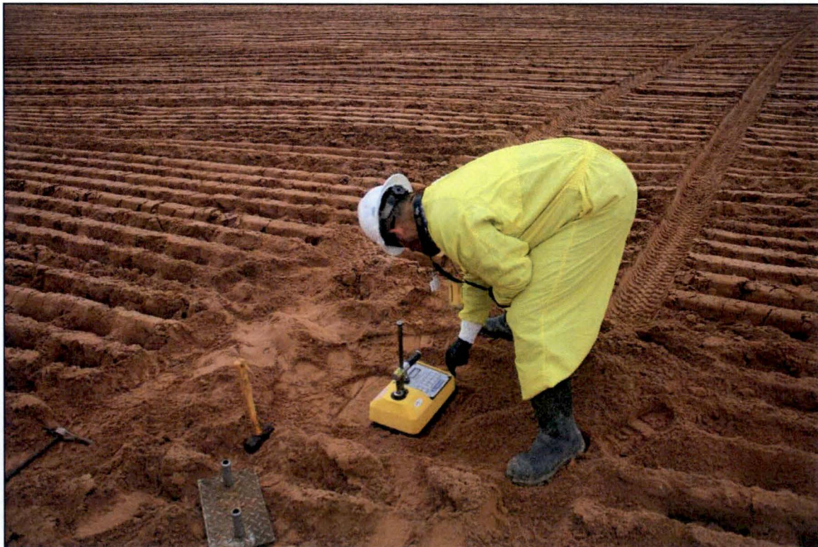
Photo 32. Moisture Density Test Start March 2018
