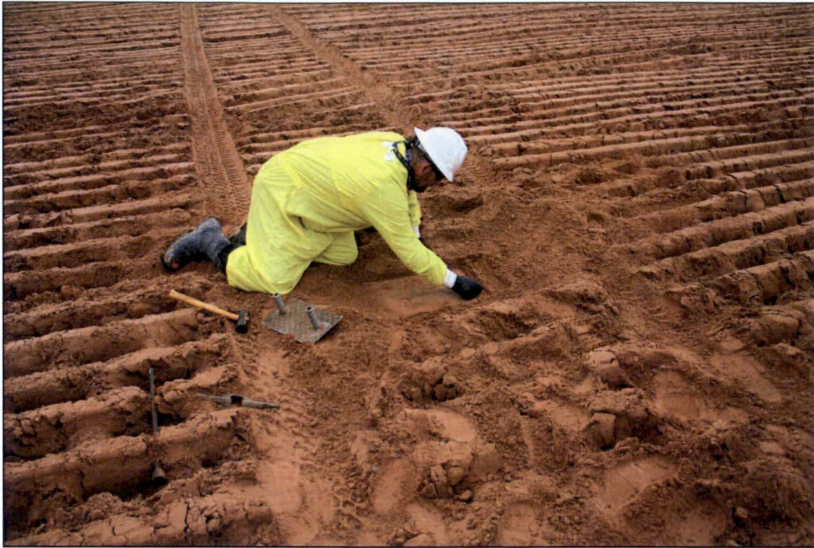
Photo 31. Moisture Density Site Preparation March 2018
