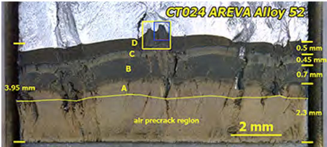
Figure 3-69 Optical Image of the Crack Growth Surface of the AREVA Alloy 52 Specimen (CT024)
