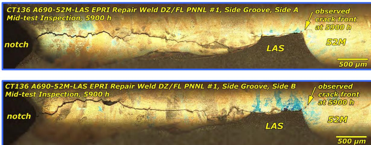
**Figure 5-113 Optical Images Showing Cracking in CT136 Side Grooves After a Test Time of 5900 Hours. Crack Front Has Reached the LOF Defects (black arrows) at the LAS Interface on Both Sides and Small Cracks Appear to Extend to the End of the LAS Plateau**
