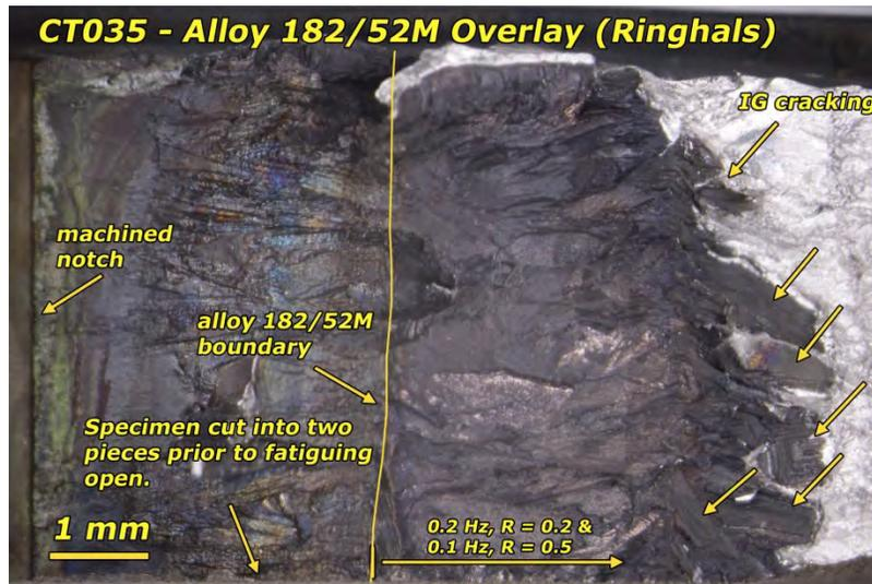
**Figure 4-18 Optical Micrograph of the Crack Growth Surface of CT035**
