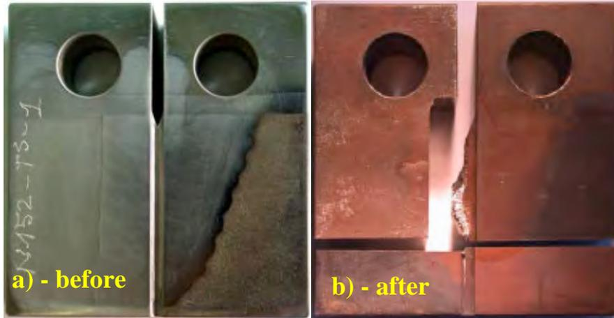
**Figure 3-61 1T CT Specimen That ANL Used for Their Test (N152-TS-1) on the ANL 152v2 Weldment**
