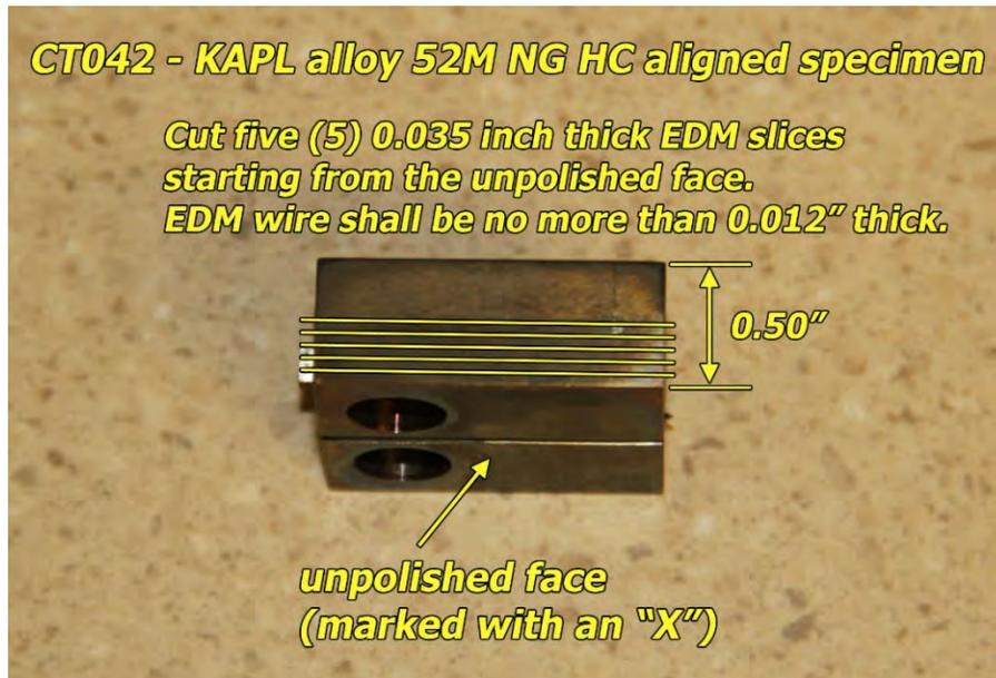
**Figure 3-113 Post-Test Serial Sectioning Plan for KAPL Alloy 52M NG Weld Specimens with Weld Cracks (CT042 and CT043)**
