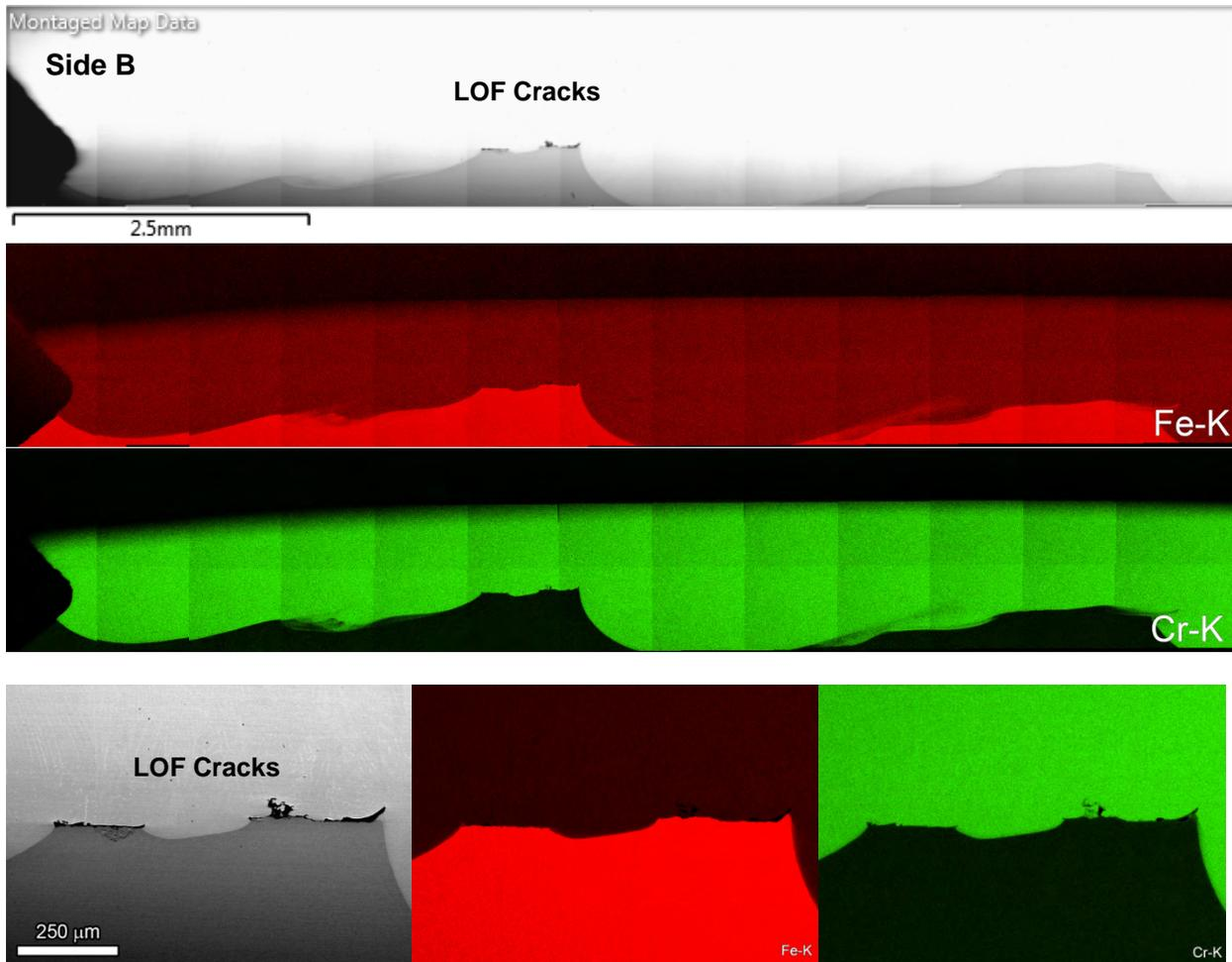
**Figure 5-22 SEM-BSE Images and EDS Elemental Maps Showing the 52M/LAS Interface Ahead of the Notch in the Side B Side Groove for the CT136 Specimen. Bottom Images Highlight the Local LOF Cracks**
