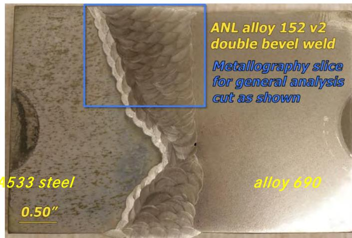
**Figure 3-29 Optical Macro Image of a Weld Slice Taken from the ANL Alloy 152v2 Weldment. Note That the Weld Orientation Is Flipped from Drawing in Figure 3-28**
