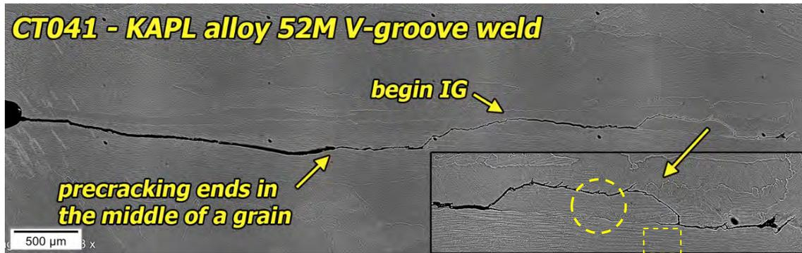
**Figure 3-99 Crack Profile of the KAPL Alloy 52M V-Groove Specimen CT041**
