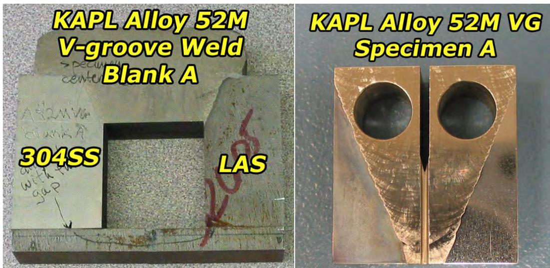
Figure 3-87 Photos of KAPL Alloy 52M V-Groove Weld Blank “A” and CT041 Specimen Machined from the Blank
