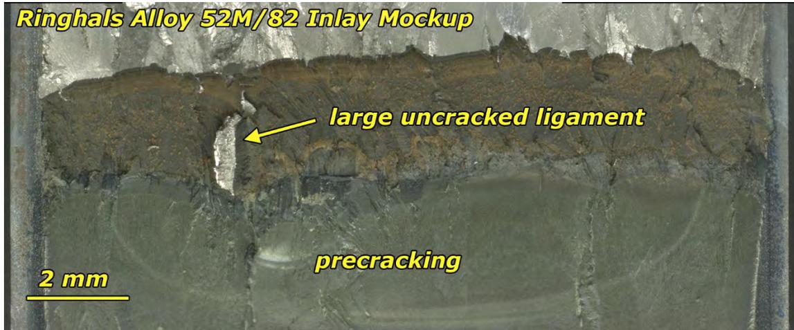
Figure 4-38 Crack Growth Surface of Ringhals Alloy 52M/82 Specimen CT030
