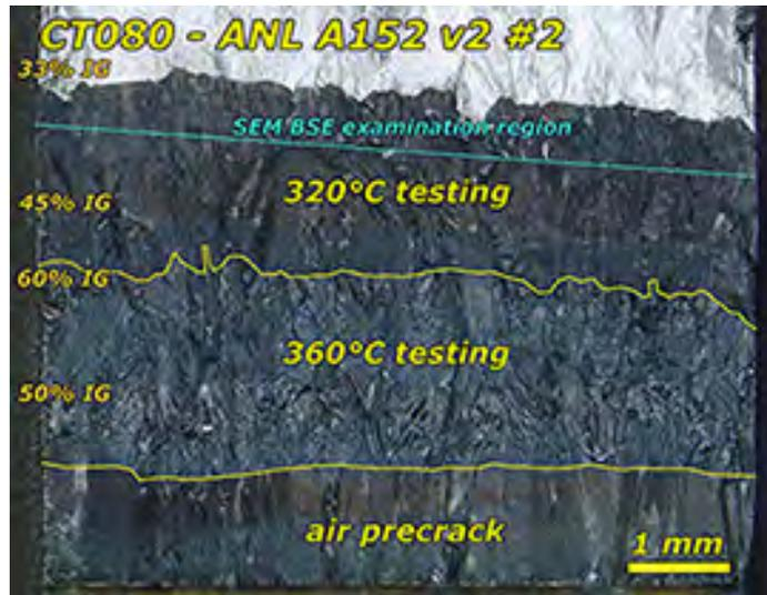
Figure 3-53 Optical Image of the 8-mm-Wide Section of the Crack-Growth Surface of the Second Alloy 152 V2 Specimen (CT080) Tested in 360°C and 320°C Simulated PWR Primary Water
