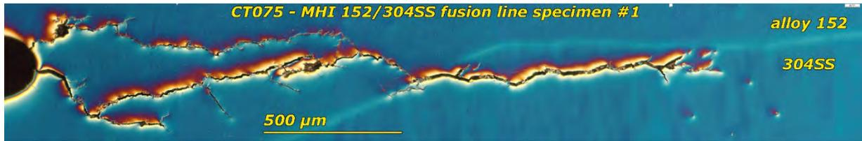
**Figure 5-27** Optical Image of the Interior Crack Profile of the Alloy 152/304SS Specimen #1 (CT075)
