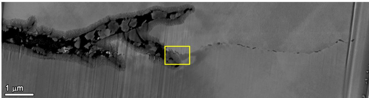
**Figure 4-24 SEM-BSE Images of the Leading IGSCC Crack Tip in the Alloy 52M Pass of Altered Composition**
