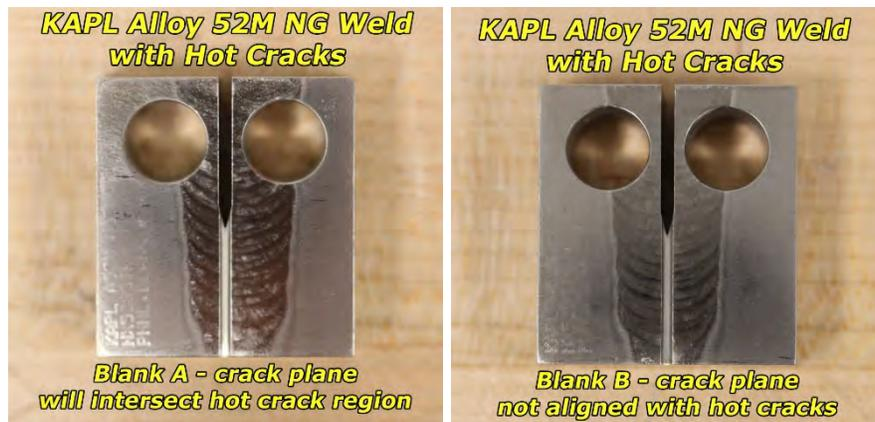
Figure 3-89 Photos of Specimens Cut from KAPL Alloy 52M Narrow Gap Weld Containing Hot Cracks. Blank a (CT042) Is Positioned Off-Center and near the Bottom of the Weldment to Insect a High Density of Weld Cracks, While Blank B (CT043) Is Positioned near the Center of the Weld Where No Weld Cracks Were Observed
