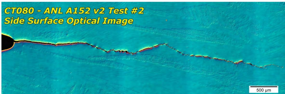
Figure 3-55 Optical Image of the Side-Surface Cross Section Taken from the Second Alloy 152 V2 Specimen (CT080) After SCC Testing
