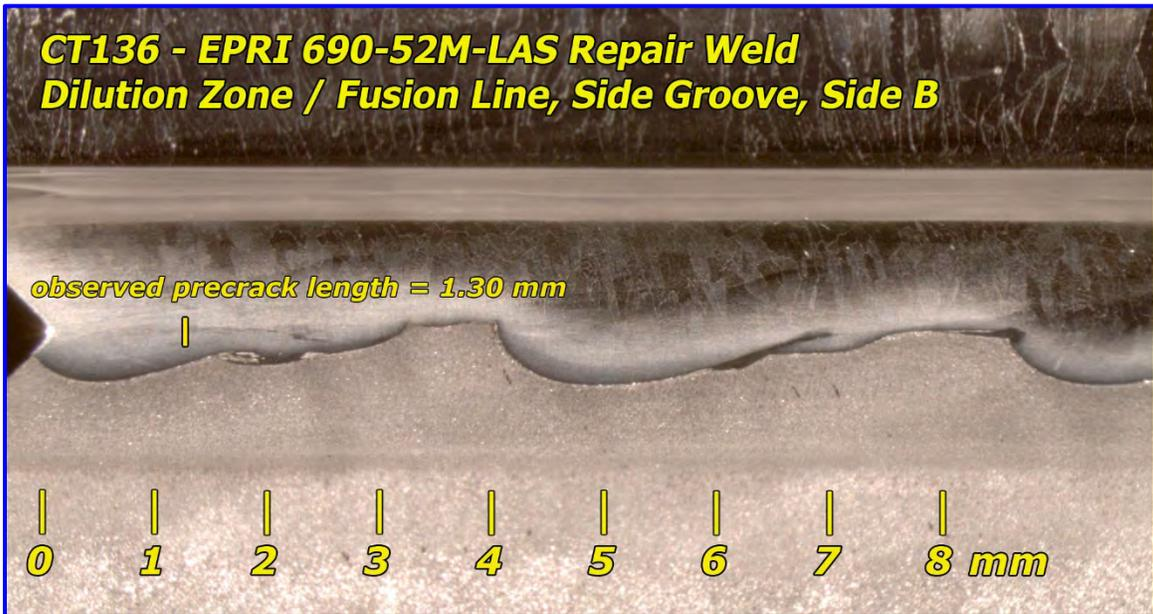
**Figure 5-19 Polished and Etched Side-Grooves of the EPRI Temper Bead DM Repair Weld Specimen CT136**
