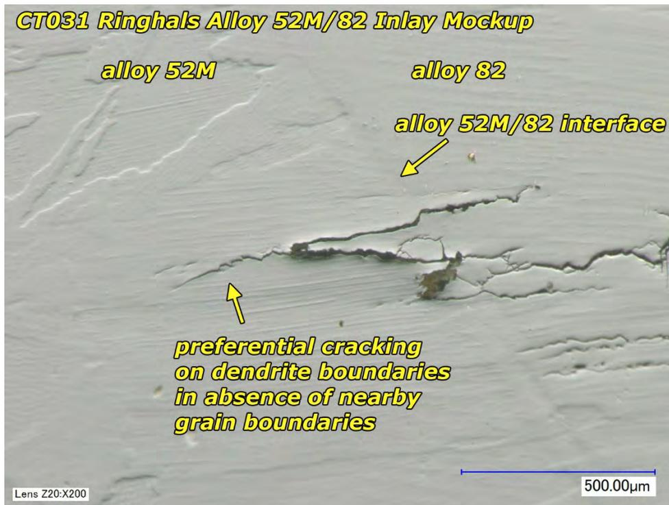
Figure 4-39 Optical Image of Side Surface of Crack Growing into Alloy 52M in the Ringhals Alloy 52M/82 Specimen CT031
