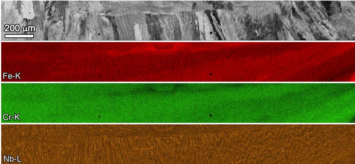
Figure 5-10 SEM-EDS Composition Maps from the Area near Aligned Grain Boundary #1
