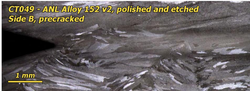
**Figure 3-37** Optical Images of the Polished and Etched Side Grooves for the First Specimen (CT049) Cut from the ANL Alloy 152 V2 Weldment. Grain Shape Is Highly Variable, but Based on These Side-Groove Observations the Geometric Crack Path Is Well Aligned with the Grain Boundaries of the Elongated Grains
