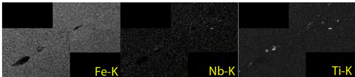
**Figure 3-121 STEM-BF Image and EDS Elemental Maps of the Weld Crack in CT043 from the Yellow Dashed Box in Figure 3-120. At Higher Magnification, Small (100 nm) Nb-Rich Precipitates Are Observed on the Grain Boundary**
