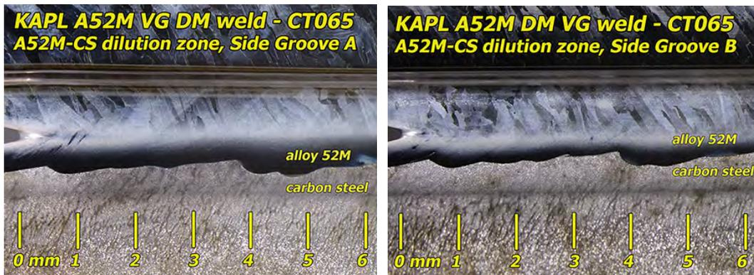
Figure 5-5 Polished and Etched Side Grooves of the Alloy 52M/CS Dilution Zone Specimen (CT065) Showing That the Crack Growth Plane Is ~0.5 mm into the Alloy 52M
