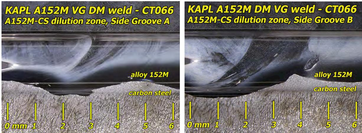
**Figure 5-6 Polished and Etched Side Grooves of the Alloy 152M/CS Dilution Zone Specimen (CT066) Showing That the Crack Growth Plane Is ~0.5-1.5 mm into the Alloy 152M**
