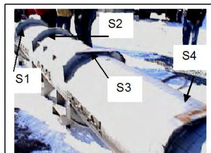
Stiffening rings show progressive damage from T/N
