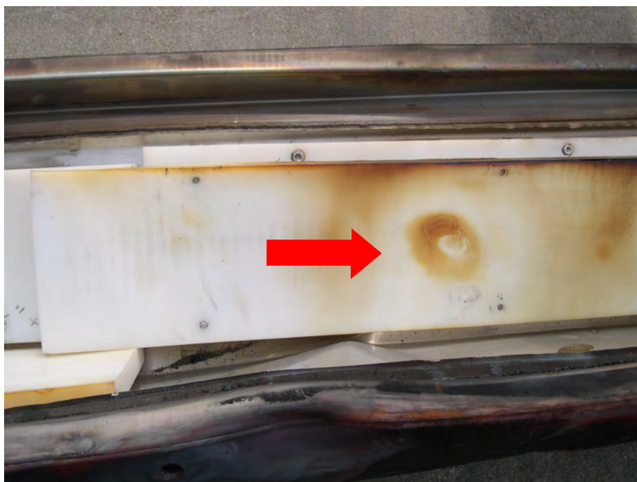
Figure 3-44 Localized Melt Spot in Lid Moderator Block
