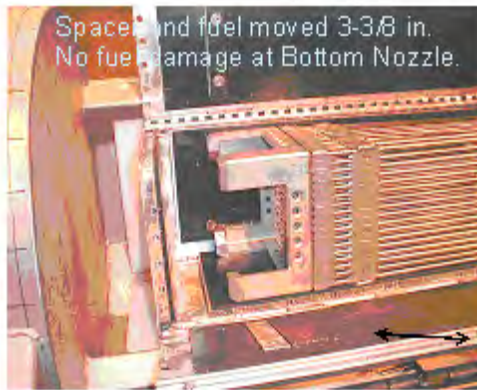
(a) FA Displacement at Bottom Nozzle End of the Package
