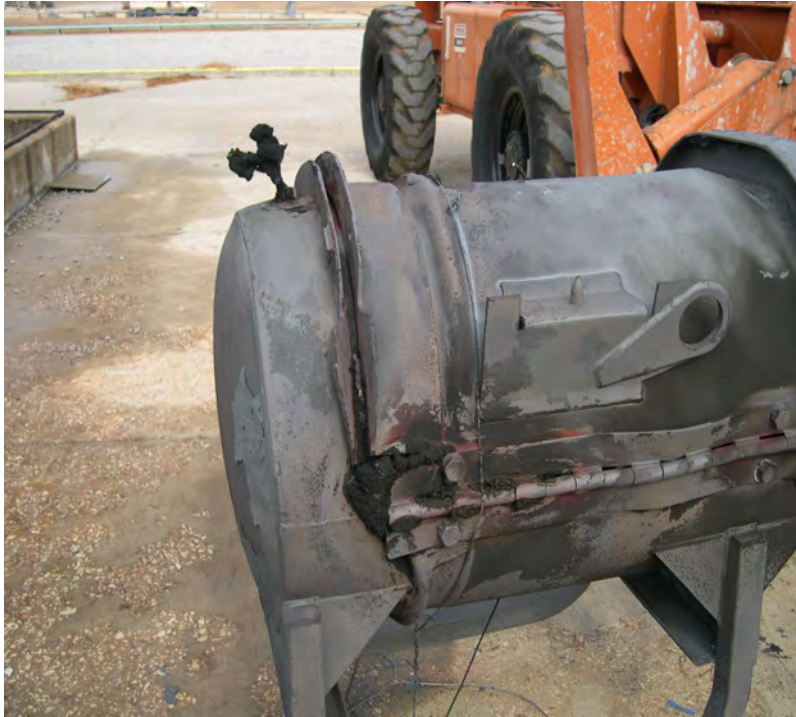
Figure 3-30 Polyurethane Char in Outerpack Seam After Burn Test
