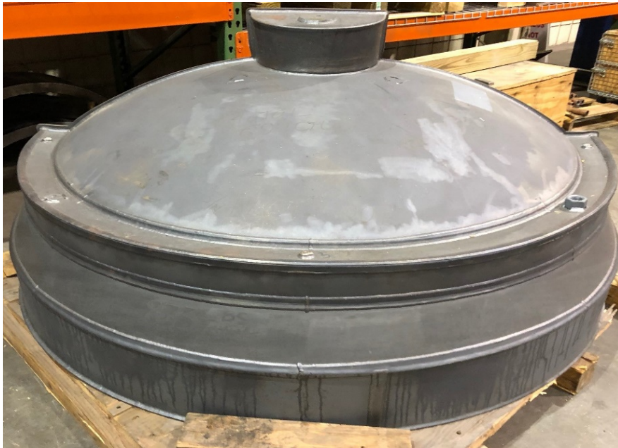
One-half Lower Reactor Head ~6500lbs (2950 kg) x 70 inches @ 2/3rds scale
