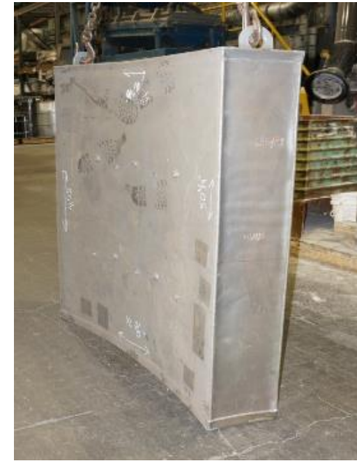
Partial RPV Ring Section
