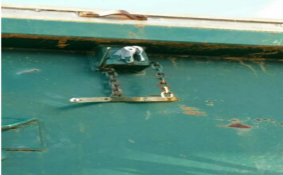
GFLU-001075 broken tie-down.
