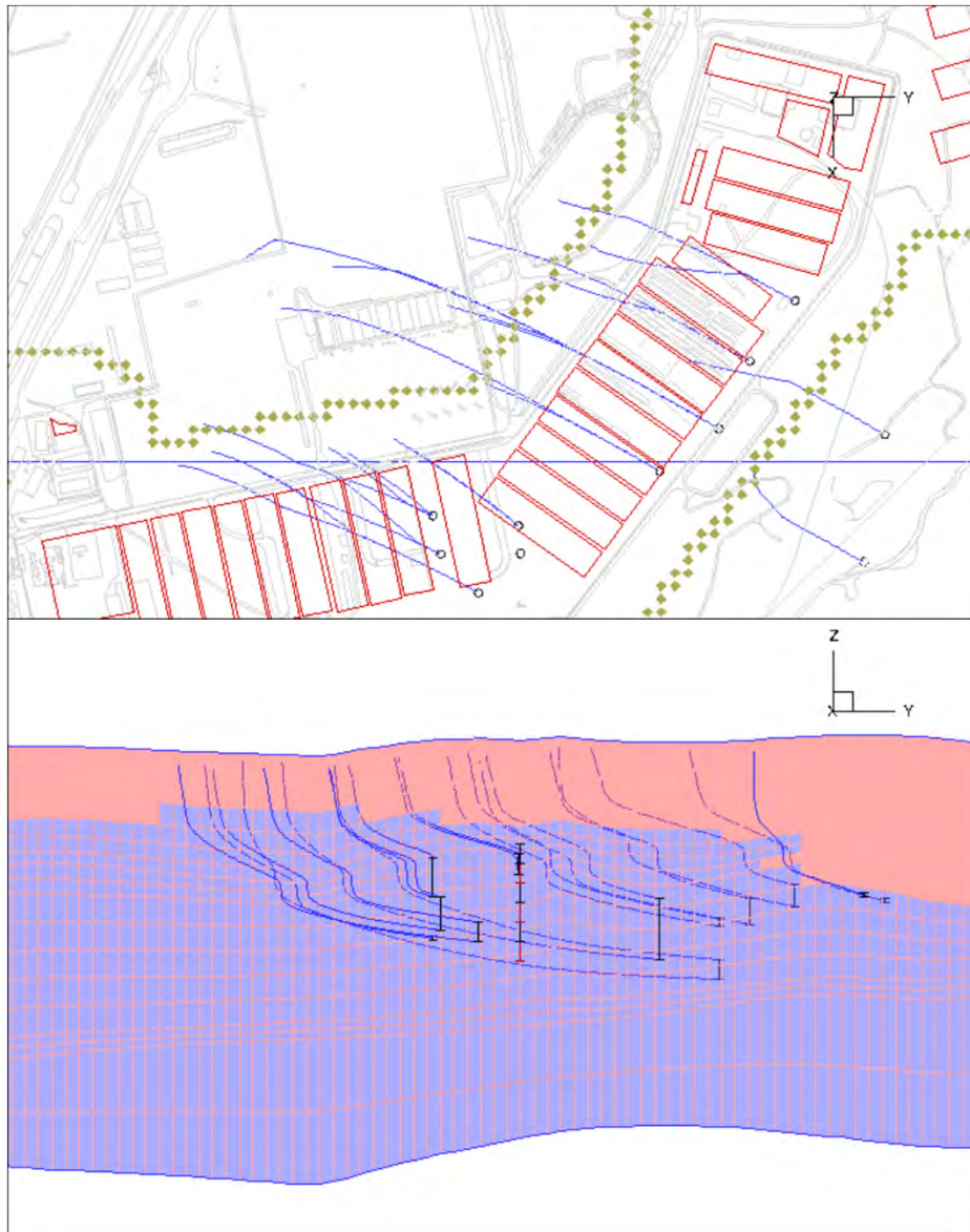
Figure 3-4. Simulated groundwater pathlines for GSA_2018 model prior to placement of low-infiltration covers.
