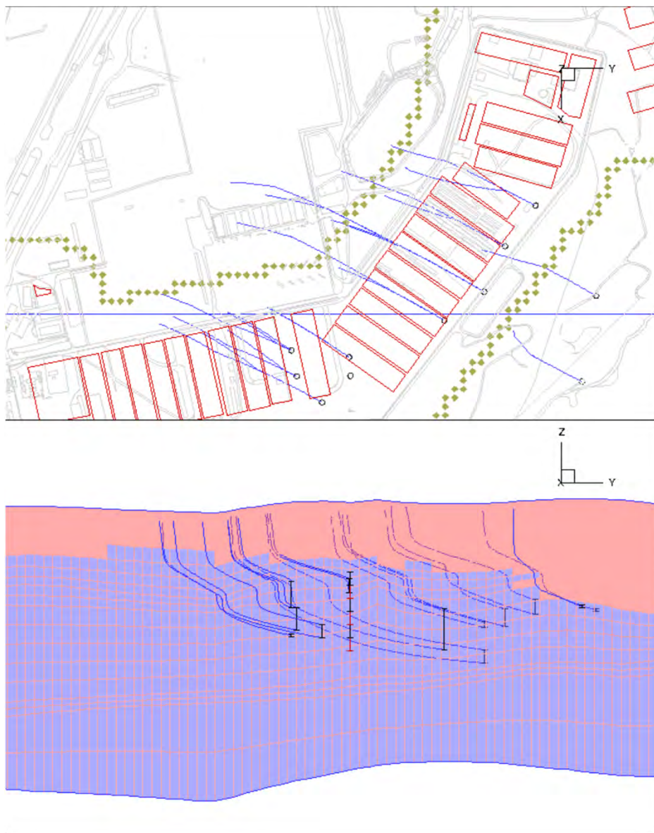
Figure 3-2. Simulated groundwater pathlines for GSA_2016 model prior to placement of low-infiltration covers.
