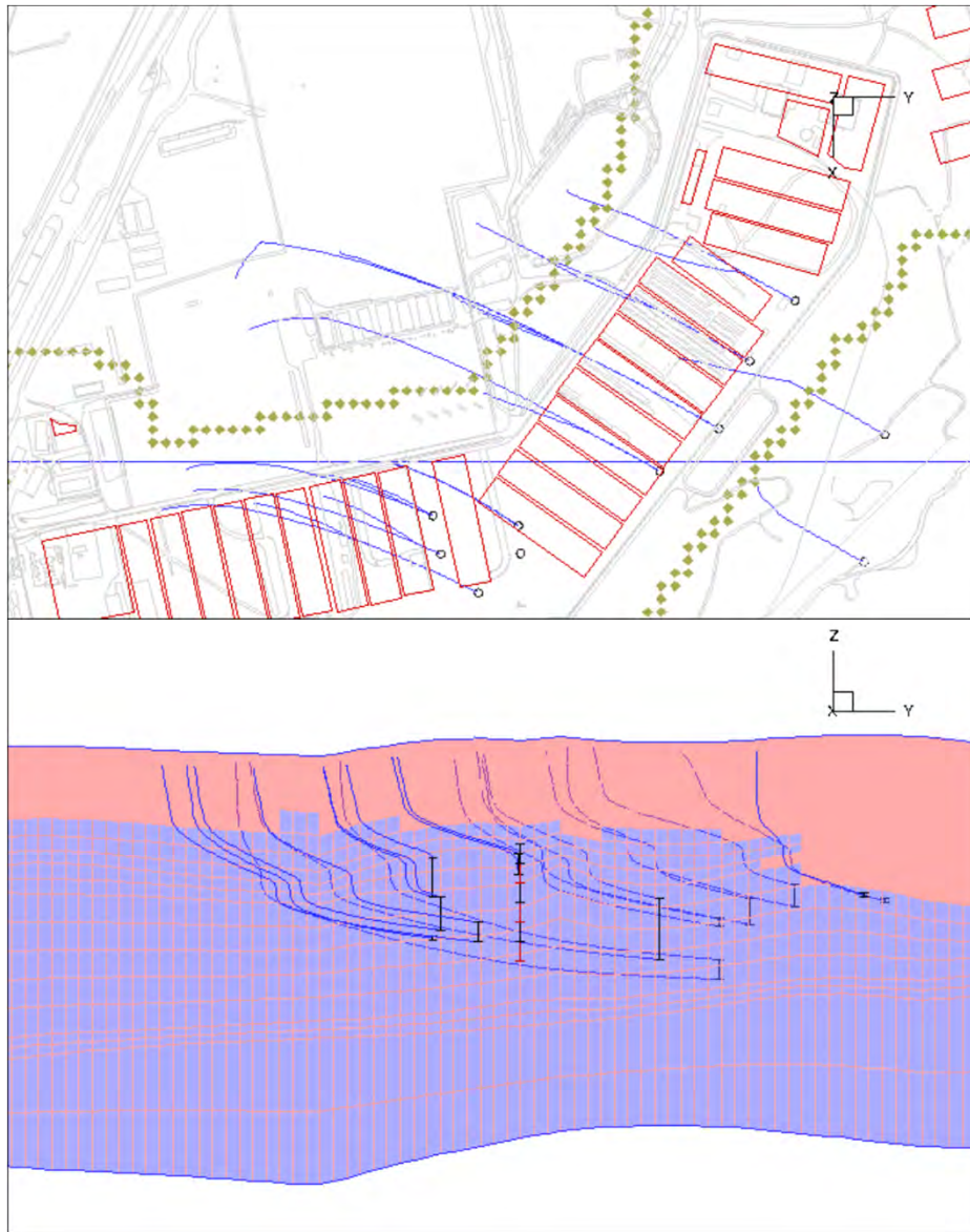
Figure 3-5. Simulated groundwater pathlines for GSA_2018 model after placement of low-infiltration covers.
