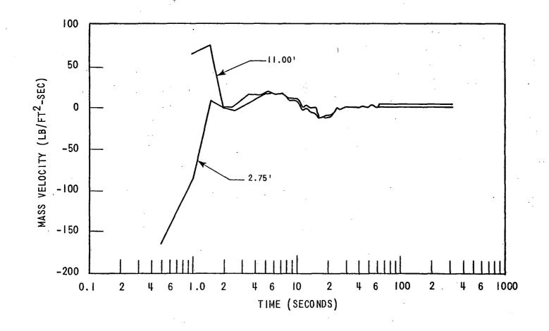
Figure 2. Mass Velocity - DECLG ( $C_D = 0.4$ )
