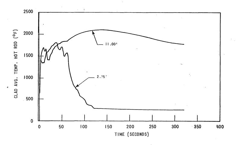
Figure 8. Peak Clad Temperature - DECLG ( $C_D = 0.4$ )
