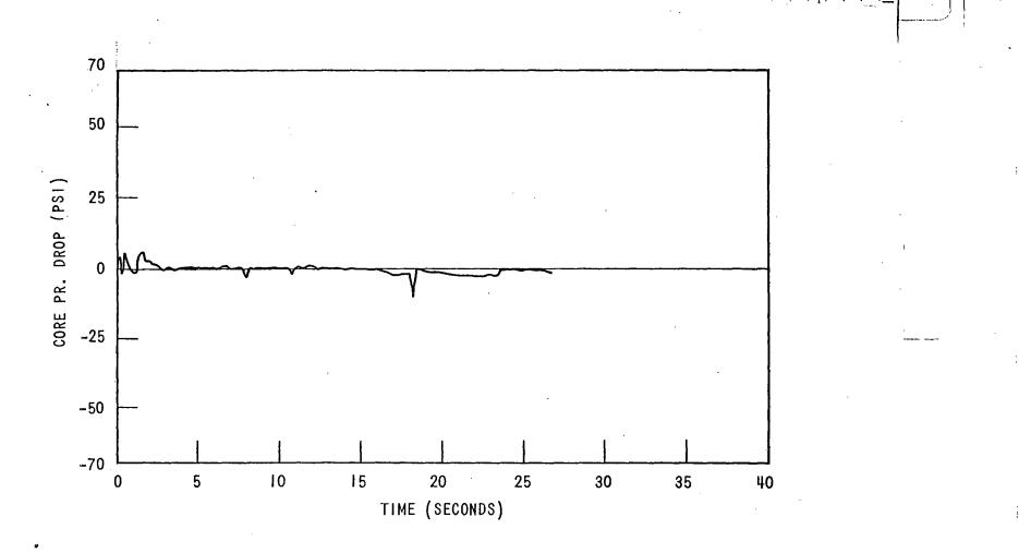
Figure 7 - Core Pressure Drop - DECLG ( $C_D = 0.4$ )
