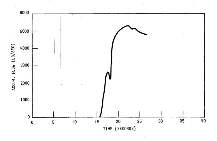
Figure 12. Accumulator Flow (Blowdown) - DECLG ( $C_D = 0.4$ )
