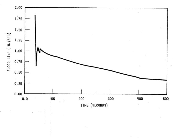
Figure 11a. Reflood Transient - DECLG ( $C_{D}$ = 0.4) Core Inlet Velocity
