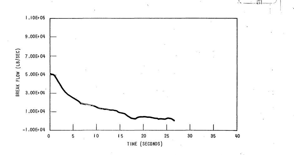
Figure 6. Break Flow Rate - DECLG ( $C_D = 0.4$ )
