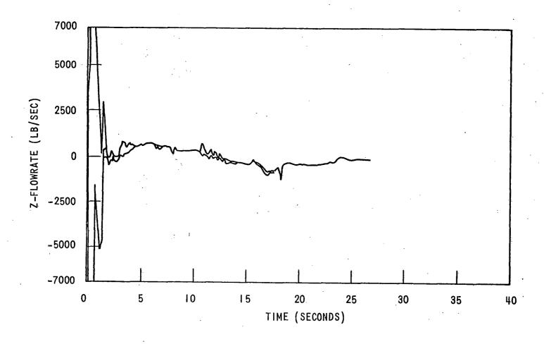
Figure 10. Core Flow - Top and Bottom - DECLG ( $C_D = 0.4$ )
