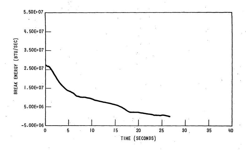
Figure 14. Break Energy Released to Containment
