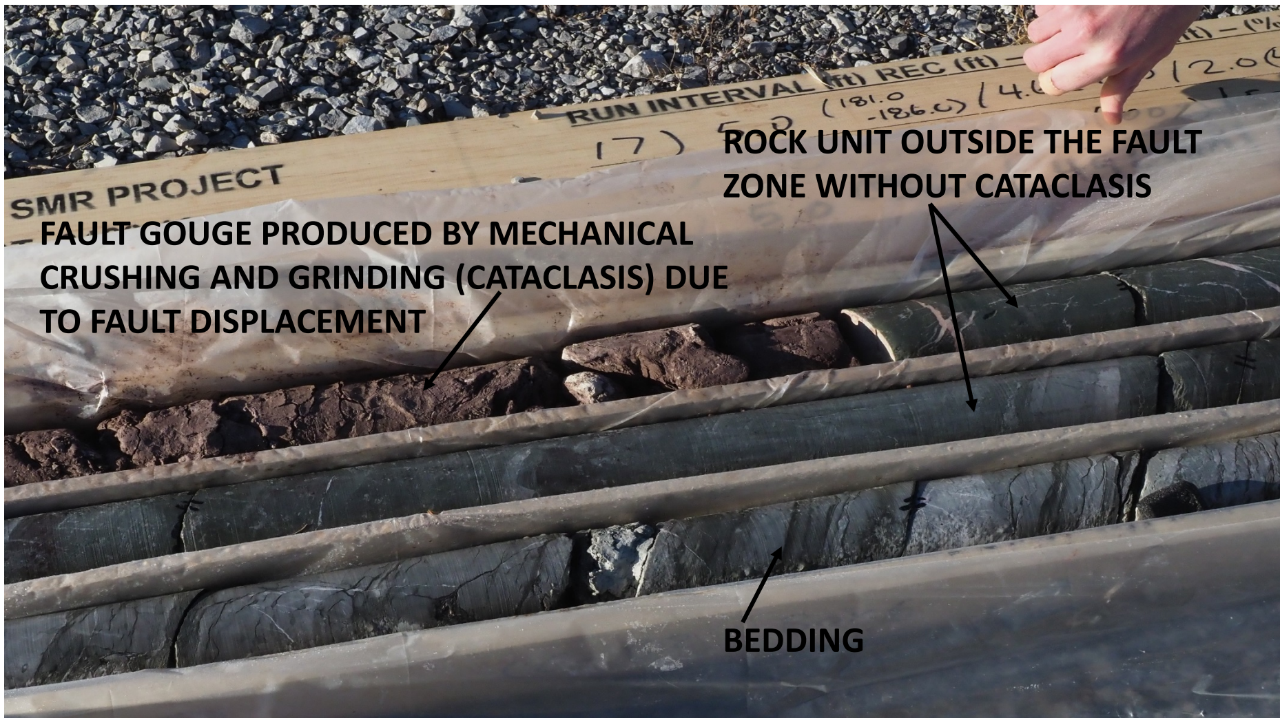
Fault gouge marking the Copper Creek Fault in Borehole CC-B2. Note the clear distinction between the gouge, dated at ~280 Ma, and intact rock. (G. Stirewalt image, January 2018)
