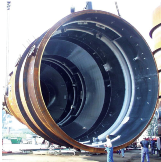
Figure 43 Vessel made from roll -bonded Ni-clad steel ; photo from Verbundmetalle GmbH.
