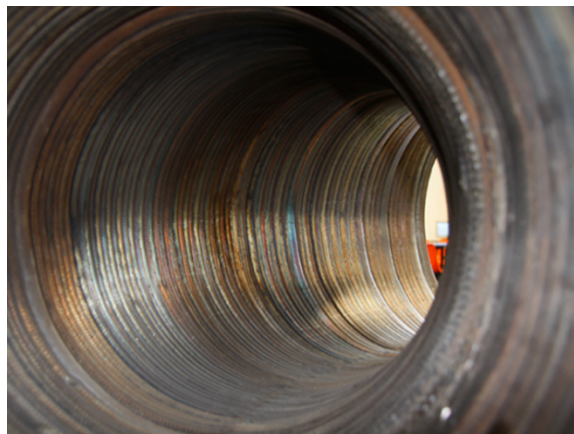
Figure 44 Weld overlay pipe fitting ; image from Chongqing GLEN Flange Limited.
