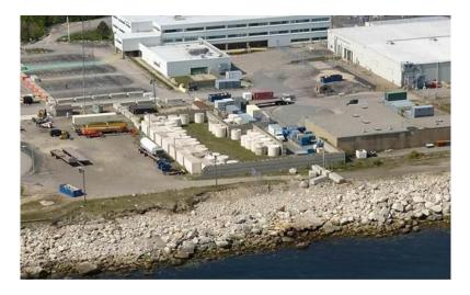
In the photograph, the white containers are for Low Level Radioactive Waste. To the right of the storage area is the LLRW building that compress materials to store or for shipment.
