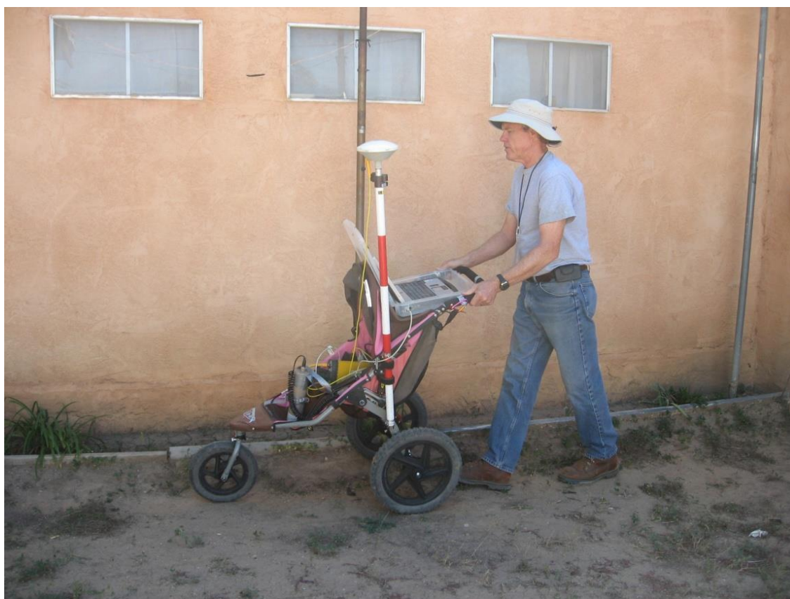
Figure 2-2 : Gamma scanning up to one acre around a house.
