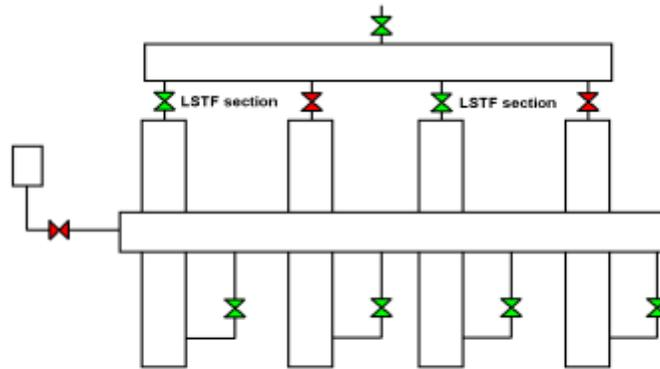
Figure 4 Nodalization of the Main Steam System
