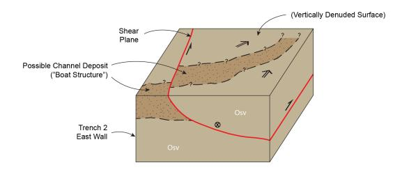
**B** Event 2 - Later block sliding along pre-existing shear plane creates extensional fracture.
