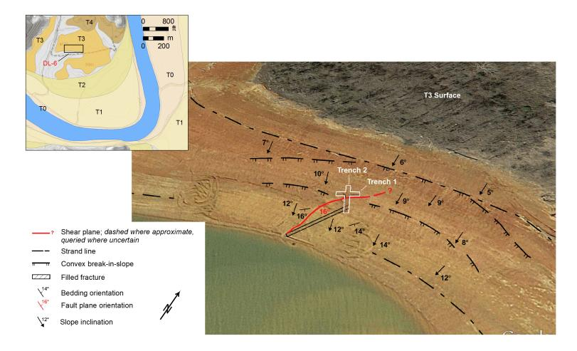
Approximate locations of References 2.5.3-12 and 2.5.3-13 trenches, filled fractures, and shear planes below T3 surface. Trench 1 and the section of Trench 2 upslope of Trench 1 were not re-excavated during field reconnaissance. Figure 2.5.3-17 shows log of the NE wall of Trench 2. Bedding orientation and slope inclination as measured during field reconnaissance.
