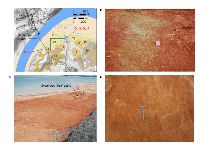
A) and B) Images from Reference 2.5.3-12 show shale-clay "boil" exposed in the NE corner of DL-5b (not exposed during field reconnaissance). C) Photo shows bleached fractures at the site (hammer for scale).
