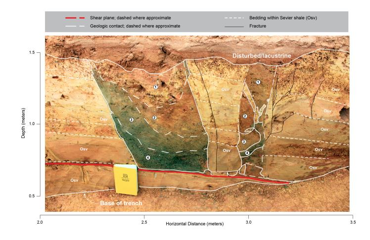
Area of figure shown as blue box in Figure 2.5.3-17 (Sheet 1 or 3). Additional excavation below the shear plane did not reveal the potentially offset alluvium filled fracture.
