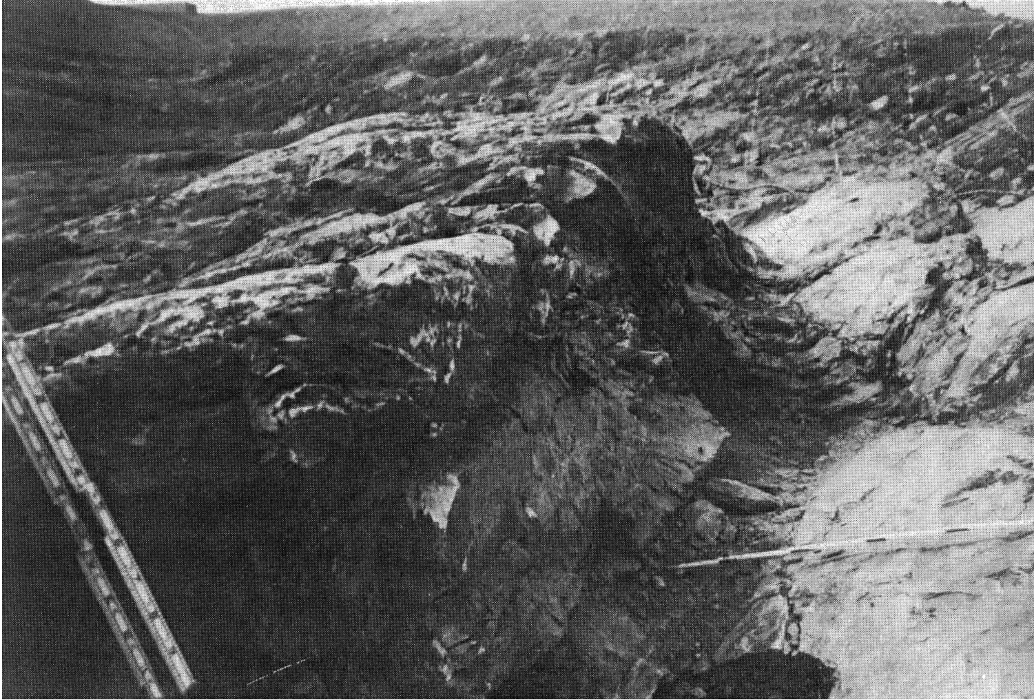
Figure 2.5.1-92. Apparent Fault Propagation Fold Exposed in CRBRP Excavation
