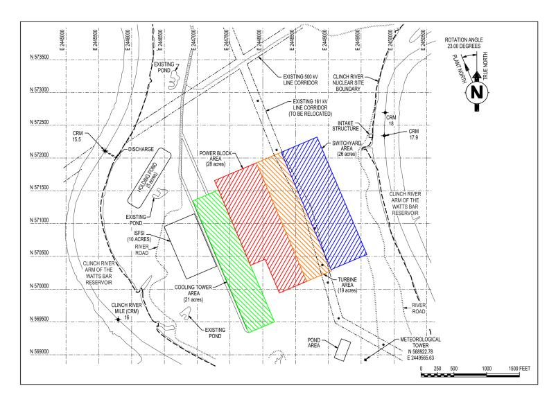
Figure 2.4.11-2. Location of the Clinch River Nuclear Site Intake Structure
