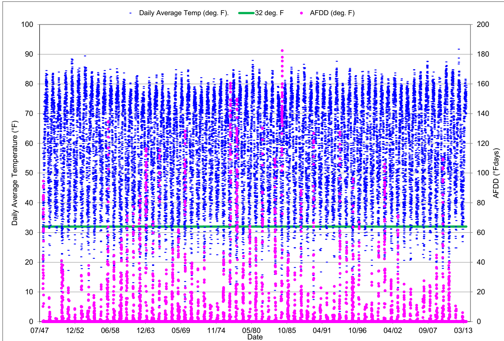
Figure 2.4.7-2. Temporal Variations of Daily Average Temperature and Accumulated Freezing Degree-Days for about 65-year Period of Record
