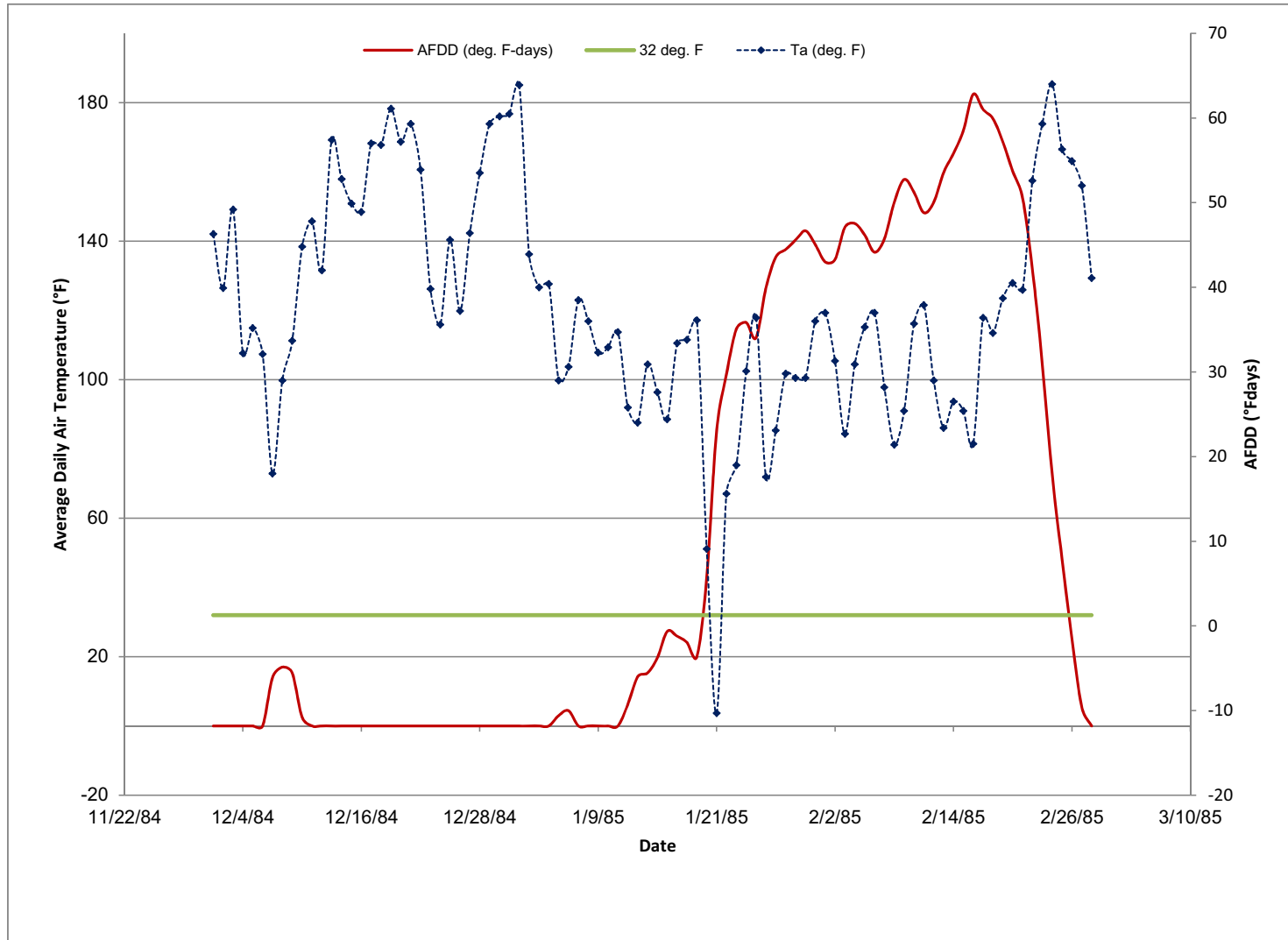
Figure 2.4.7-4. Temporal Variations of Daily Average Temperature and Accumulated Freezing Degree-Days for Winter of 1984/1985
