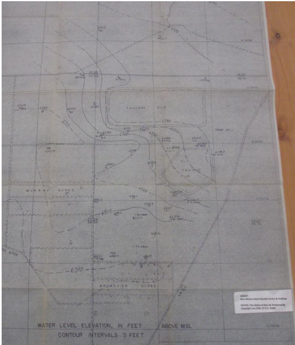
Figure 29: Snapshot of Water Level Elevation, dated 1976 as drawn. UNHP Mill and Vicinity. United Nuclear Homestake Partnership, Milan, New Mexico. (Science and Engineering Resources, Inc. 1976) Socorro, New Mexico.
