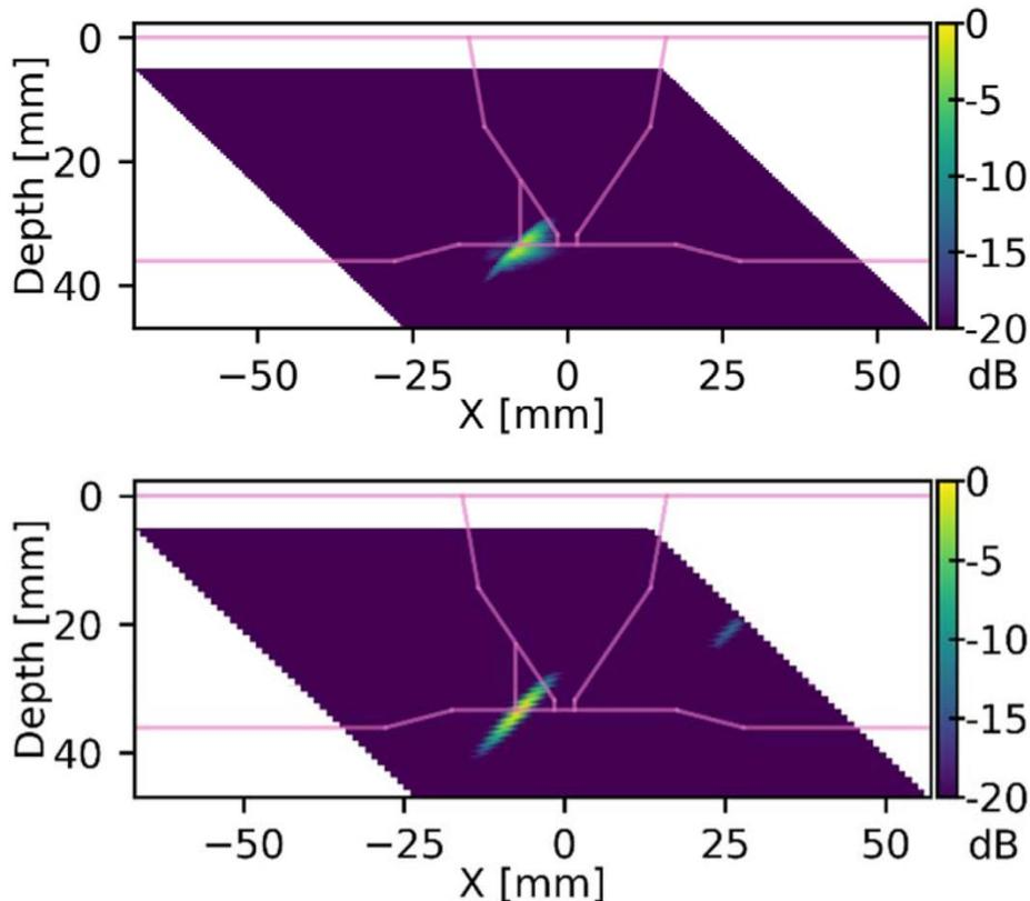
**Figure 6.9. B-scan for near side inspection using a 0.5 in. diameter, 2 MHz, 45° shear wave transducer. *Top: experiment, bottom: simulation.* The weld profile and location of the saw-cut flaw are overlaid on the B-scan. The B-scans are normalized to their own maximum signal amplitude. The color maps span amplitudes down to  $-20$  dB from the maximum.**
