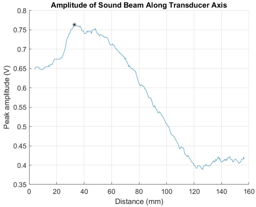
**Figure A.20. Sound beam profile for Transducer #7.**
