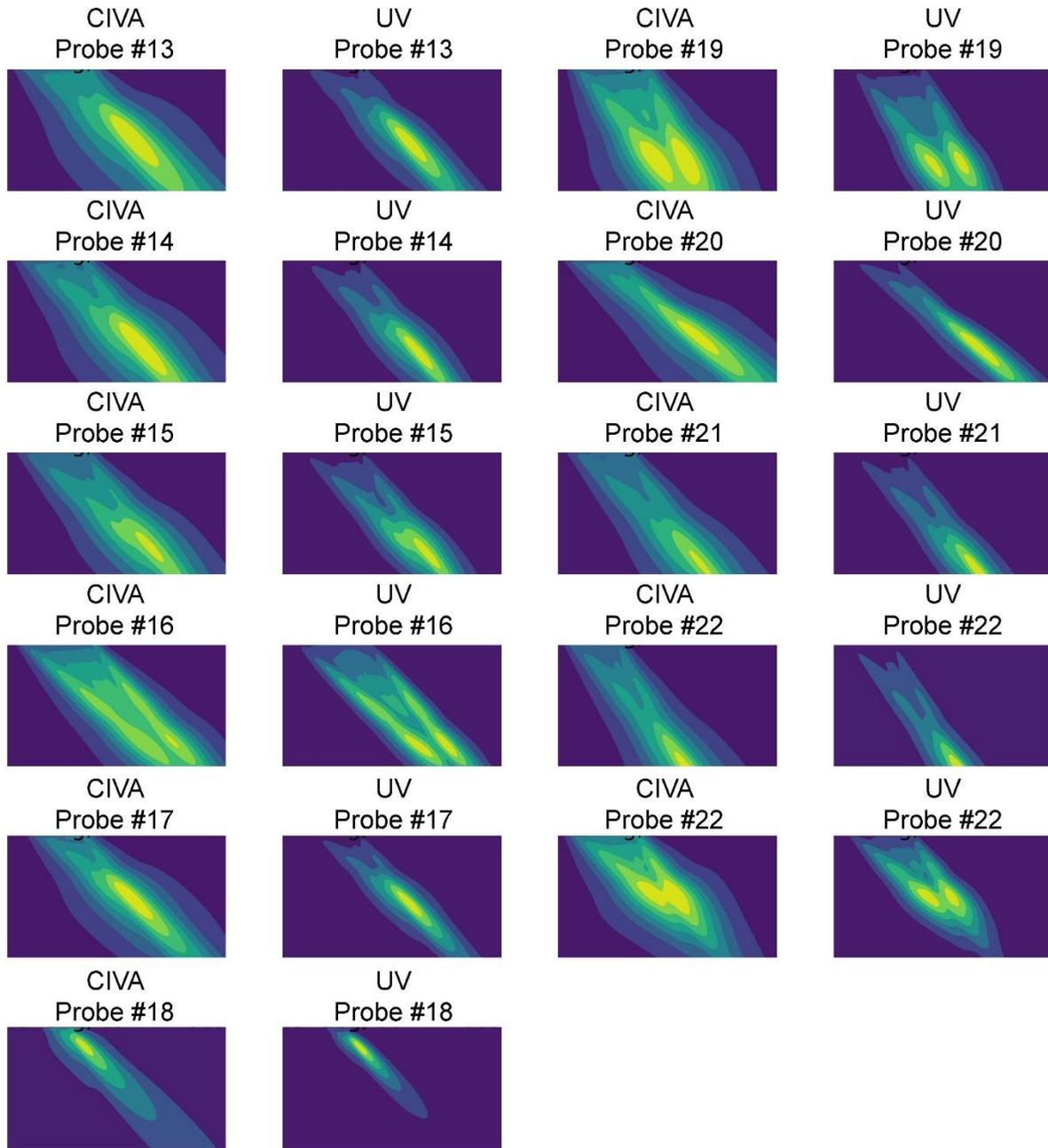
**Figure 3.2.** Beam simulations for the 11 dual-element transmit receive longitudinal wave probes using CIVA and UV. The specifications of the probes are indicated in the title of each beam as (frequency, diameter, beam angle, mode). The color map color range for each simulation shown is normalized relative to its own maximum amplitude.
