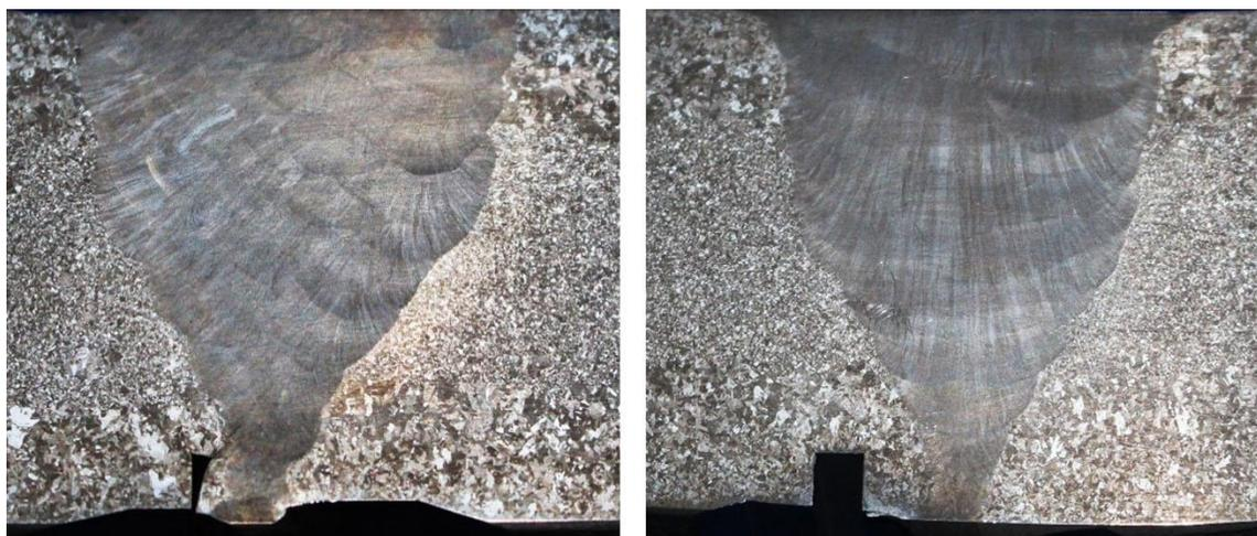
**Figure 4.3. Macrographs of the weld within Specimen 1 (*left*) and Specimen 2 (*right*).**
