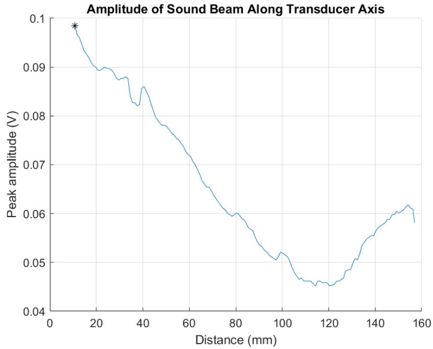
**Figure A.18. Sound beam profile for Transducer #5.**
