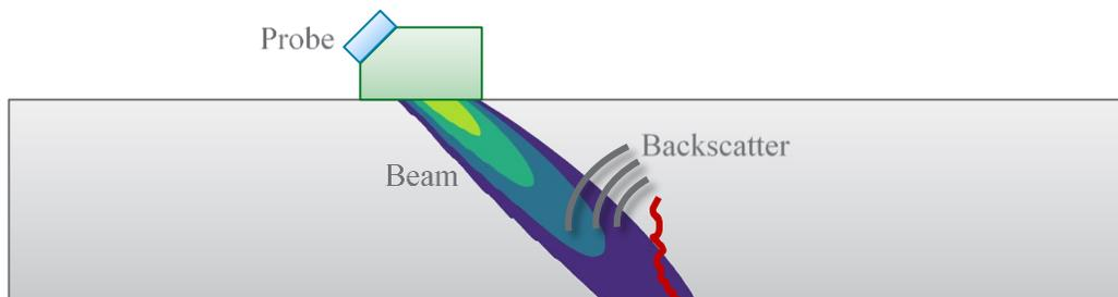
**Figure 5.1. Cross-sectional view of a beam simulation. The amplitude of the beam incident at the back-wall is  $-12$  dB relative to the maximum beam amplitude (which is always at the near-field/far-field transition point). The beam contours show color gradations in  $-3$  dB steps.**
