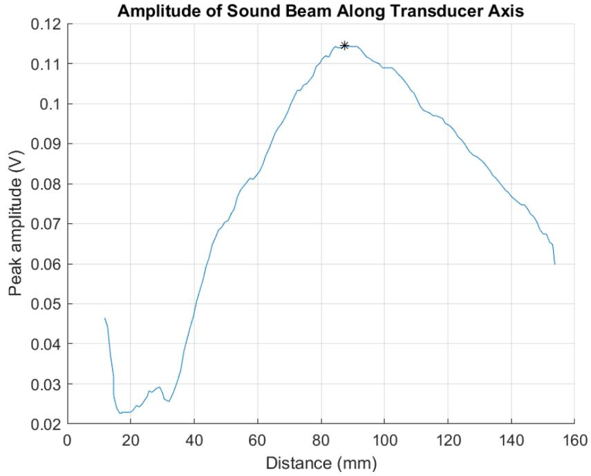
**Figure A.16. Sound beam profile for Transducer #3.**
