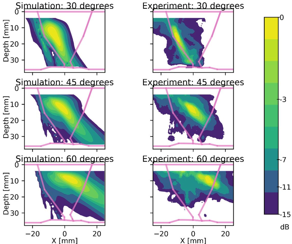
**Figure 4.9. Simulated and experimental sound beams using the phased array probe at 30°, 45°, and 60° angles through Specimen 1. The weld root is located at X=0 mm. Each beam map is normalized to itself.**
