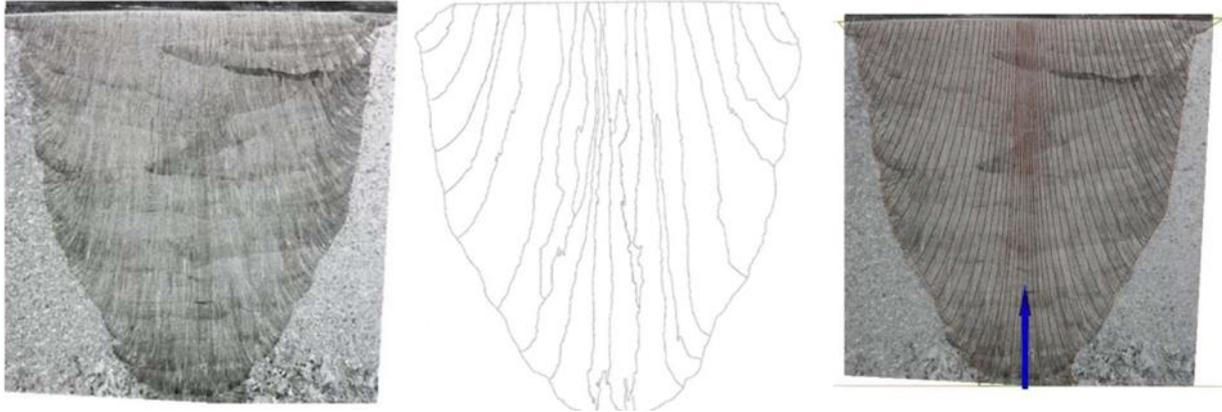
**Figure 2.1. Macrograph showing the dendrites within a weld (*left*), the dendrites boundaries defining multiple homogeneous regions of the weld (*middle*), and parametric definition of continuously changing domains (*right*). The parametric definition (*right figure*) requires a reference coordinate system, as indicated by the blue arrow.**
