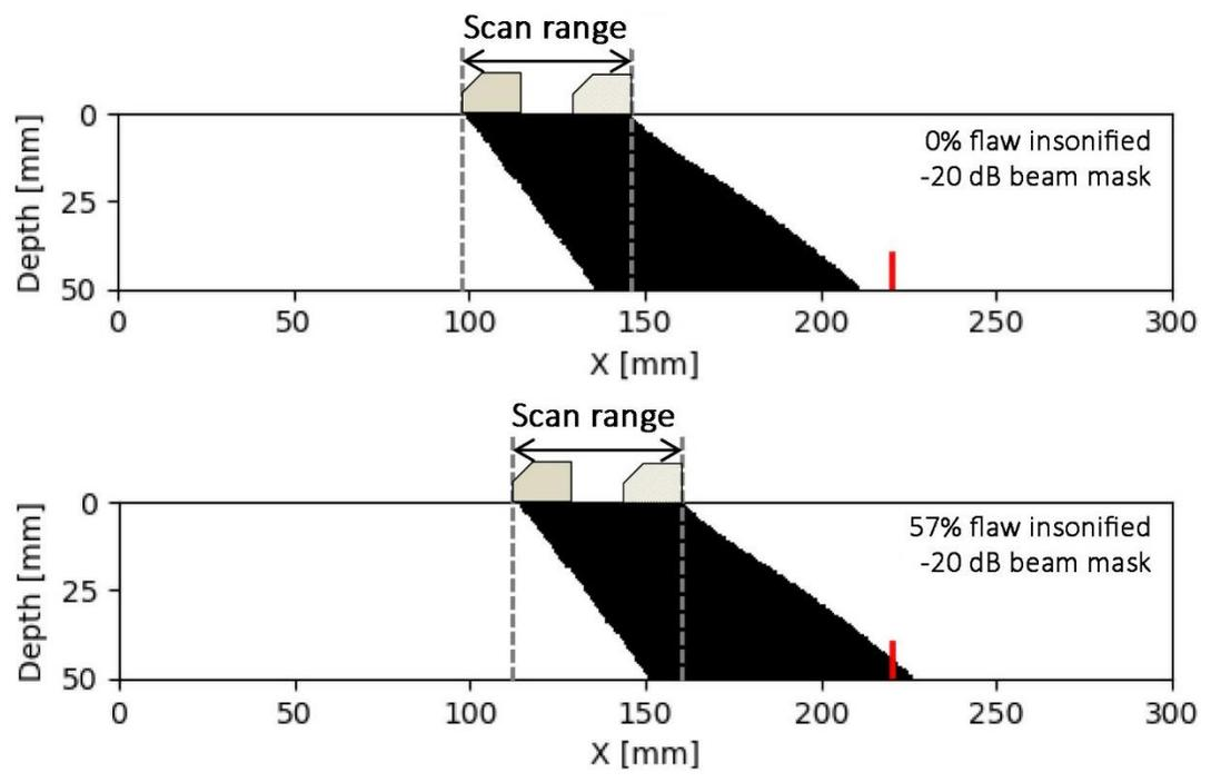
**Figure 5.11. Example of a scenario where a probe has a limited scan range due to access restrictions at the specimen surface. The middle panel shows no flaw insonification and the bottom panel shows partial flaw insonification.**
