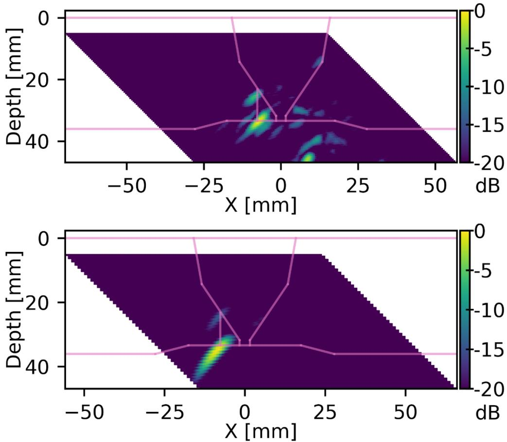
Figure 6.6. B-scan for near-side inspection using a 10x5 phased array longitudinal probe at 2 MHz, 45° longitudinal wave, and 35 mm (1.38 in.) depth focus. *Top*: experiment, *bottom*: simulation. The weld profile and location of the saw-cut flaw are overlaid on the B-scan. The B-scans are normalized to their own maximum signal amplitude. The color maps span amplitudes down to -20 dB from the maximum.
