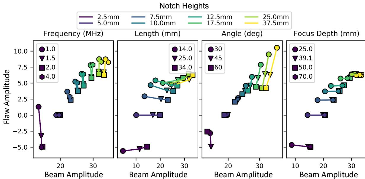
**Figure 5.9. Normalized beam metric vs. normalized flaw backscatter amplitude for the TRL probes with eight different notch heights. One probe parameter was changed at a time from left to right—frequency, probe size (length x width), beam angle, and focal distance.**
