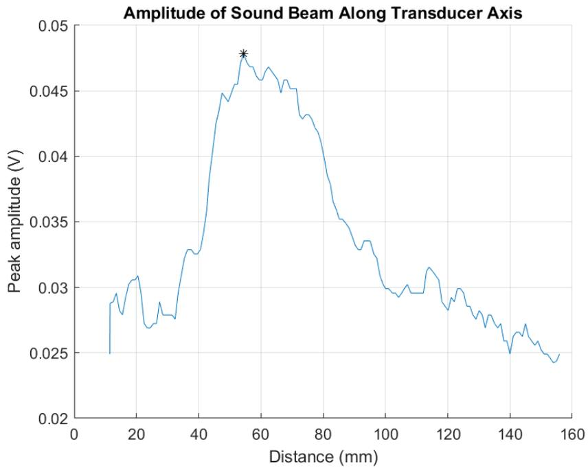
**Figure A.21. Sound beam profile for Transducer #8.**
