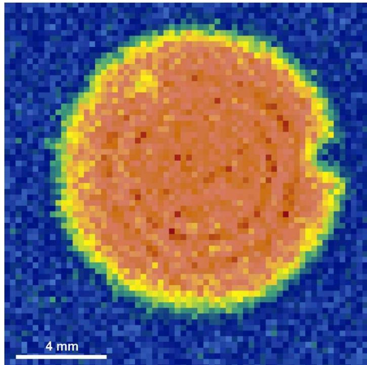
**Figure A.38. Probe face scan of Transducer #3.**
