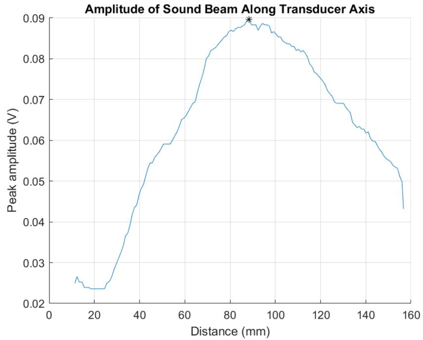
**Figure A.23. Sound beam profile for Transducer #10.**
