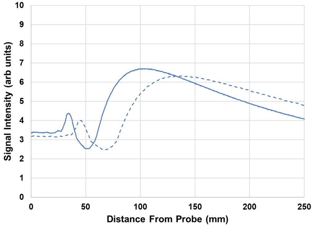
Figure A.47. Solid line: Beam profile generated in CIVA for Transducer #5. Dashed line: Beam profile generated in CIVA for the nominal transducer.
