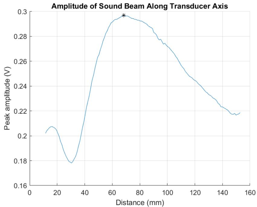
**Figure A.15. Sound beam profile for Transducer #2.**
