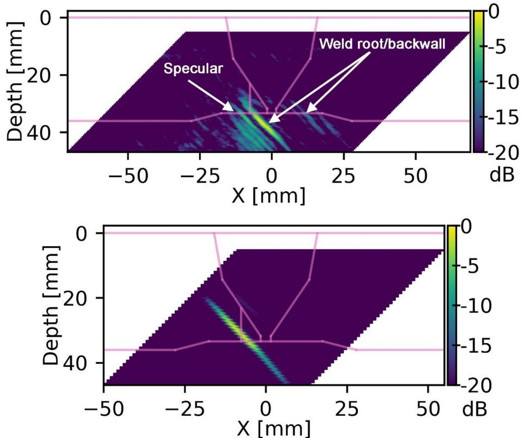
**Figure 6.5. B-scan for far side inspection using a dual-element TRL probe at 2 MHz, 45° longitudinal wave. *Top*: experiment, *bottom*: simulation. The weld profile and location of a saw-cut flaw are overlaid on the B-scan. The B-scans are normalized to their own maximum signal amplitude. The color maps span amplitudes down to -20 dB from the maximum.**
