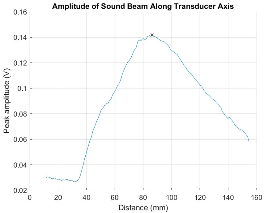
**Figure A.19. Sound beam profile for Transducer #6.**
