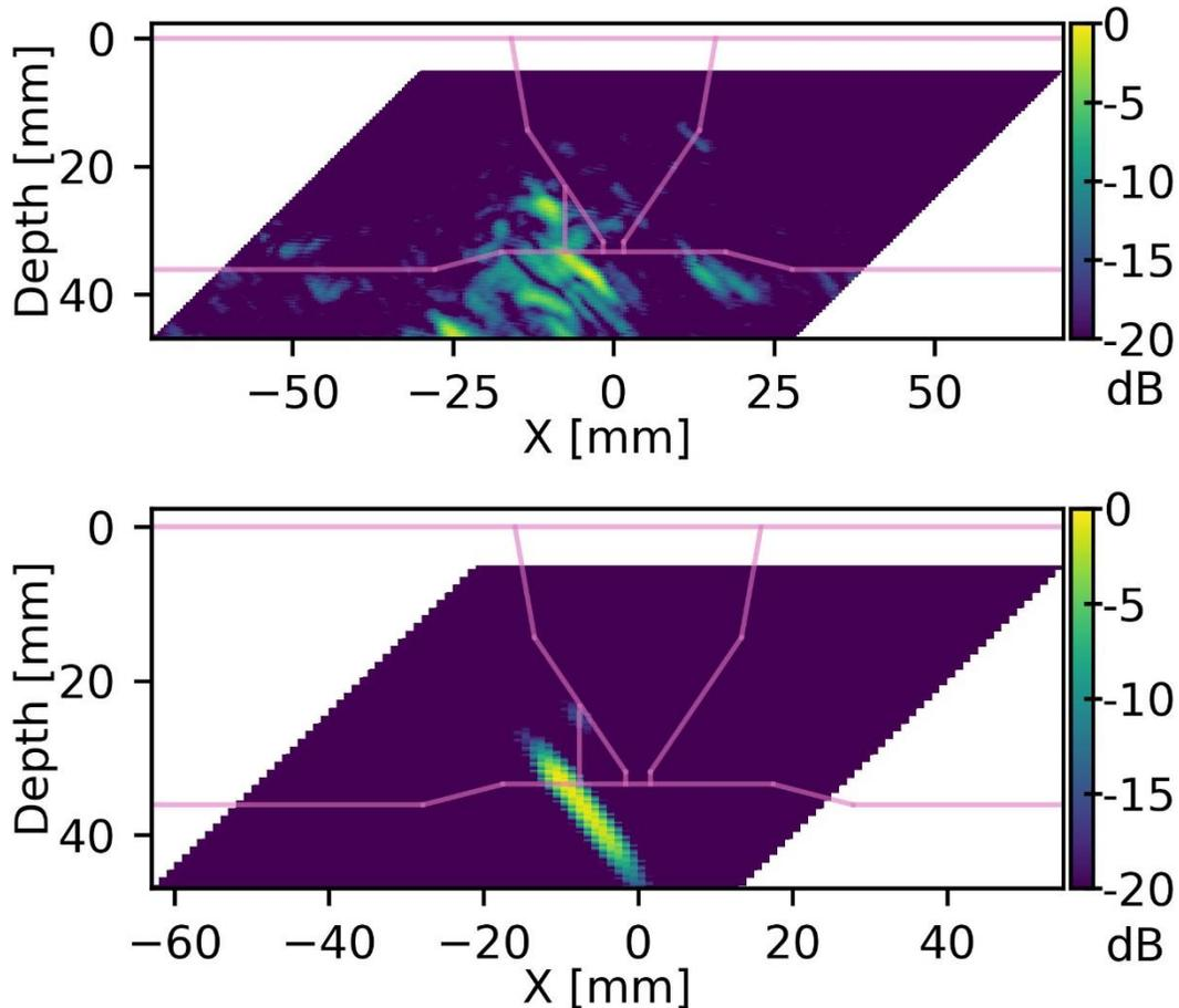
**Figure 6.7. B-scan for far-side inspection using a 10x5 phased array longitudinal probe at 2 MHz, 45° longitudinal wave, and 35 mm (1.38 in.) depth focus. *Top*: experiment, *bottom*: simulation. The weld profile and location of the saw-cut flaw are overlaid on the B-scan. The B-scans are normalized to their own maximum signal amplitude. The color maps span amplitudes down to -20 dB from the maximum.**
