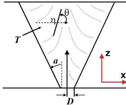
**Figure 2.3. Definition of the Ogilvy geometrical weld model.**
