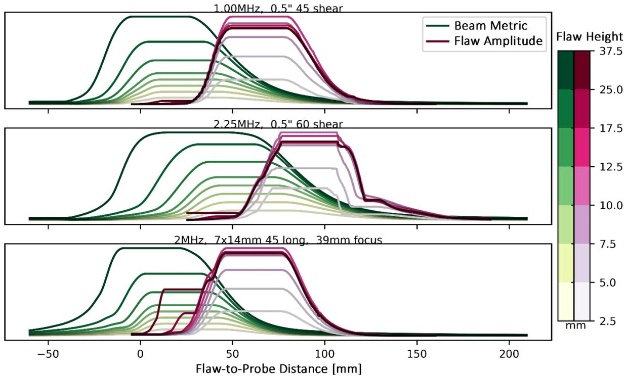
**Figure 5.13.** The flaw backscatter amplitude vs. flaw-to-probe distance is shown in shades of red. The total beam amplitude incident onto the flaw for different flaw-to-probe distances is shown in shades of green. The different shades refer to different flaw sizes, as indicated by the color bars.
