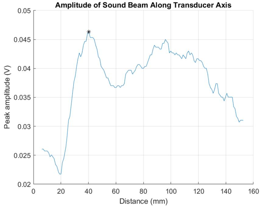
Figure A.24. Sound beam profile for Transducer #11.
