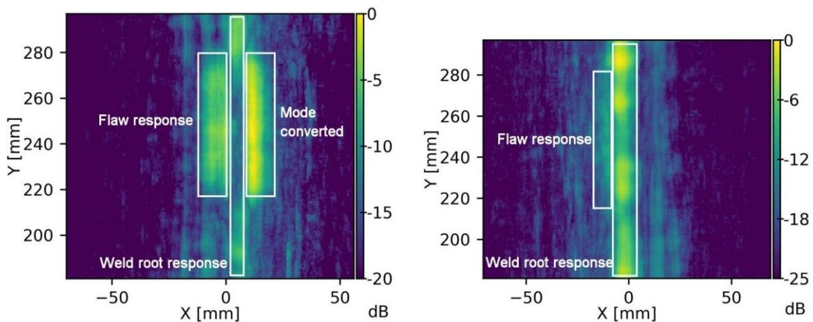
Figure 6.4. Experimental C-scan using the dual-element TRL probe at 2 MHz, 45° longitudinal wave. *Left*: near side inspection, *right*: far side inspection. The C-scan is normalized to its own maximum amplitude.
