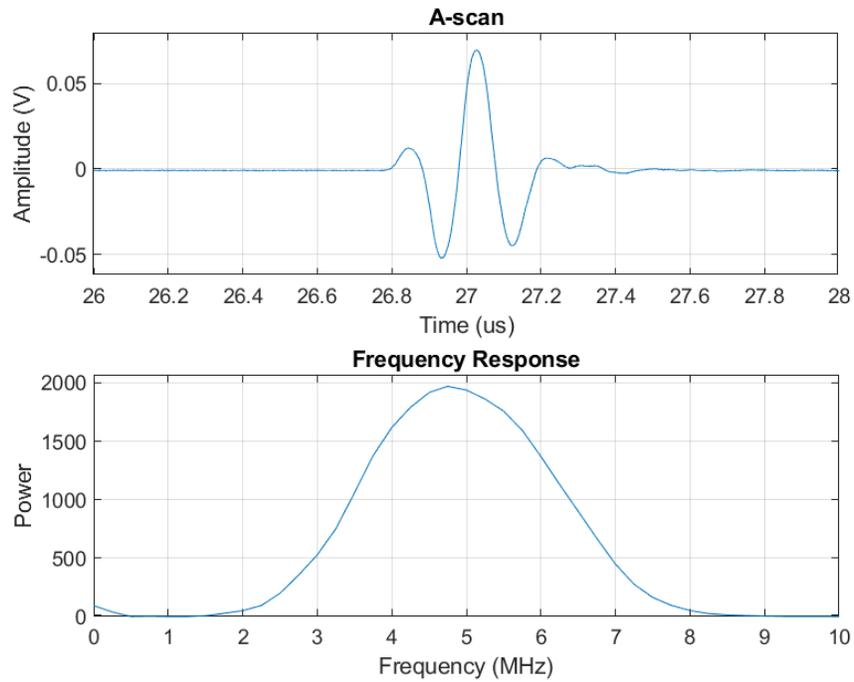
**Figure A.11. Time and frequency response for Transducer #10.**
