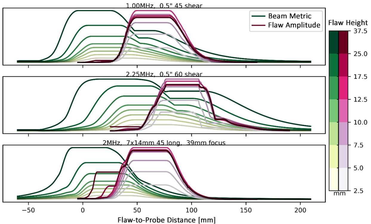
**Figure 5.16. The flaw backscatter amplitude vs. flaw-to-probe distance is shown in shades of red. The total beam amplitude (direct + backwall reflected) incident onto the flaw for different flaw-to-probe distances is shown in shades of green. The different shades refer to different flaw sizes, as indicated by the color bars.**
