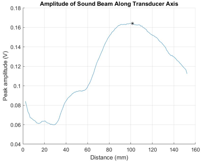
**Figure A.22. Sound beam profile for Transducer #9.**
