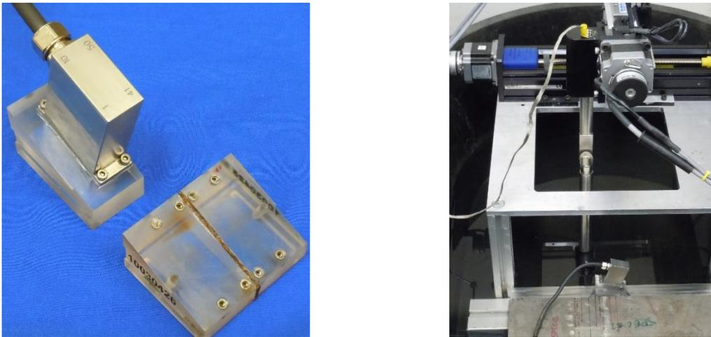
**Figure 4.4. Phased-array probe (transmit only) used for transmitting a beam through the specimen (*left*). Only half of the wedge was used (the full wedge is shown for comparison). The probe is shown positioned on a specimen for beam mapping (*right*).**
