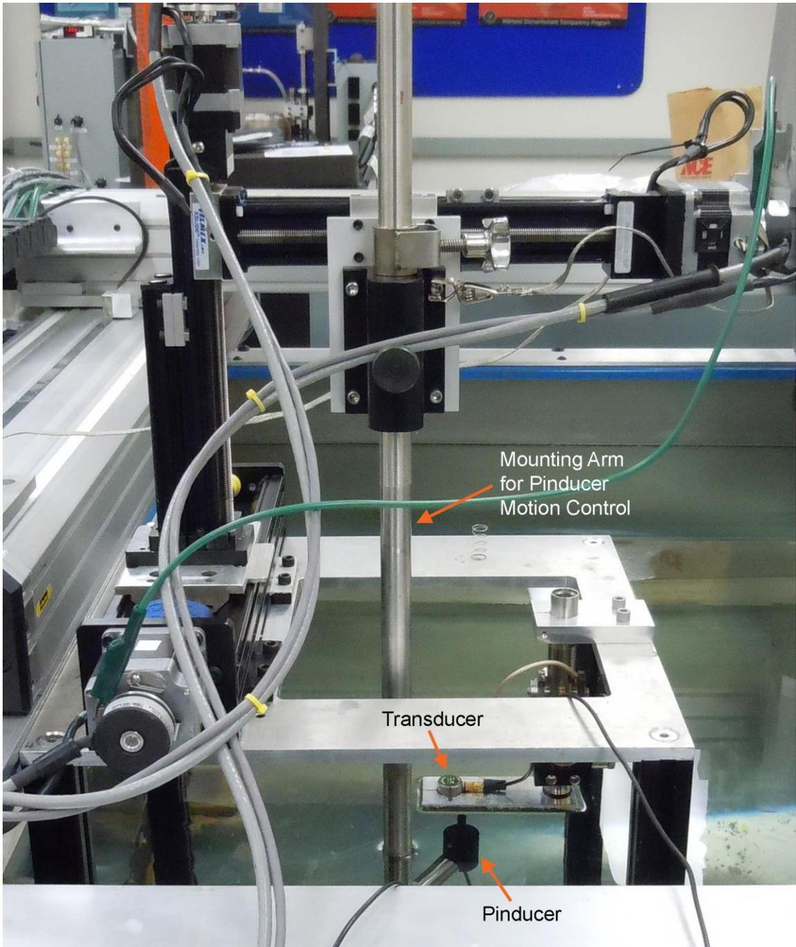
**Figure 7.10** The scanning apparatus with a mounted transducer and pinducer.
