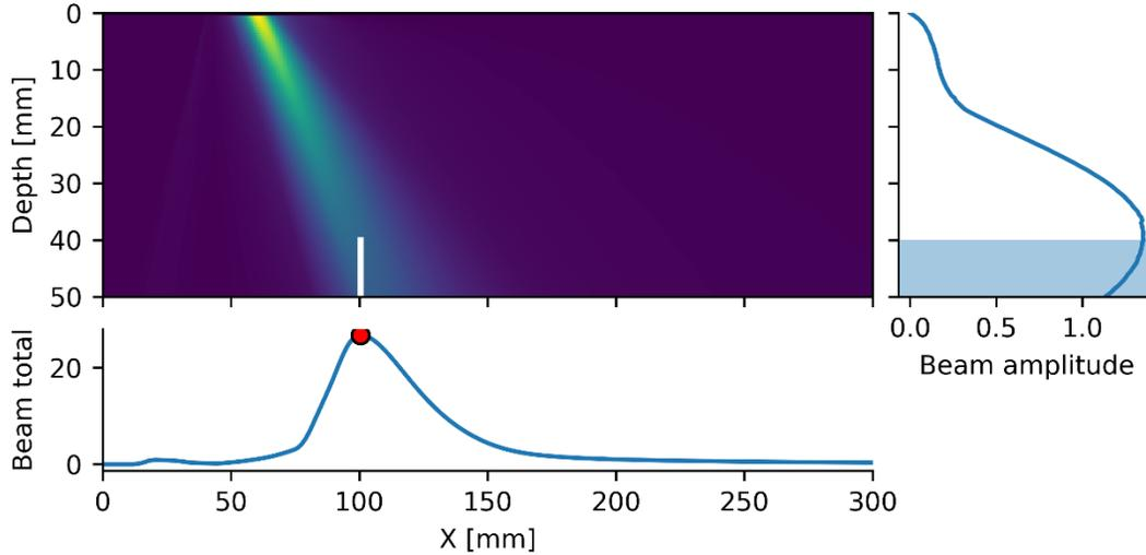
**Figure 5.4. Computation of the total beam amplitude incident onto flaw.**
