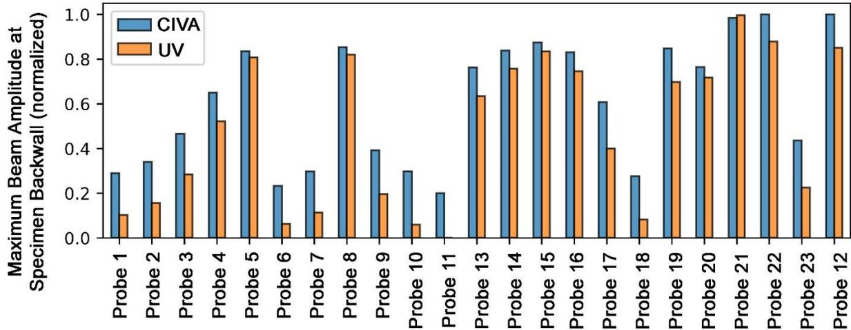
**Figure 3.3. Computed beam maximum at specimen backwall (50 mm [1.97 in.] depth) for each of the 23 probes in CIVA and in UV. Each simulation was normalized to its own maximum beam amplitude.<sup>1</sup>**
