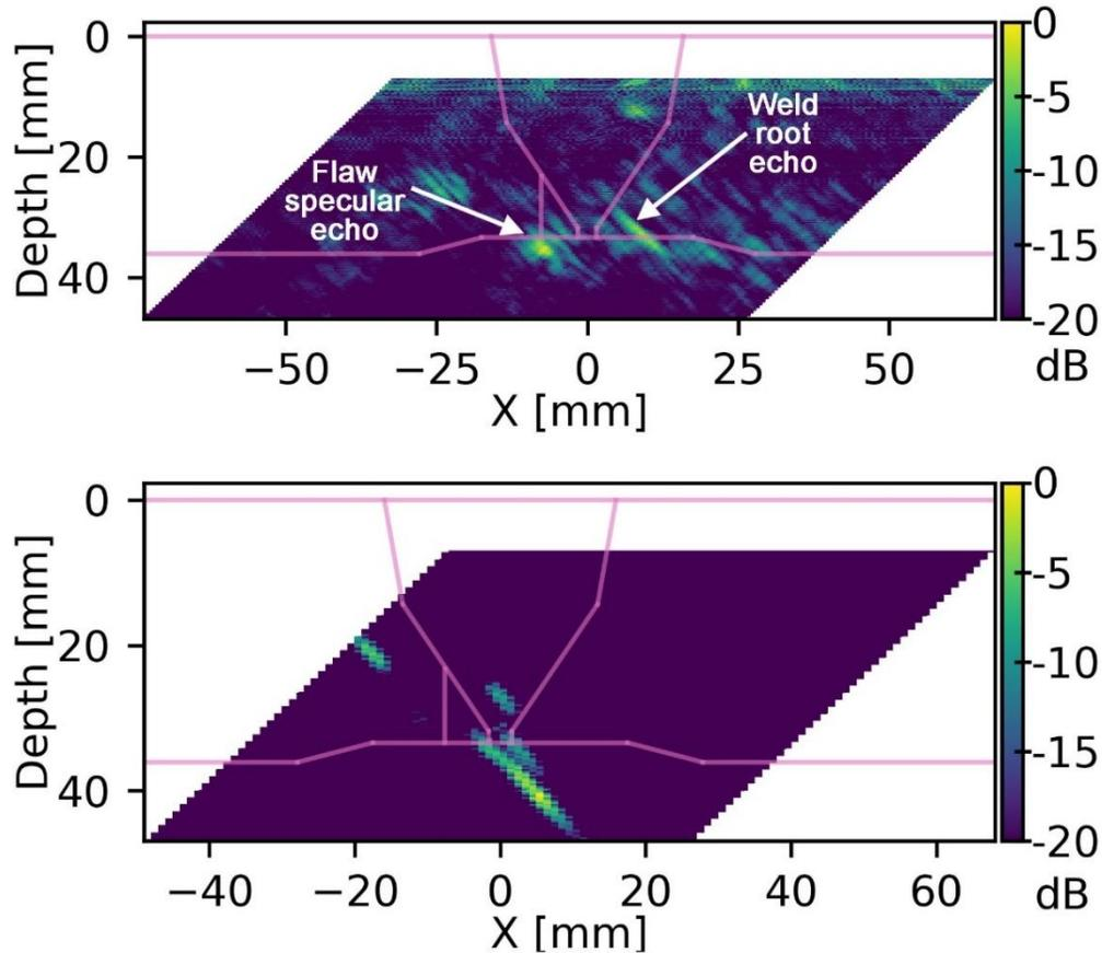
**Figure 6.11.** B-scan for far side inspection using a 0.5 in. diameter, 2 MHz, 45° shear wave transducer. *Top:* experiment, *bottom:* simulation. The weld profile, and location of the saw-cut flaw are overlaid on the B-scan. The B-scans are normalized to their own maximum signal amplitude. The color maps span amplitudes down to -20 dB from the maximum.
