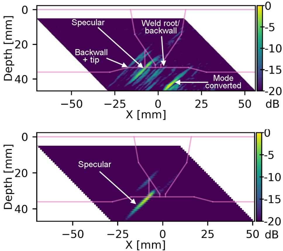
Figure 6.3. B-scan for near side inspection using a dual-element TRL probe at 2 MHz, 45° longitudinal wave. *Top*: experiment, *bottom*: simulation. The weld profile and location of saw-cut flaw are overlaid on the B-scan. The B-scans are normalized to their own maximum signal amplitude. The color maps span amplitudes down to -15 dB from the maximum.
