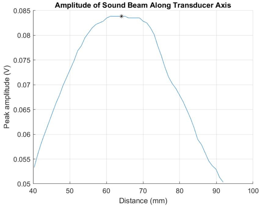
**Figure A.17. Sound beam profile for Transducer #4.**
