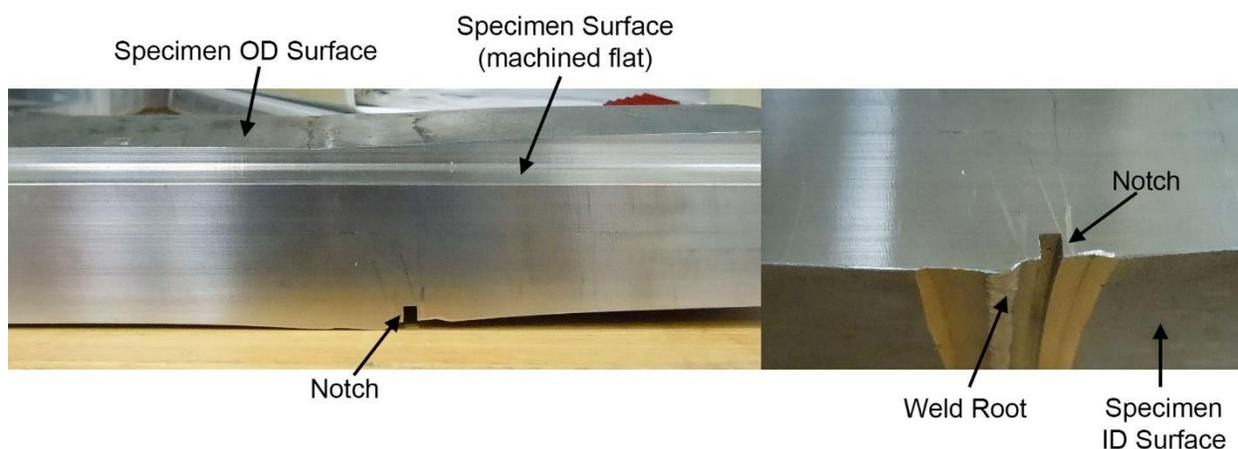
**Figure 4.2. Photograph of Specimen 2 with a saw-cut notch. *Left:* Side view of the specimen showing the machined flat top face. *Right:* Bottom of the specimen, showing the weld root and counterbore.**
