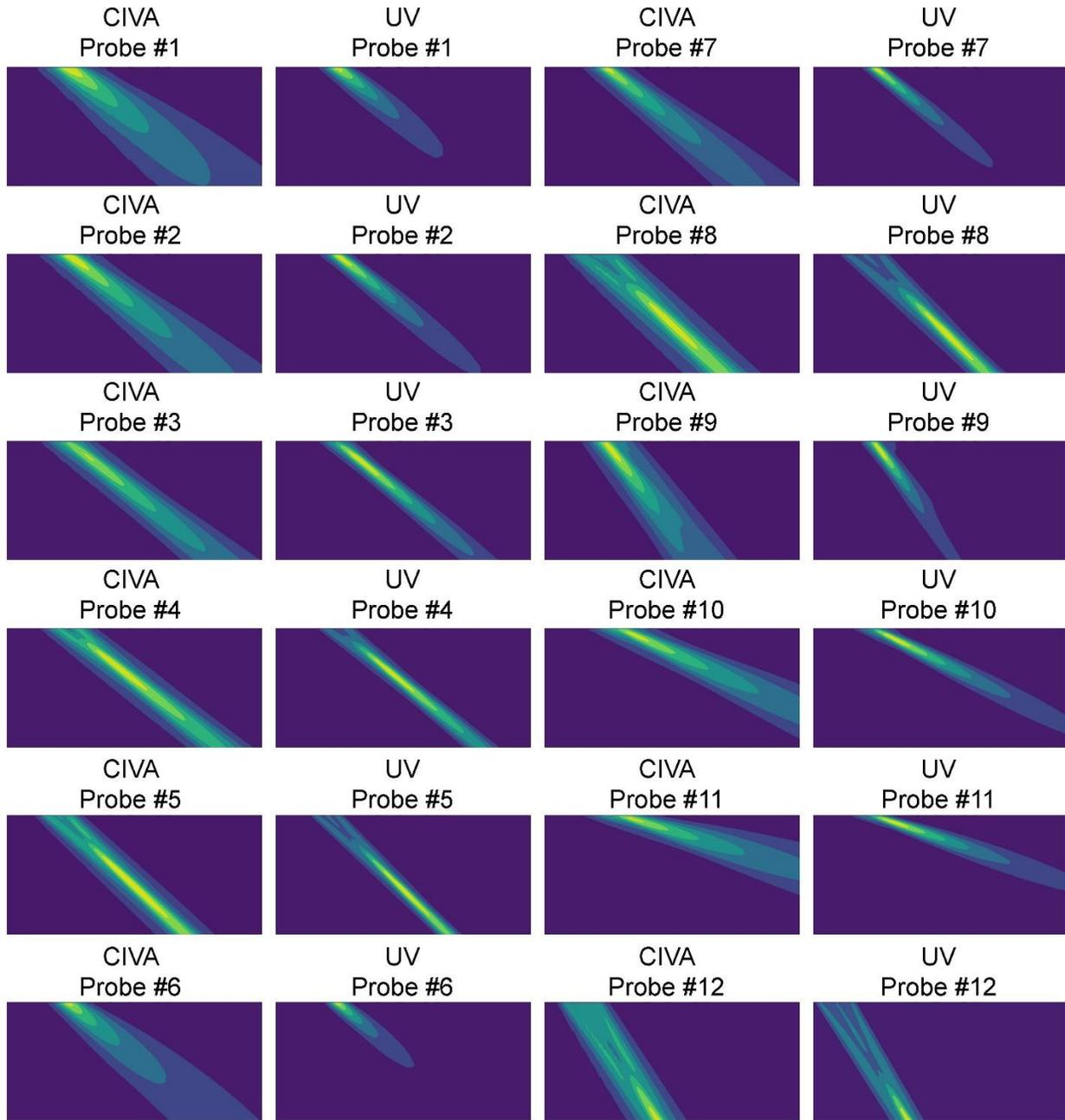
**Figure 3.1.** Beam simulations for the 12 shear wave probes using CIVA and UV. The specifications of the probes are indicated in the title of each beam as (frequency, diameter, beam angle, mode). The color map color range for each simulation shown is normalized relative to its own maximum amplitude.
