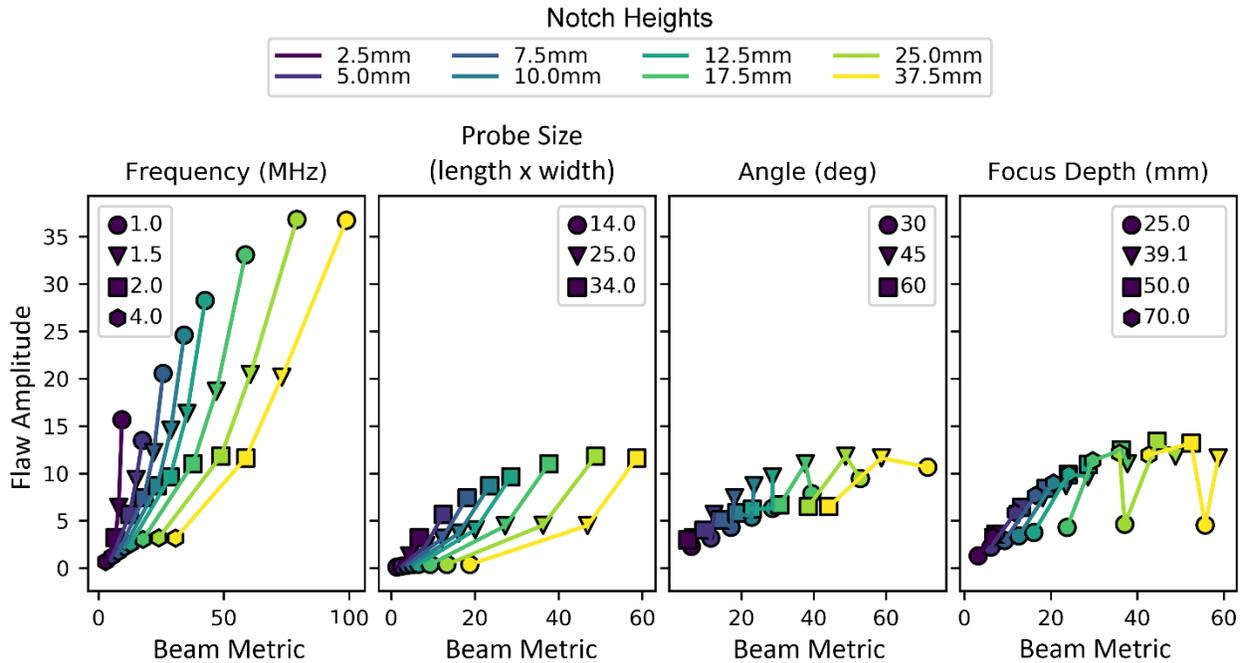
**Figure 5.6. Beam metric vs. flaw backscatter amplitude for transmit receive longitudinal probes and for eight different notch heights. One probe parameter was changed at a time from left to right: frequency, probe size (length x width), beam angle, and focal distance.**
