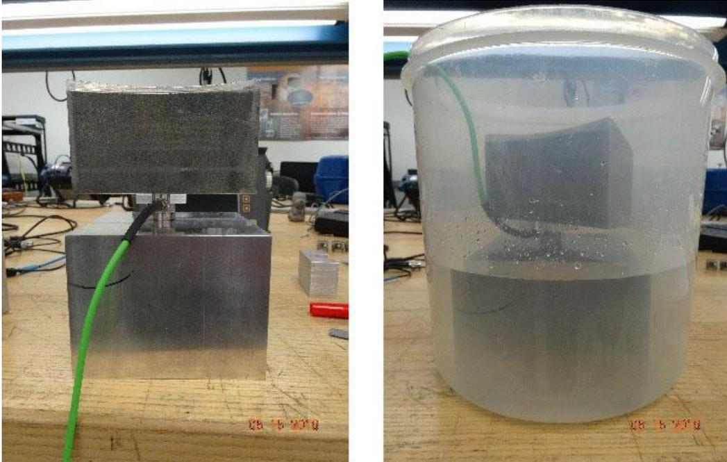
Figure 7.3. Contact configuration using 4.5 lb. weight for consistent coupling.
