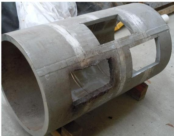
**Figure 4.1. Mockup 3C-022 from which the two specimen samples were cut for this work. Note that there are three cuts in this pipe, but only two were used.**
