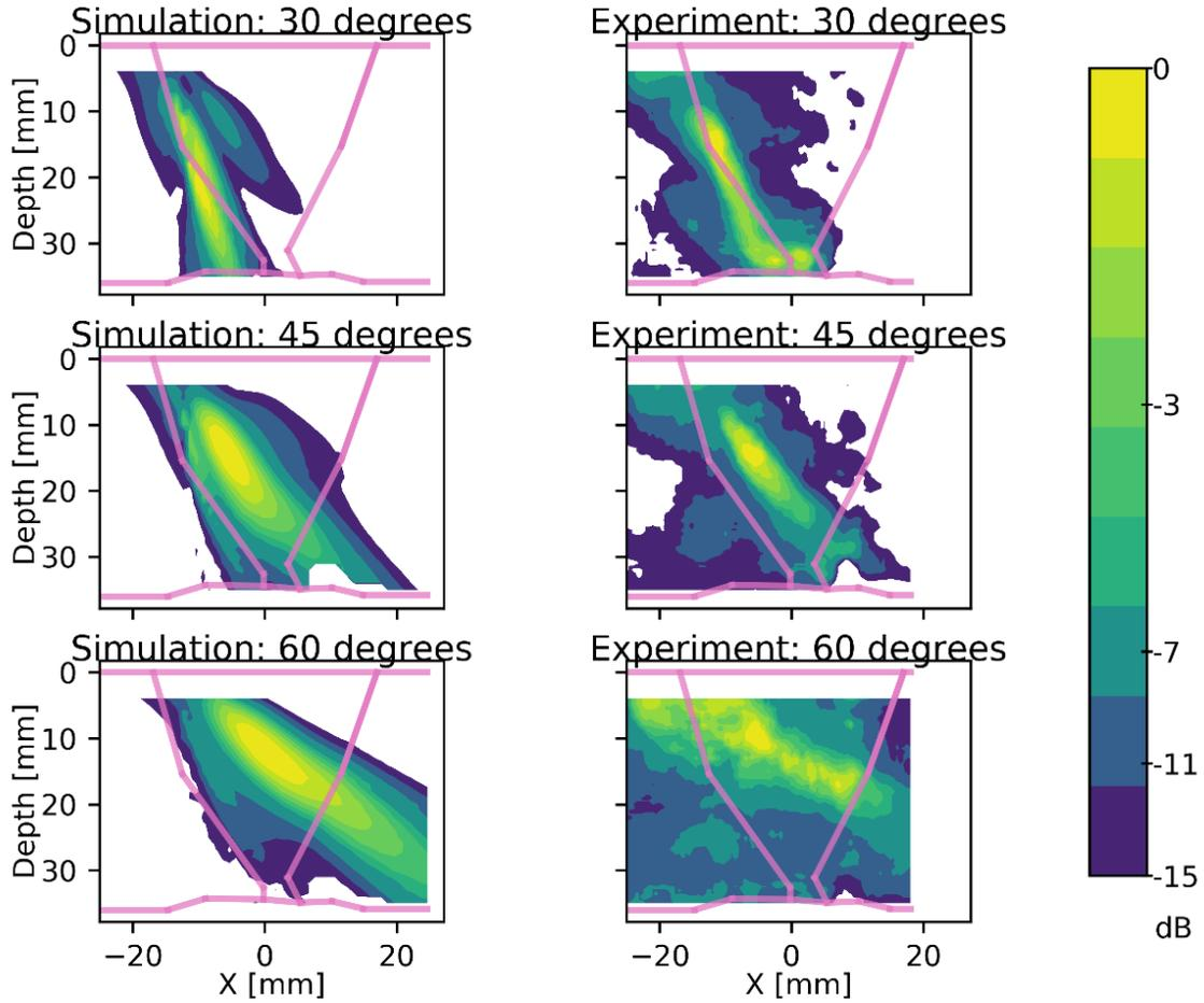
**Figure 4.10. Simulated and experimental sound beams using the phased-array probe at 30°, 45°, and 60° angles through Specimen 2. The weld root is located at X=0 mm. Each beam map is normalized to itself.**
