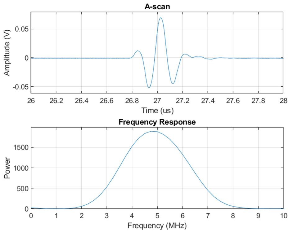
Figure 7.4. Representative transducer time-domain (*top*) and frequency-domain (*bottom*) results.
