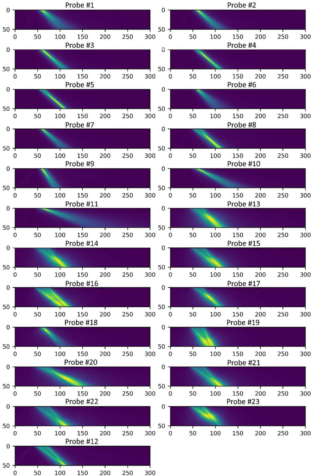
**Figure 5.2.** The cross-sectional beam simulations for all 23 probes. The color map ranges for each beam are independent. That is, each beam has its own color map normalized to span its independent minimum to maximum range.
