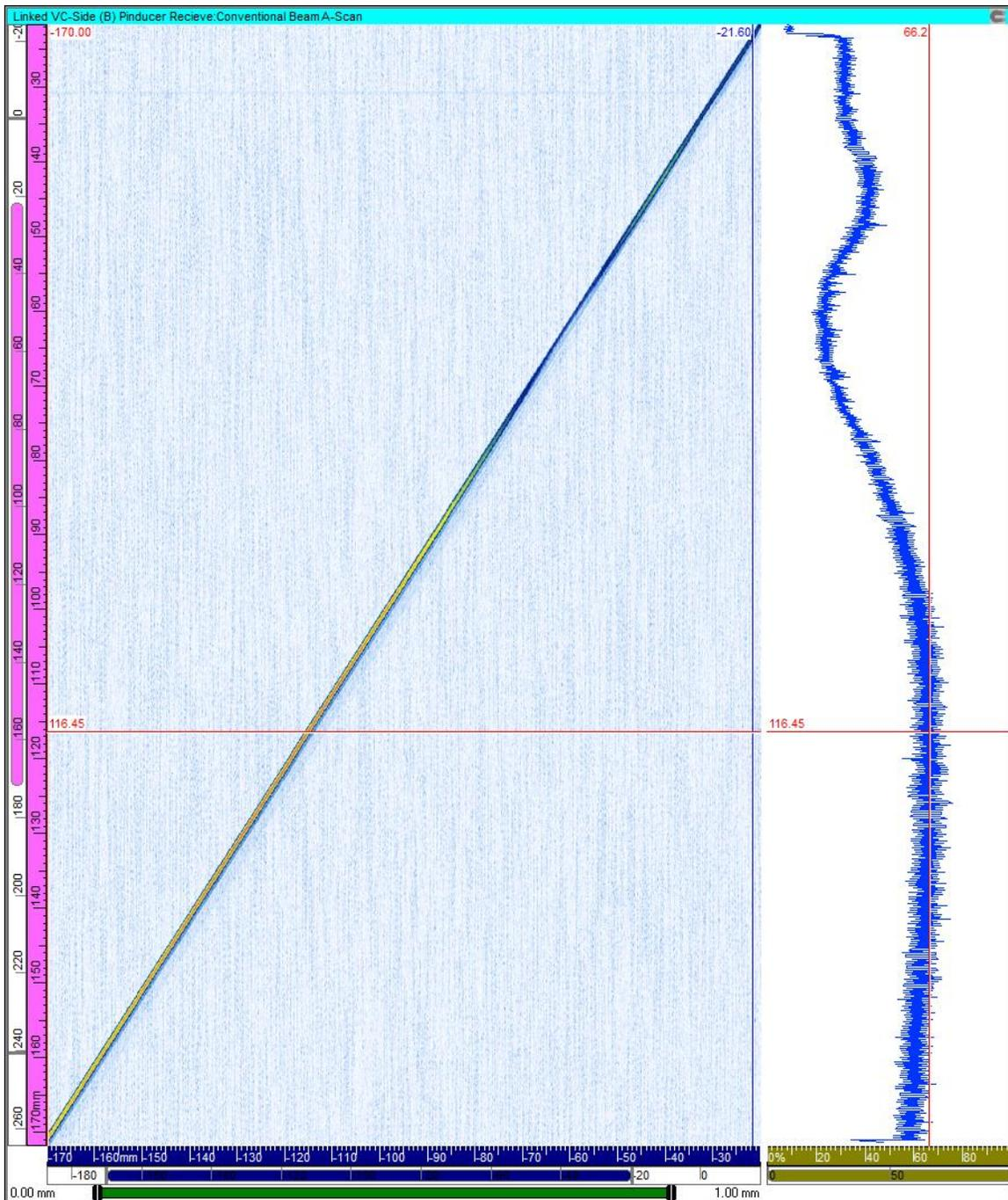
**Figure 7.12** UltraVision line profile data from Transducer #7 showing the raw line scan data (*left*) and the data profile (*right*). The horizontal red line indicates the approximate position of the signal maximum.
