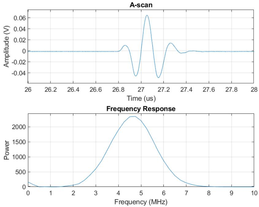
**Figure A.5. Time and frequency response for Transducer #4.**
