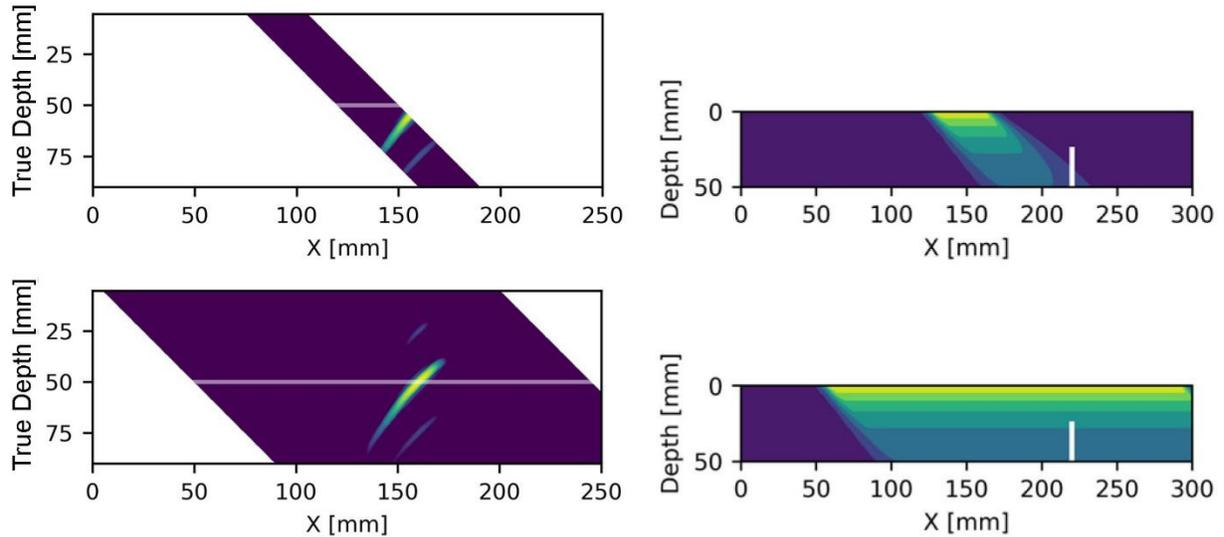
**Figure 5.12. Example of partial access simulations as seen by the B-scan (*top left*), and the total beam incident onto flaw (*top right*). The bottom panels show the full access scenario for reference. In the B-scans, the horizontal line indicates the specimen backwall. In the beam plots, the vertical line shows the flaw location and size (through-wall depth).**
