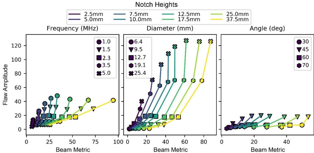
**Figure 5.5. Beam metric vs. flaw backscatter amplitude for shear wave probe and for eight different notch heights. One probe parameter was changed at a time: frequency (*left*), diameter (*center*), and beam angle (*right*).**
