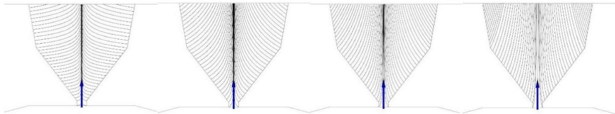
**Figure 2.4. Different weld morphologies controlled by the value of  $T$ . From left to right,  $T = 0.1, 0.5, 1, 2$ .**
