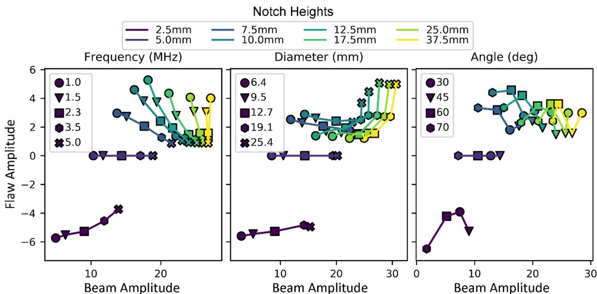
**Figure 5.8. Normalized beam metric vs. normalized flaw backscatter amplitude for the shear wave probes and for eight different notch heights. One probe parameter was changed at a time—frequency (*left*), diameter (*center*), and beam angle (*right*).**
