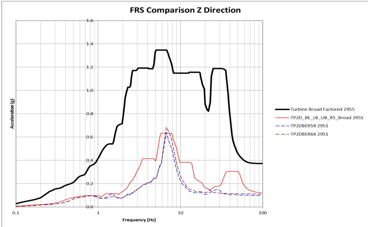
Figure F.2-2. TPNP TB 1<sup>st</sup> Bay BE Sensitivity FRS Comparison and FRS Envelope in Z-Direction – Node 2951
