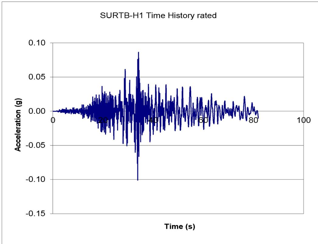
Figure F.1-9. TPNP Updated TB 1st Bay Seismic Input H1 in X-Direction (Scaled to 0.1g) – EI. +25.5' – Reference 12
