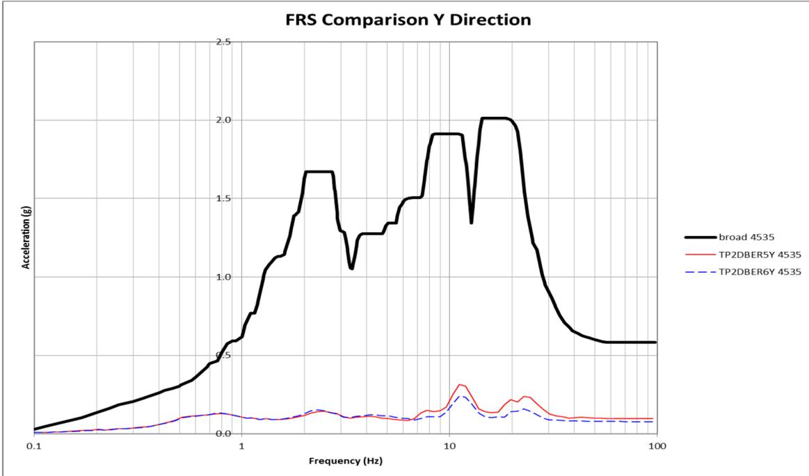
Figure F.2-21. TPNP 2D NI BE Sensitivity FRS Comparison, Y Direction – Node 4535 (El. 134.25 ft)
