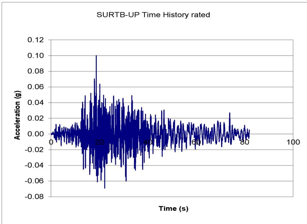
Figure F.1-10. TPNP Updated TB 1st Bay Seismic Input UP in Z-Direction (Scaled to 0.1g) – EI. +25.5 – Reference 12
