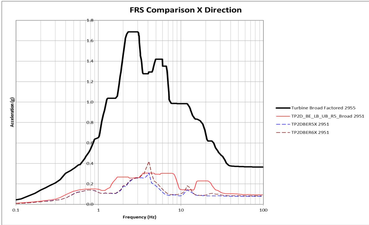
Figure F.2-1. TPNP TB 1<sup>st</sup> Bay BE Sensitivity FRS Comparison and FRS Envelope in X-Direction – Node 2951
