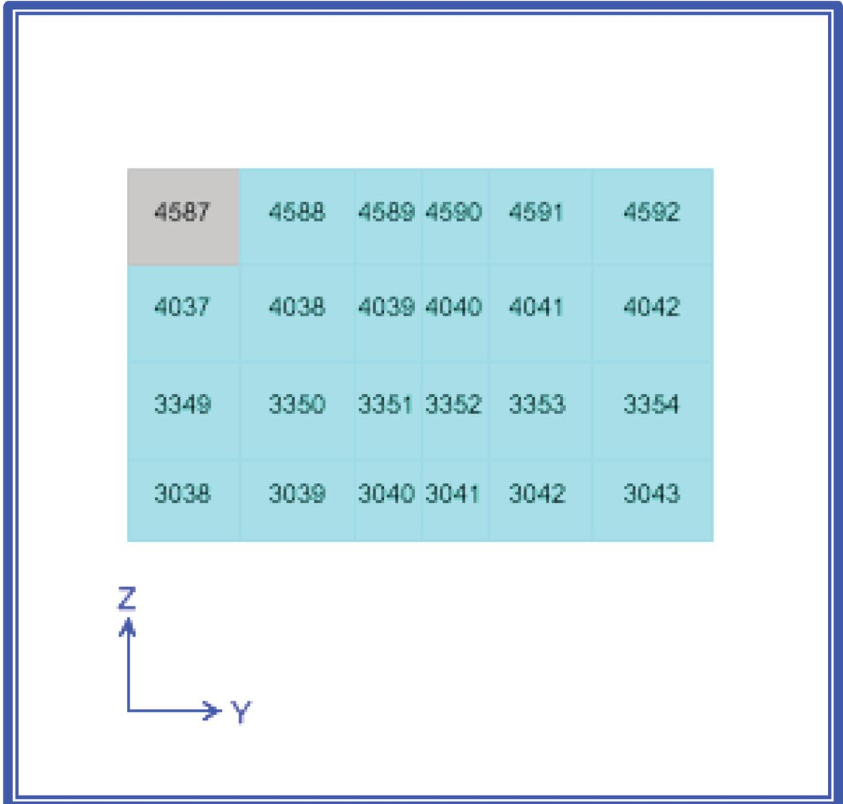
**Figure 4-12. Single Elements from Pool Gate Support Wall with Insufficient Thermal T0 Strain Capacity for Load Combination 9-6 in X Direction.**
