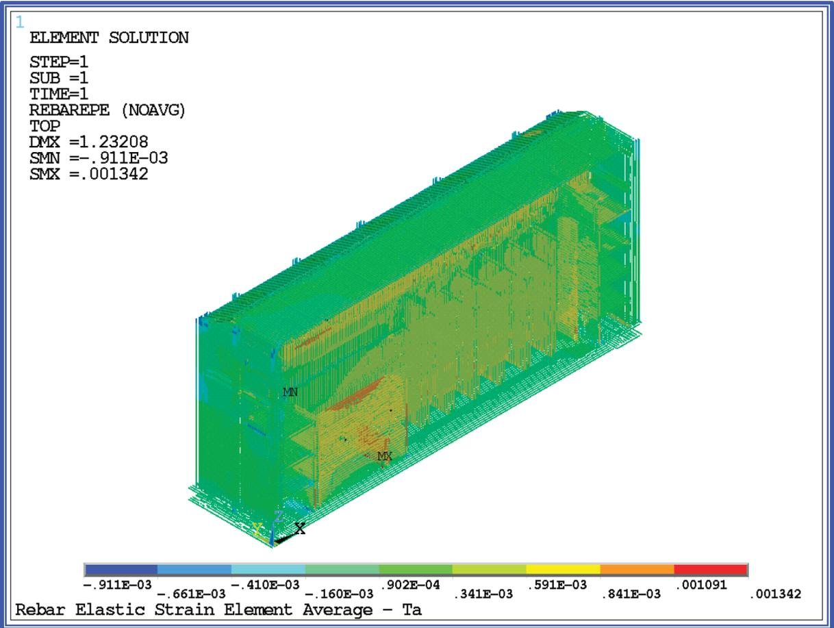
Figure 2-7. RXB Rebar Elastic Strain - Ta - All Sections (View 1).
