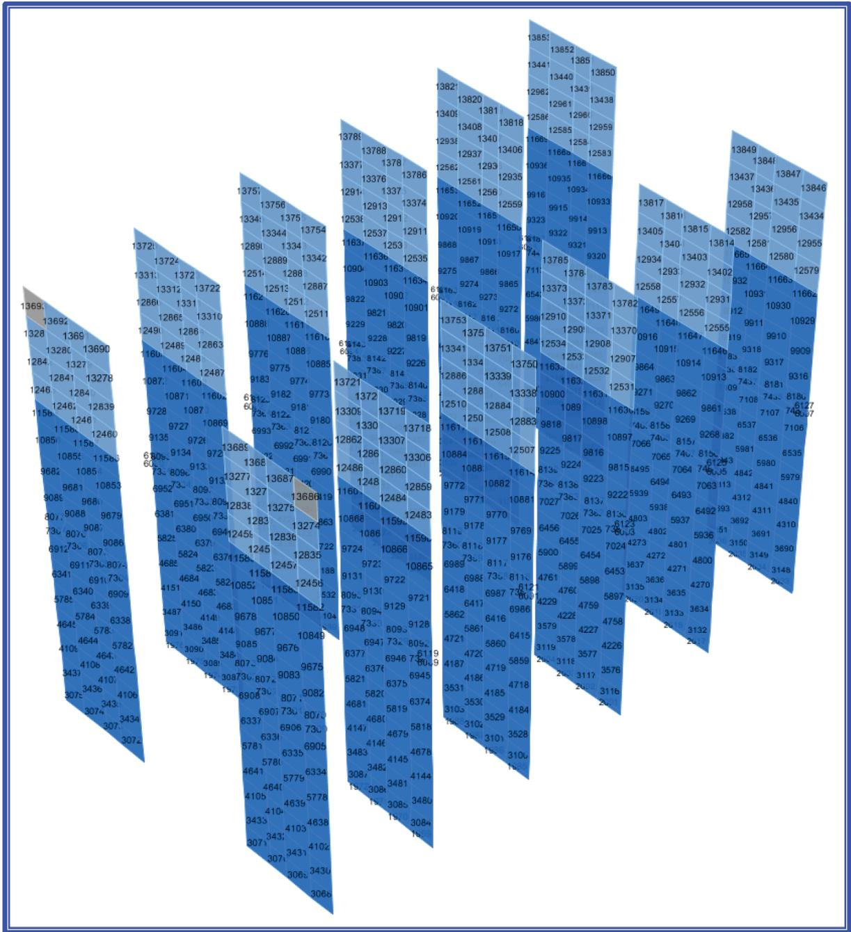
**Figure 4-18. Single Elements from NPM Support Walls with Insufficient Thermal  $T_a+P_a$  Strain Capacity for Load Combination 9-9 in X Direction.**
