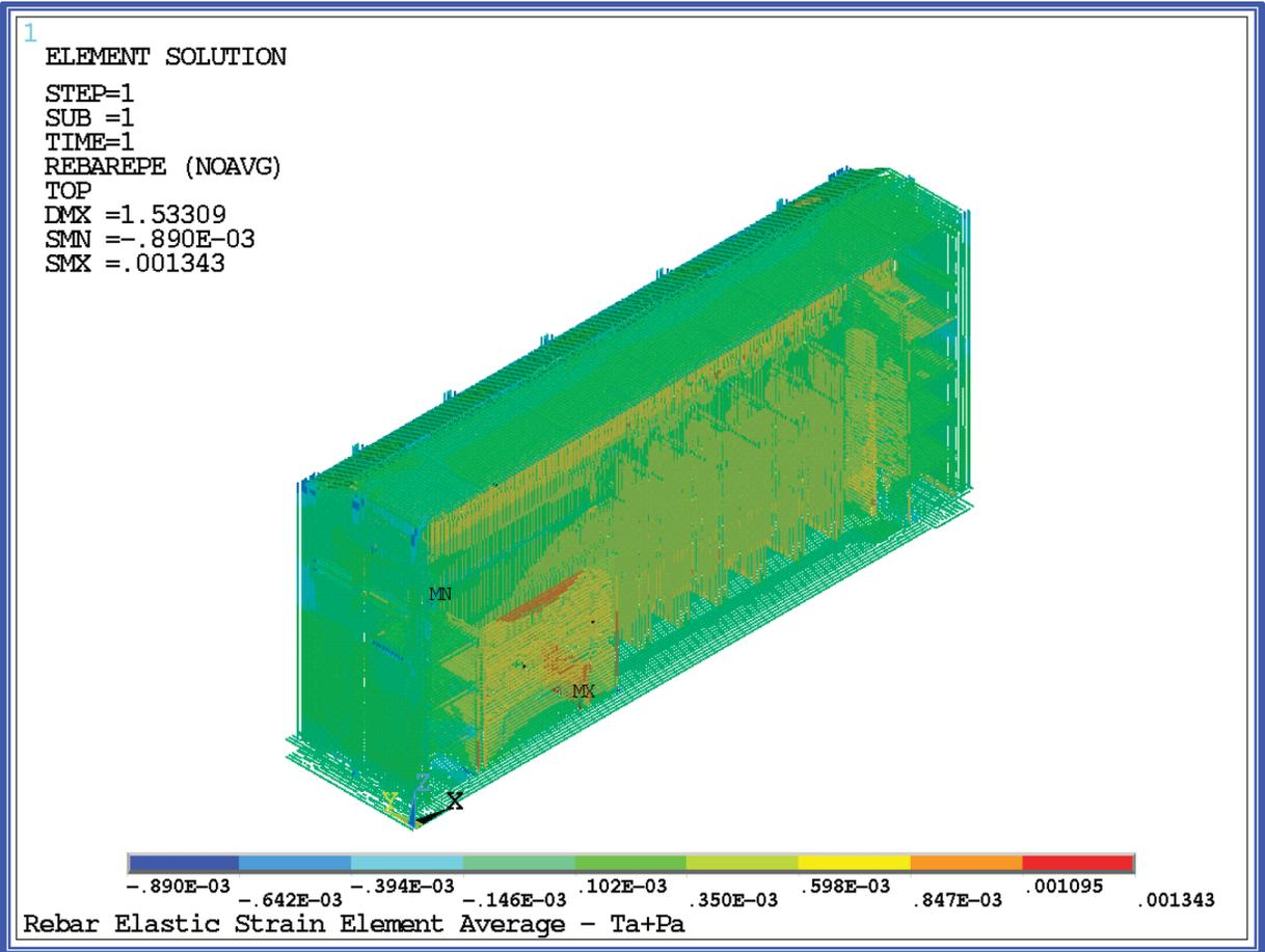
Figure 2-9. RXB Rebar Elastic Strain - Ta+Pa - All Sections (View 1).
