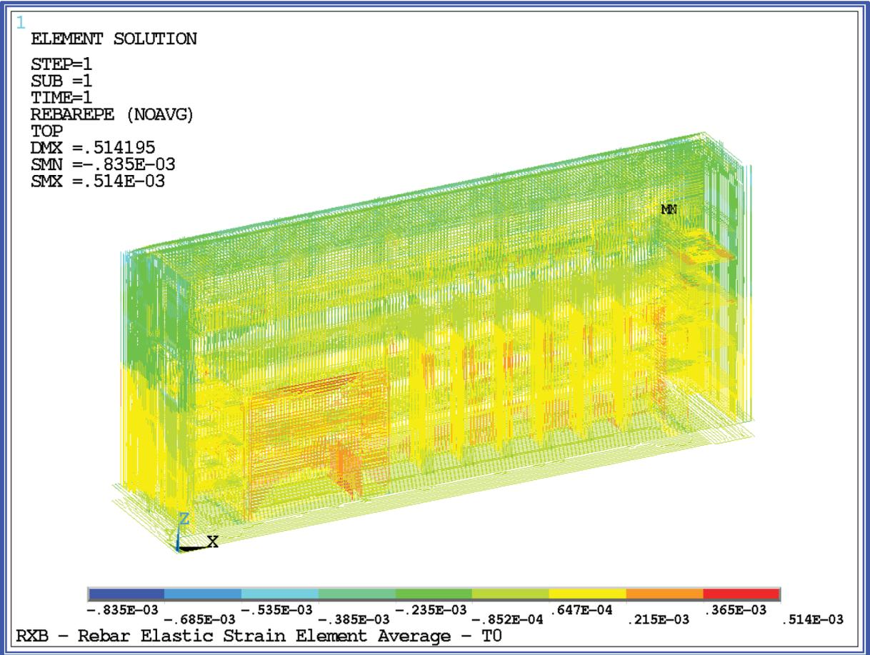
**Figure 2-3. RXB Rebar Elastic Strain - T0 - All Sections (View 1).**
