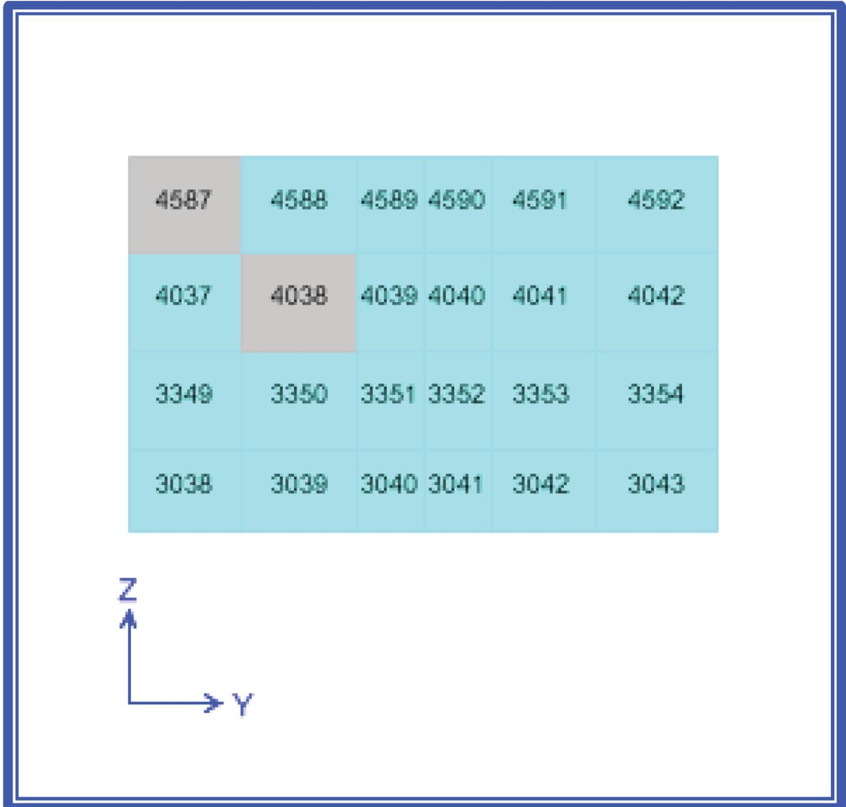
**Figure 4-15. Single Elements from Pool Gate Support Wall with Insufficient Thermal Ta+Pa Strain Capacity for Load Combination 9-9 in Y Direction.**
