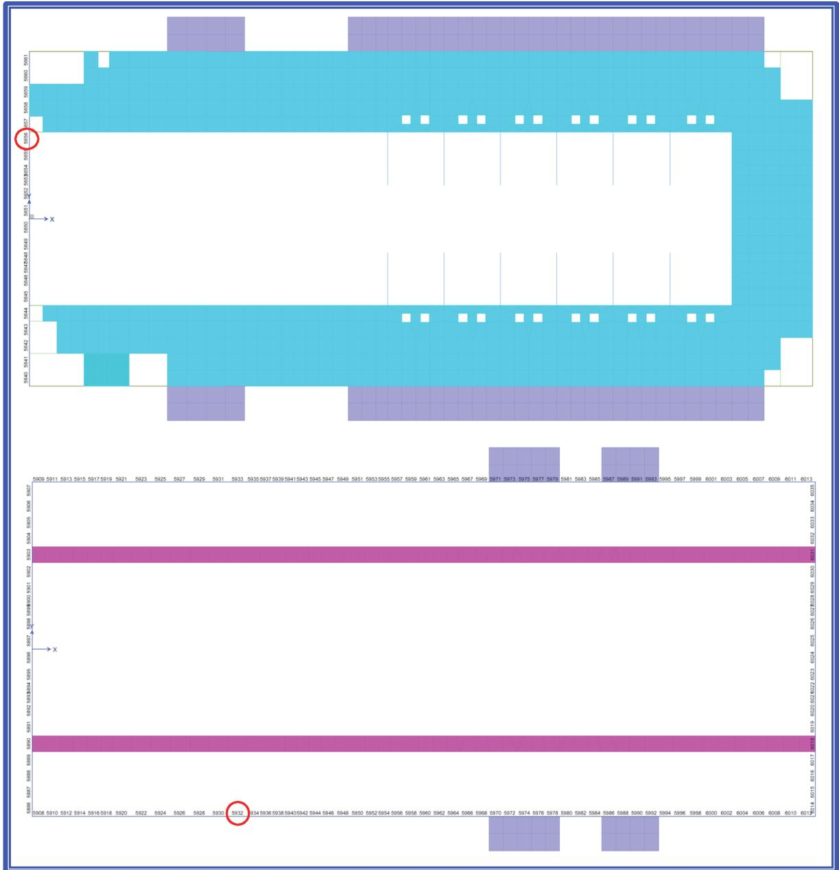
**Figure 4-23. Single Elements from Buttress at TOC EL 126'-0" and 145'-0" with Insufficient Thermal  $T_a+P_a$  Strain Capacity for Load Combination 9-9.**
