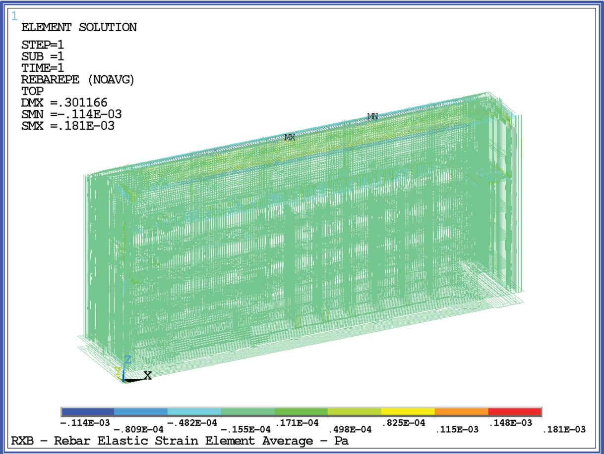
Figure 2-5. RXB Rebar Elastic Strain - Pa - All Sections (View 1).
