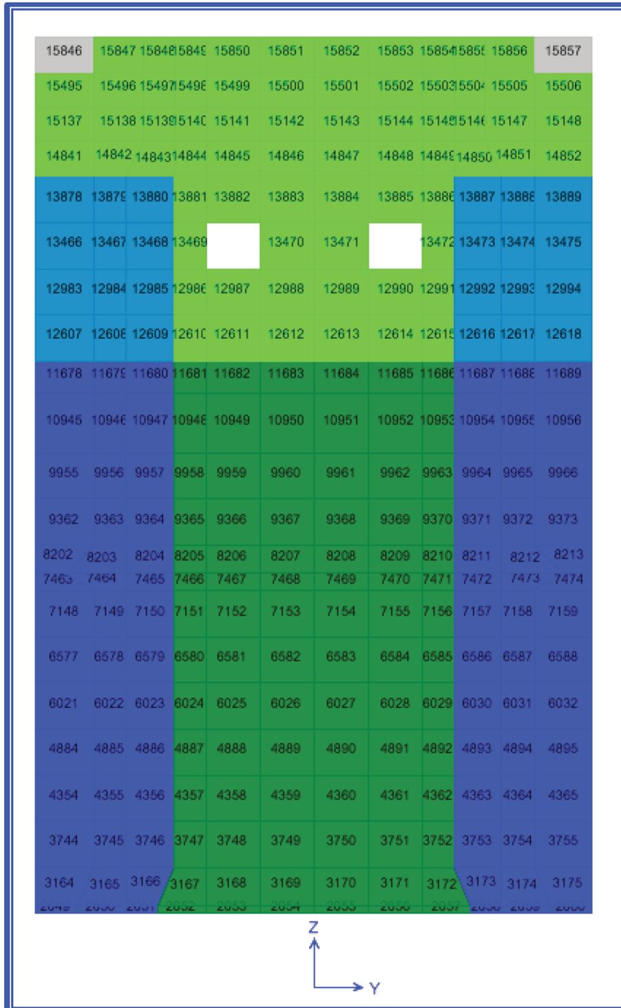
Figure 4-6. Single Elements from Pool Wall - East (Grid Line 6) with Insufficient Thermal T0 Strain Capacity for Load Combination 9-6 in X Direction.
