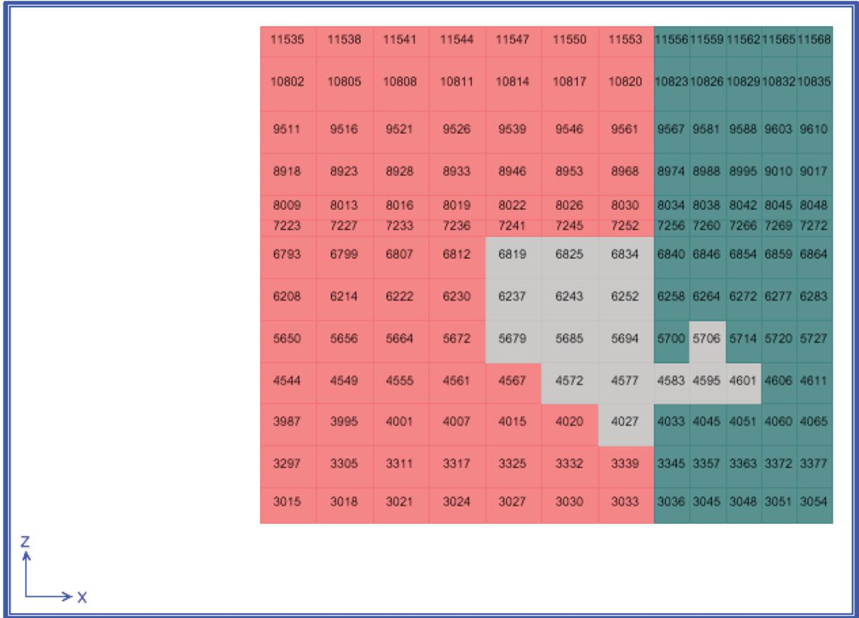
**Figure 4-11. Single Elements from Pool Wall - Middle (Grid Line C) with Insufficient Thermal Ta+Pa Strain Capacity for Load Combination 9-9 in Y Direction.**
