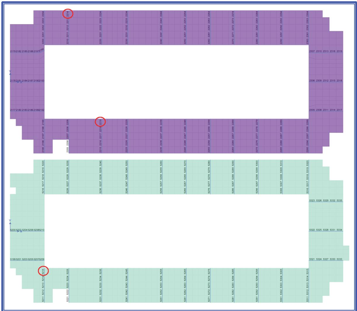
**Figure 4-24. Single Elements from T-Beams at TOC EL 50'-0", 75'-0", and 100'-0" with Insufficient Thermal  $T_a+P_a$  Strain Capacity for Load Combination 9-9.**
