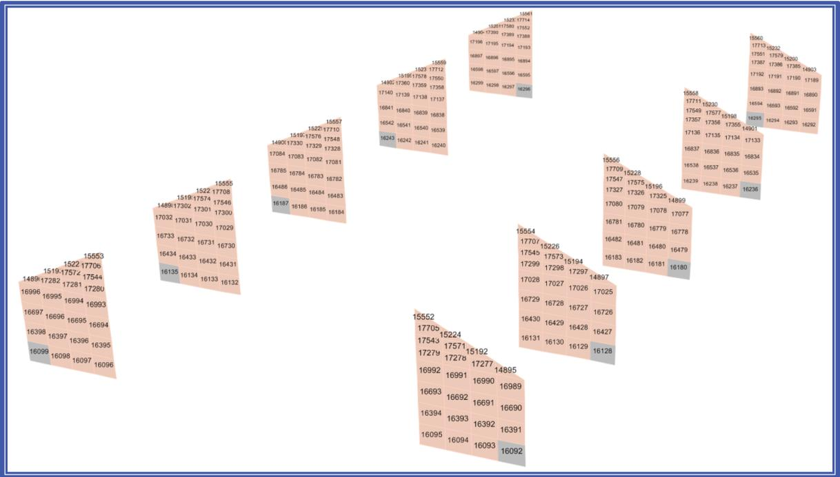
**Figure 4-17. Single Elements from Roof Support Stiffeners with Insufficient Thermal  $T_a+P_a$  Strain Capacity for Load Combination 9-9 in X Direction.**
