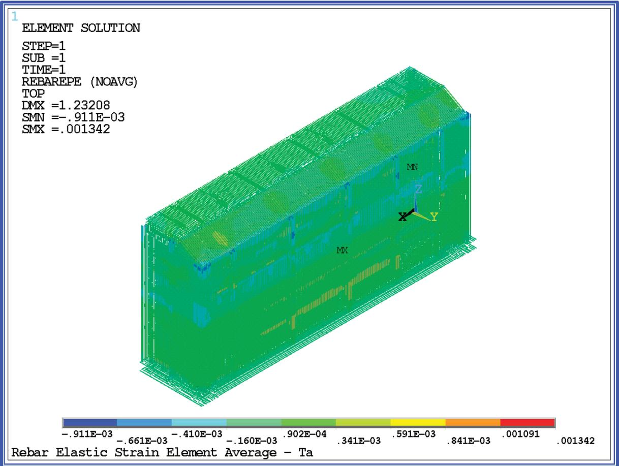
Figure 2-8. RXB Rebar Elastic Strain - Ta - All Sections (View 2).
