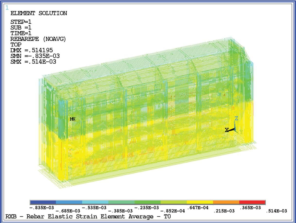
**Figure 2-4. RXB Rebar Elastic Strain - T0 - All Sections (View 2).**
