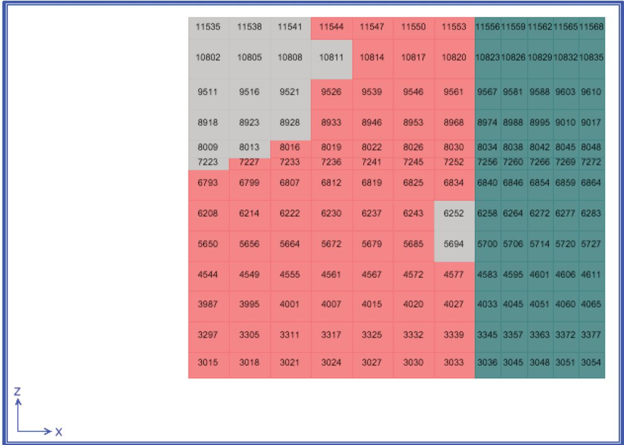
**Figure 4-10. Single Elements from Pool Wall - Middle (Grid Line C) with Insufficient Thermal Ta+Pa Strain Capacity for Load Combination 9-9 in X Direction.**
