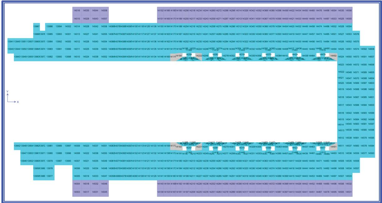
**Figure 4-19. Single Elements from Major Floor Slabs with Insufficient Thermal T0 Strain Capacity for Load Combination 9-6 in Y Direction.**
