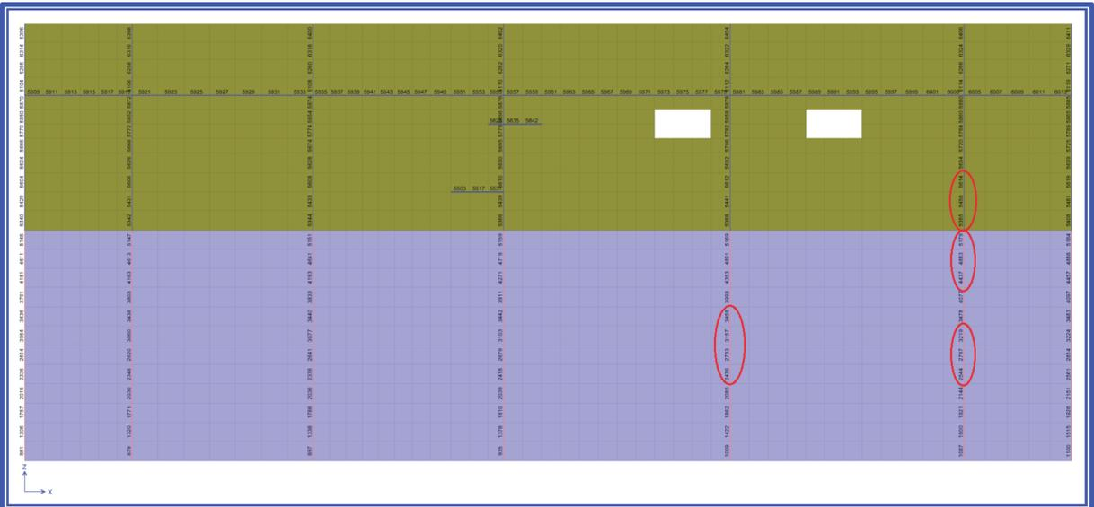
**Figure 4-22. Single Elements from Pilasters at Grid Line A with Insufficient Thermal  $T_a + P_a$  Strain Capacity for Load Combination 9-9.**
