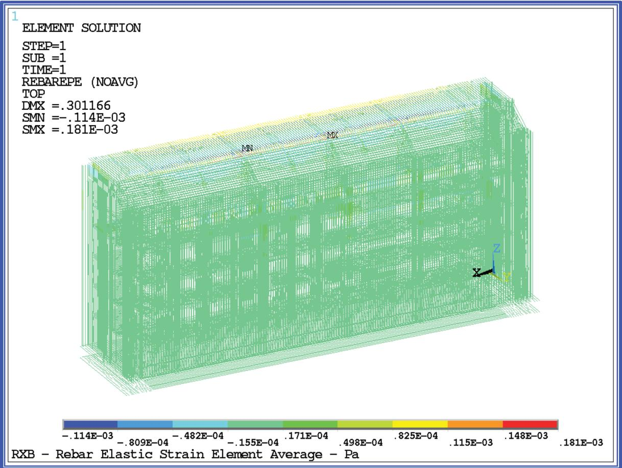
Figure 2-6. RXB Rebar Elastic Strain - Pa - All Sections (View 2).
