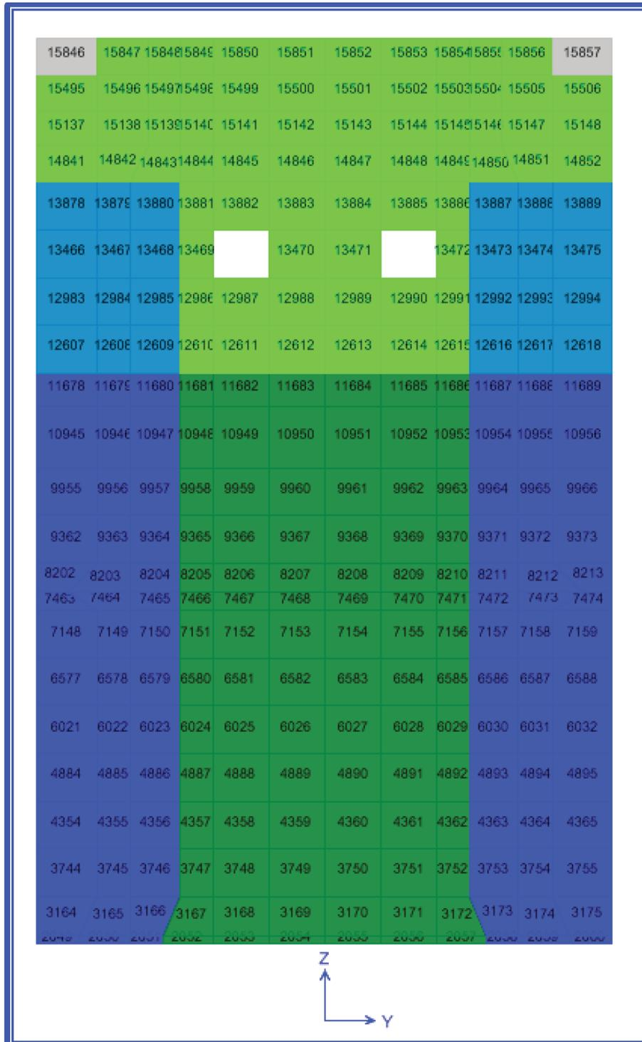
**Figure 4-7. Single Elements from Pool Wall - East (Grid Line 6) with Insufficient Thermal Ta+Pa Strain Capacity for Load Combination 9-9 in X Direction.**
