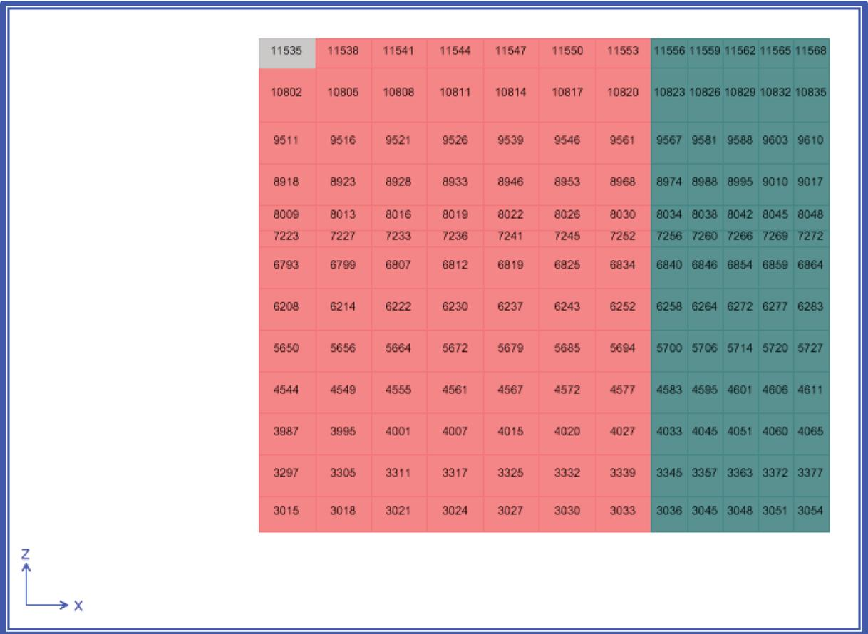
**Figure 4-1. Single Elements from Pool Wall - Middle (Grid Line C) Exceeding Allowable Concrete Strain in X Direction.**
