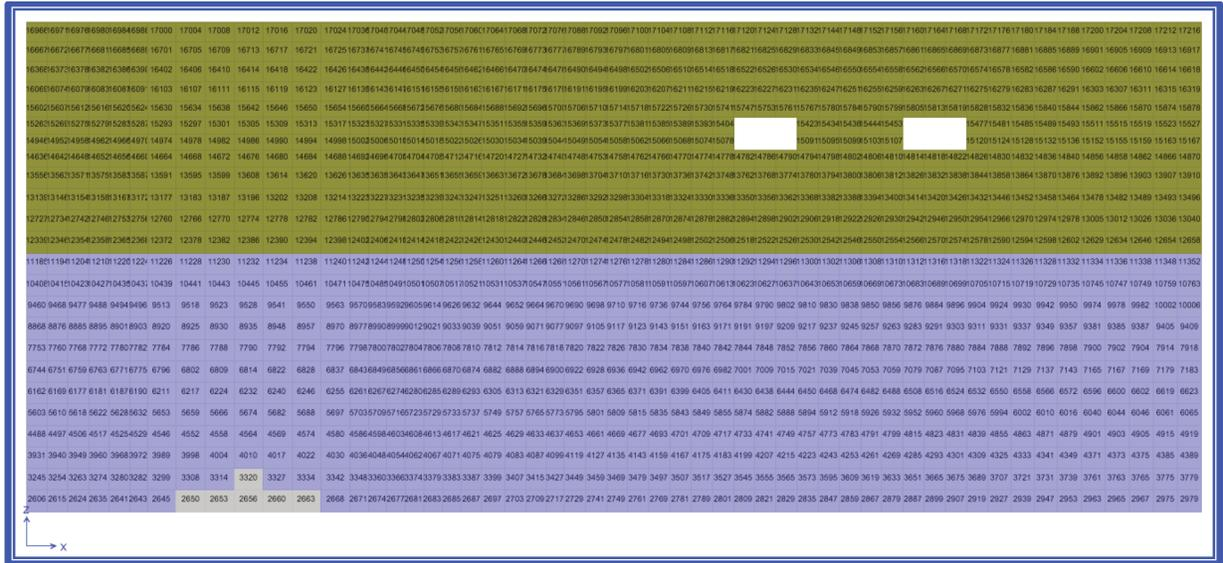
**Figure 4-3. Single Elements from Outer Wall - North (Grid Line A) with Insufficient Thermal Ta+Pa Strain Capacity for Load Combination 9-9 in Y Direction.**
