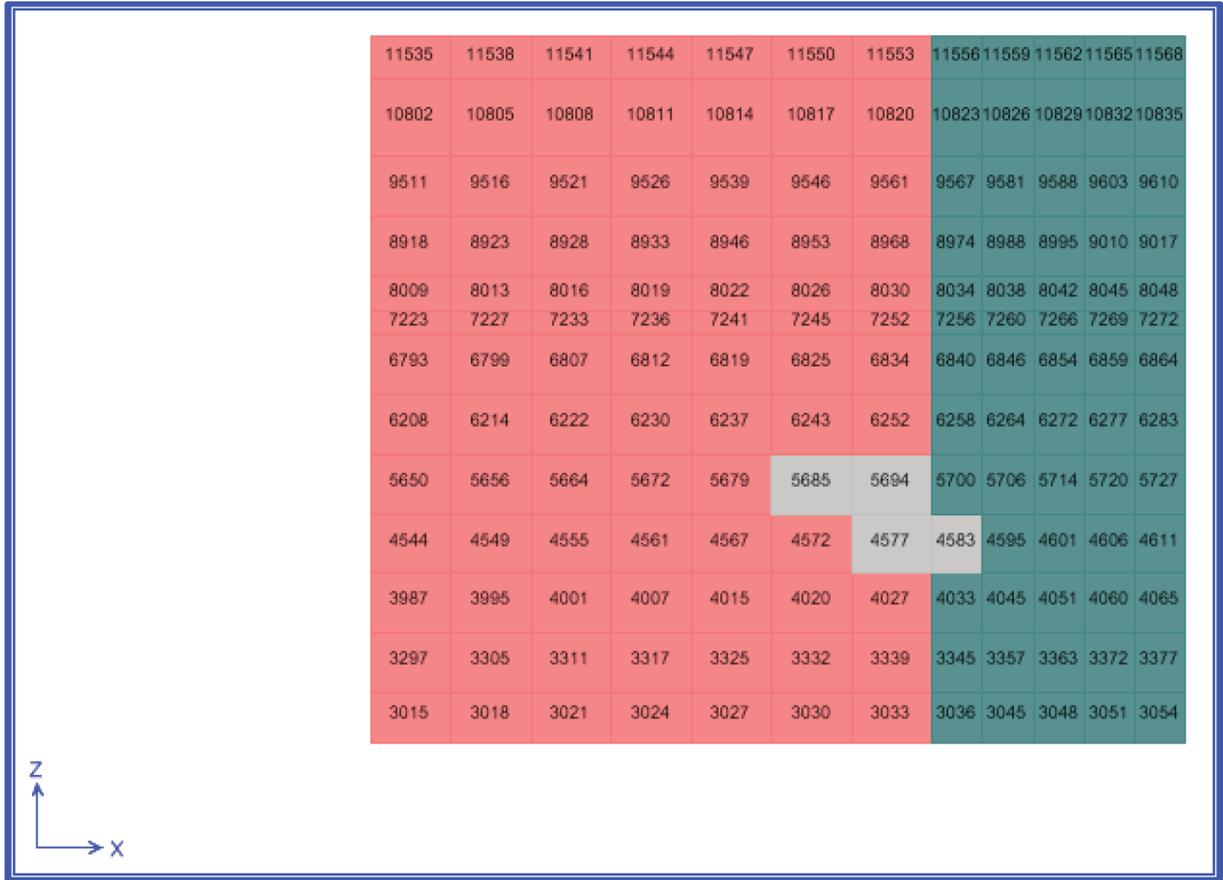
**Figure 4-9. Single Elements from Pool Wall - Middle (Grid Line C) with Insufficient Thermal T0 Strain Capacity for Load Combination 9-6 in Y Direction.**
