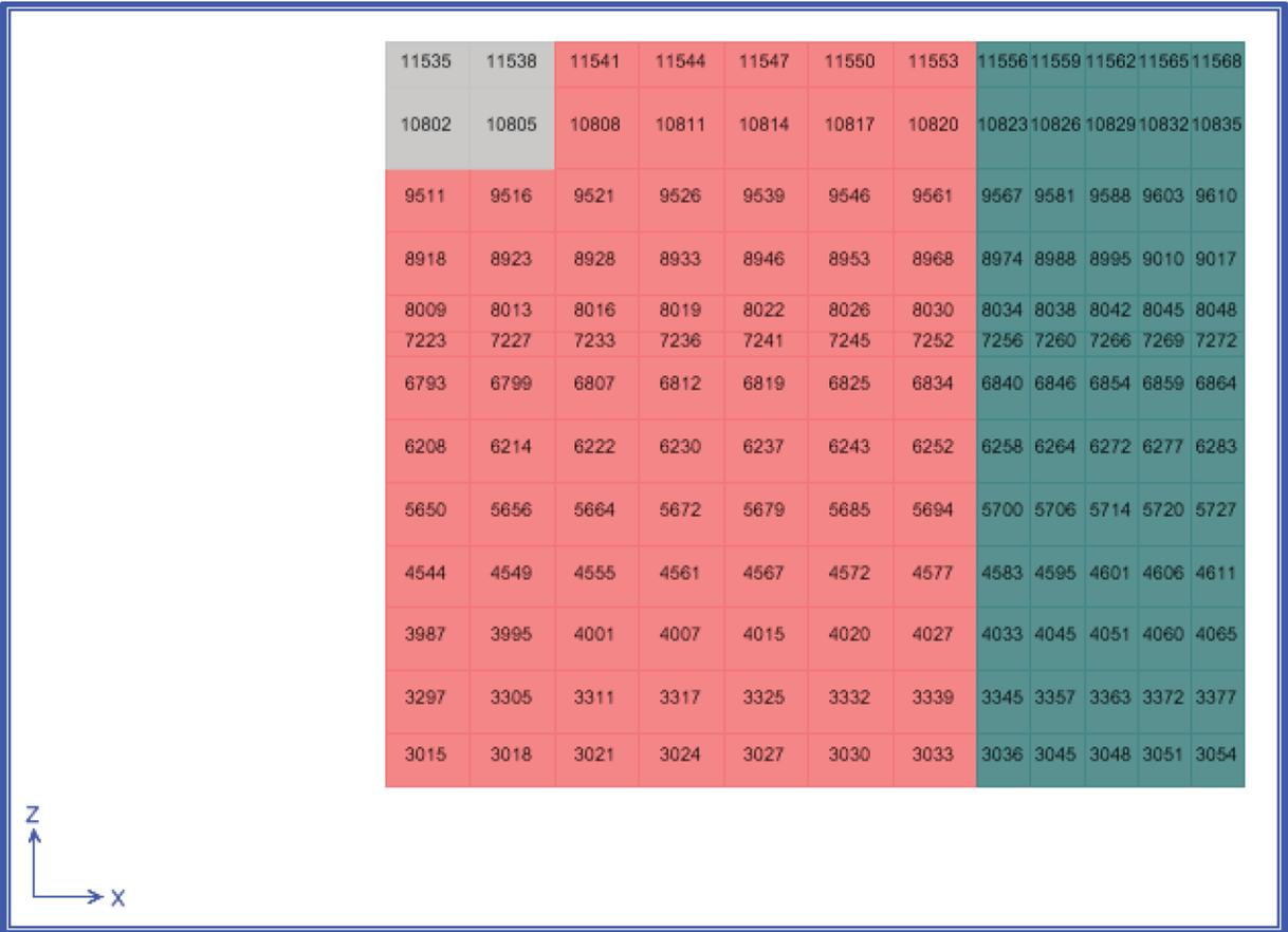
**Figure 4-8. Single Elements from Pool Wall - Middle (Grid Line C) with Insufficient Thermal T0 Strain Capacity for Load Combination 9-6 in X Direction.**
