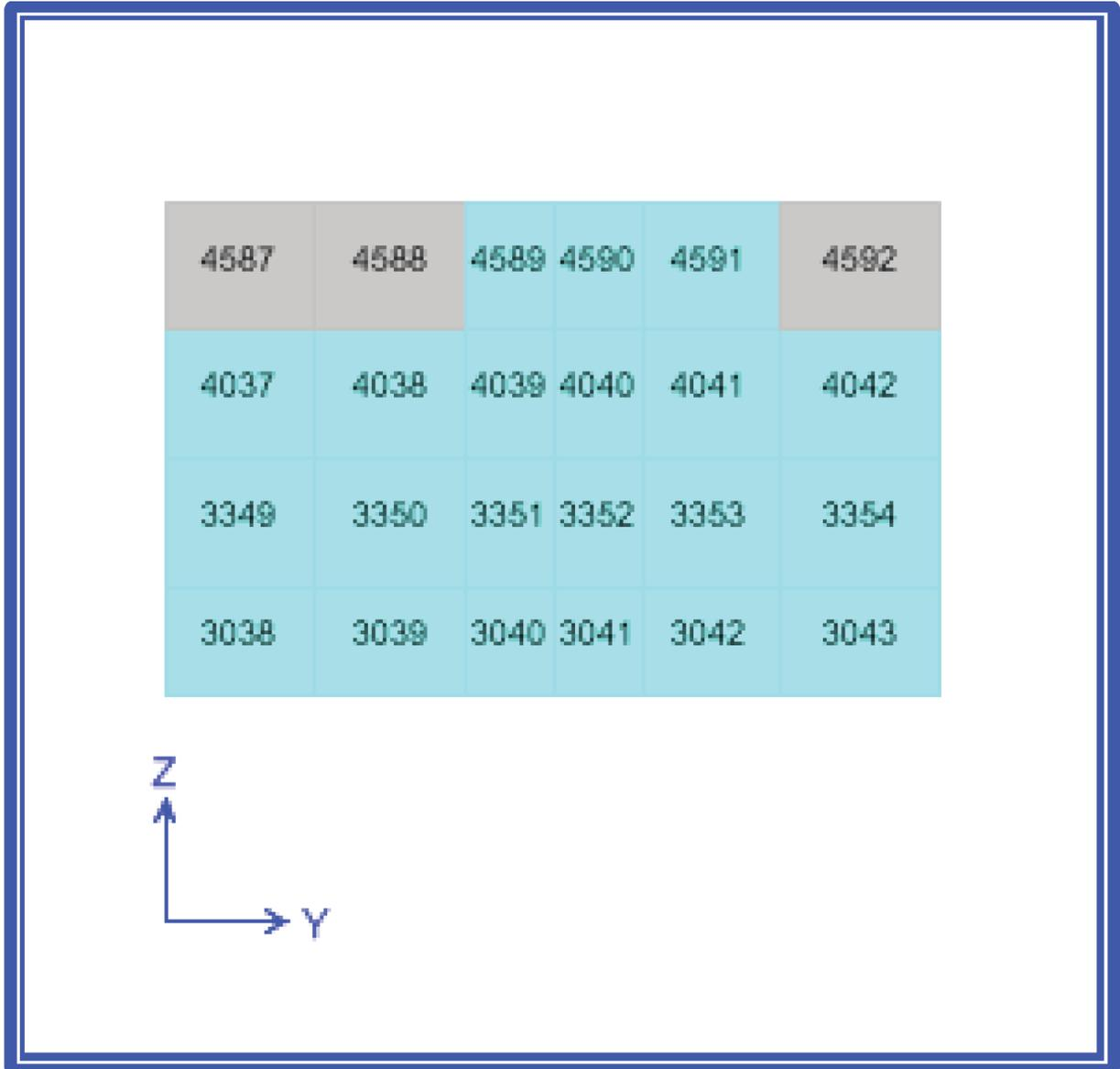
**Figure 4-14. Single Elements from Pool Gate Support Wall with Insufficient Thermal Ta+Pa Strain Capacity for Load Combination 9-9 in X Direction.**
