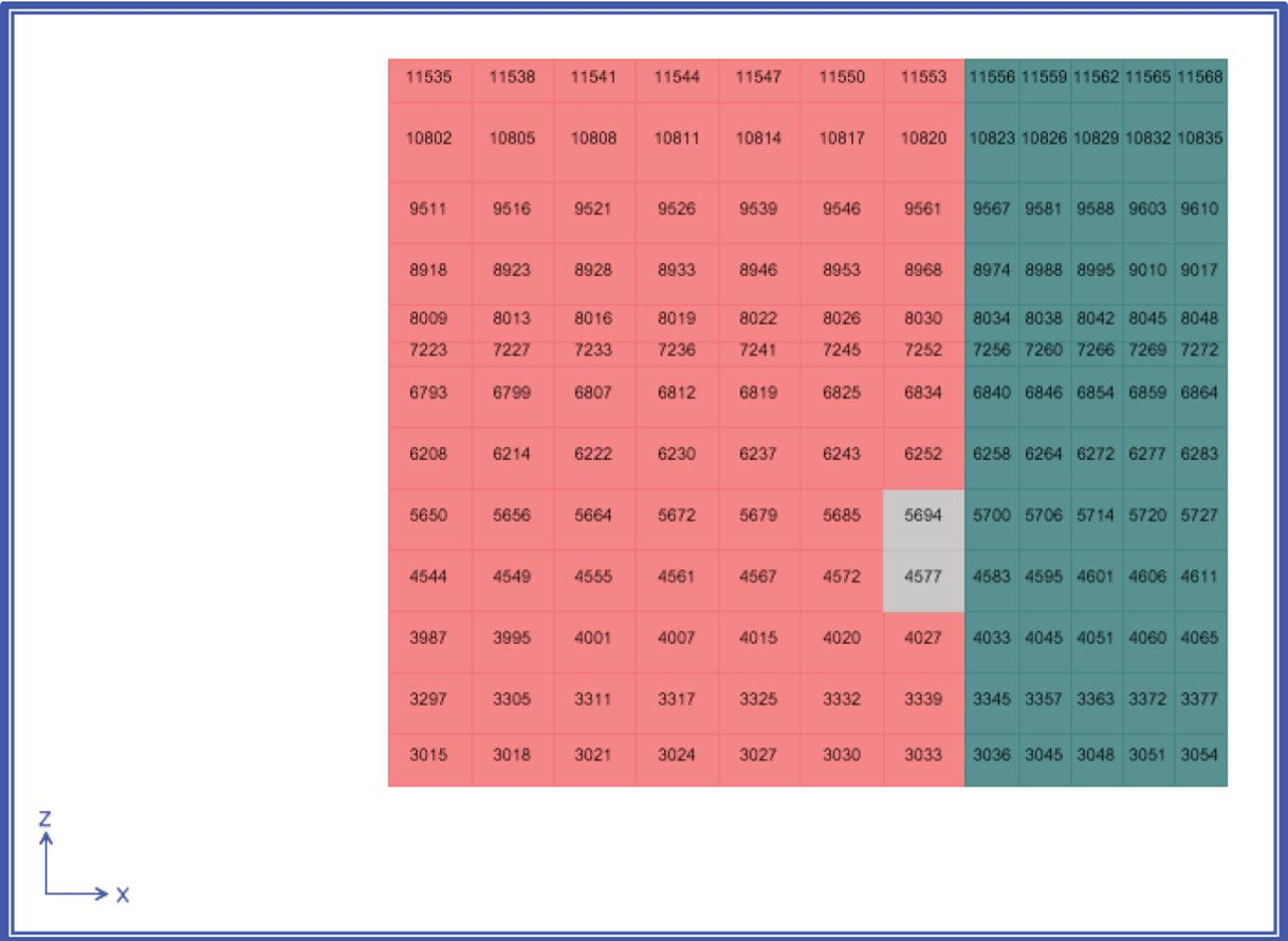
**Figure 4-2. Single Elements from Pool Wall - Middle (Grid Line C) Exceeding Allowable Concrete Strain in Y Direction.**
