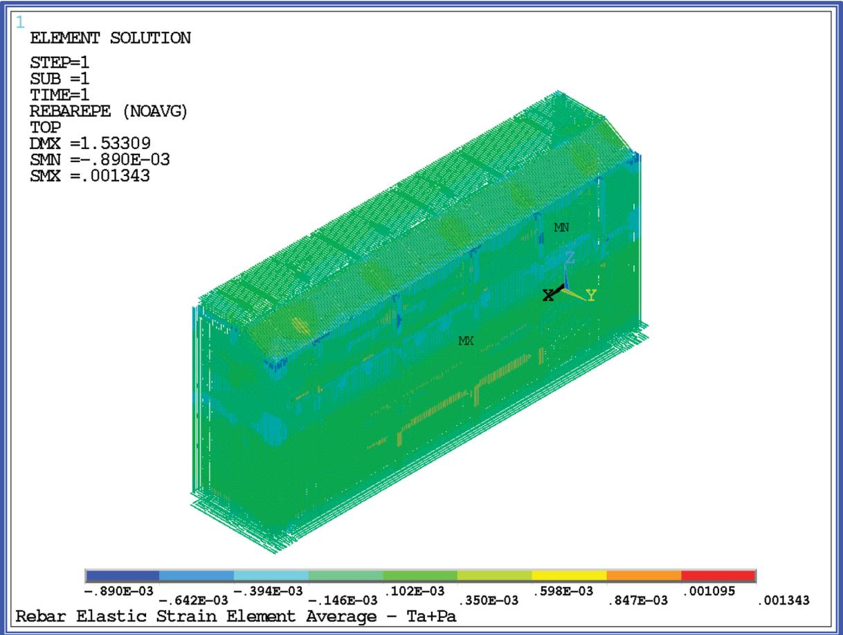
Figure 2-10. RXB Rebar Elastic Strain - Ta+Pa - All Sections (View 2).
