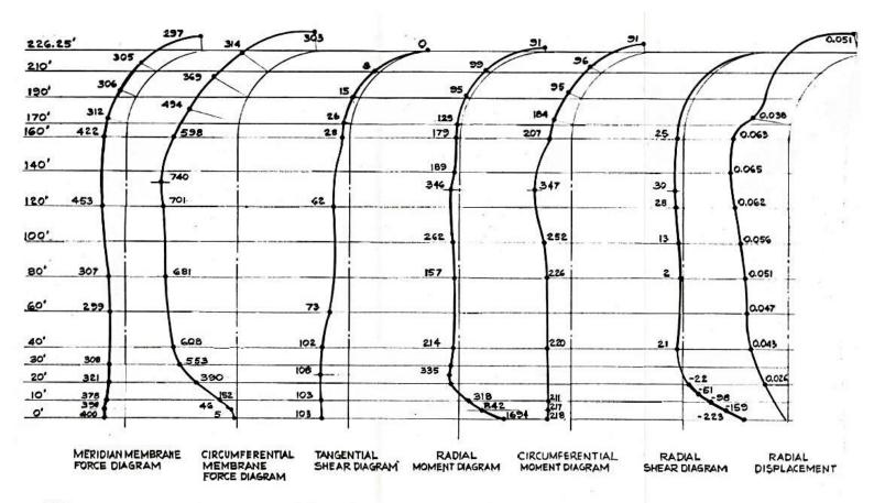
UNITS: FORCE IN KIPS, MOMENT IN FT — KIP, DISPLACEMENT IN FT. MEMBRANE FORCE SHOWN: TENSION IS POSITIVE
