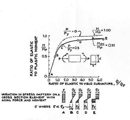
MOMENT-CURVATURE RELATIONSHIP FOR RECTANGULAR SECTION WITH AXIAL FORCE AND MOMENT ADAPTED FROM REF. 3. 8. 1-50
