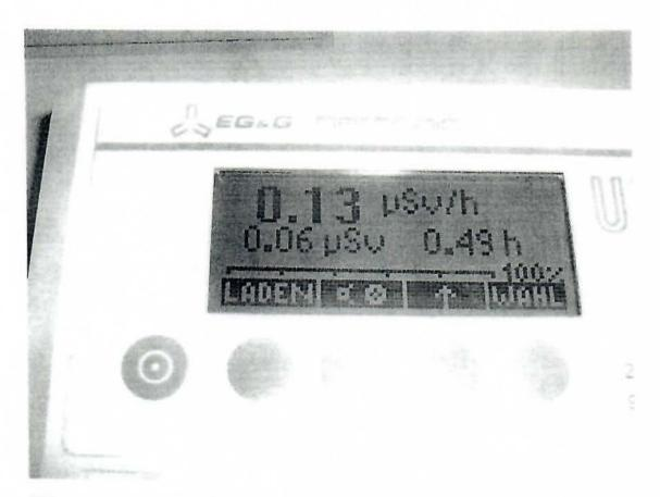
With arc tube in a distance of 1 cm same measurement was done (see picture). In order to increase the sensitivity we filled this arc-tube with 800 mbar which is at least 20 times more than usual. In addition we omit the absorber but measurements were done in air.
