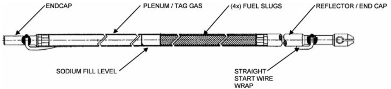
**Figure 3-3 PRISM Fuel Rod [3-10]**
