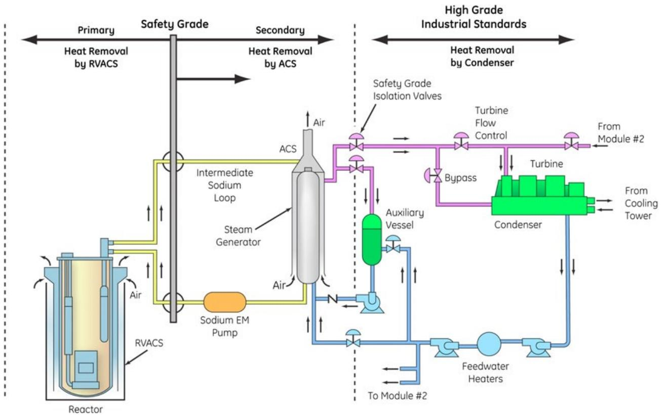
Figure 3-1 PRISM Nuclear Steam Supply System [3-10]
