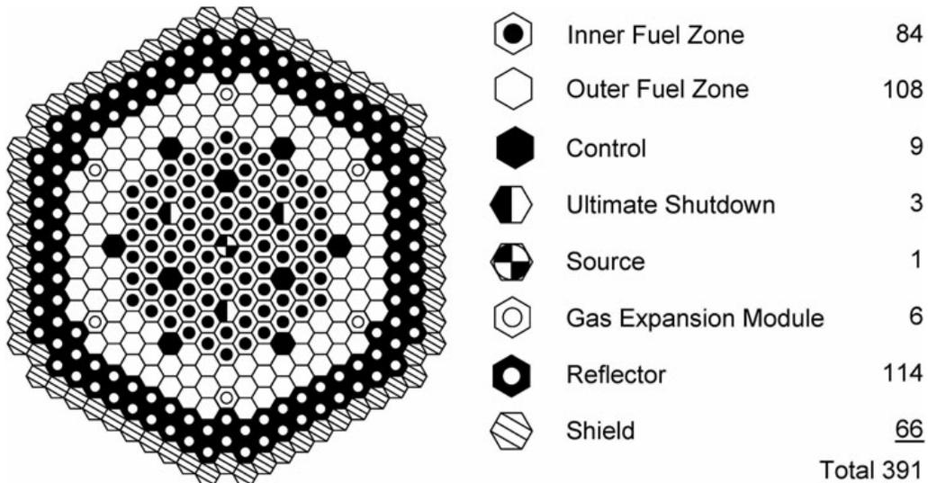
Figure 3-2 Fuel Assembly Layout for UNF Recycle Core [3-10]
