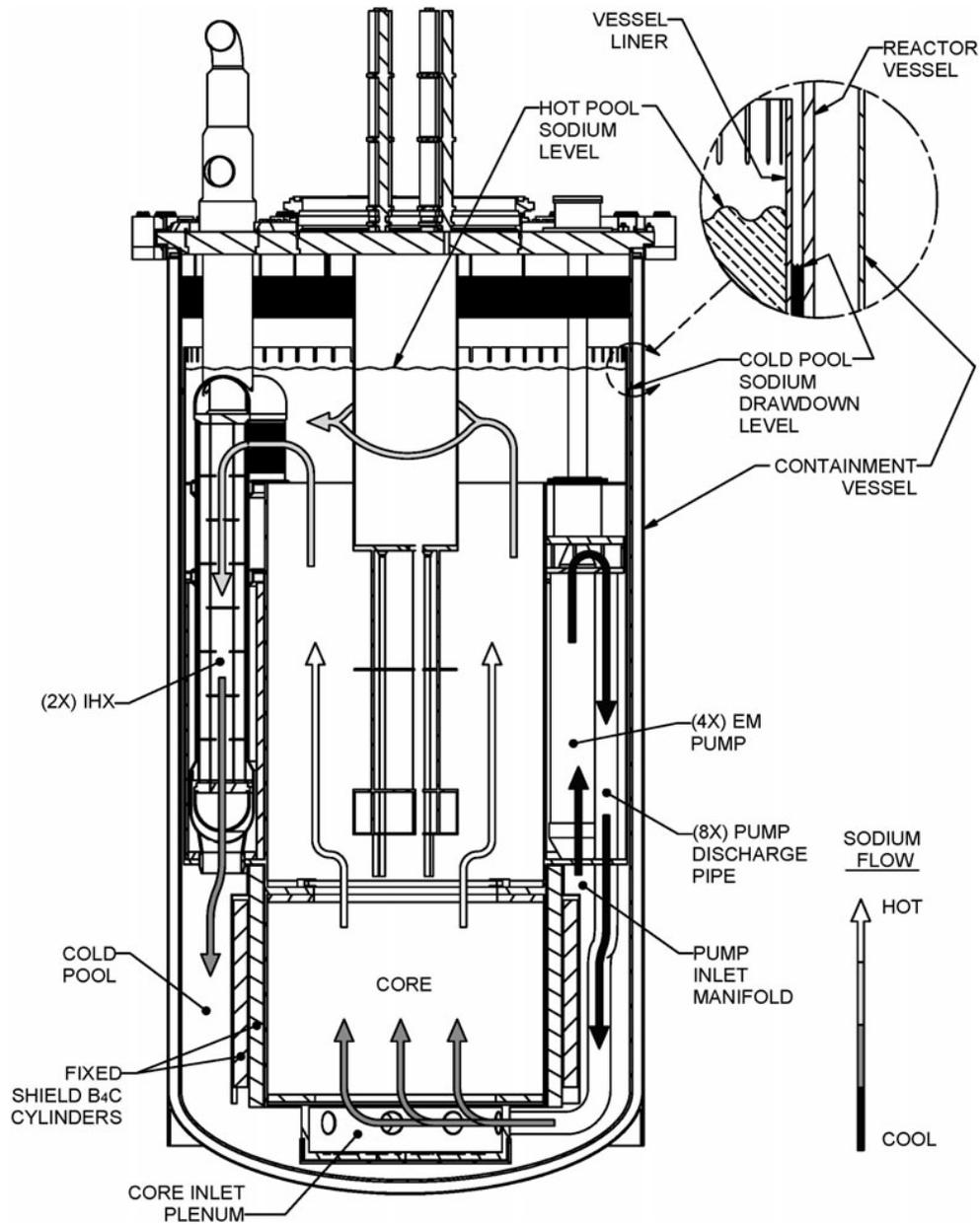
**Figure 3-7 PRISM Primary Heat Transport System [3-10]**
