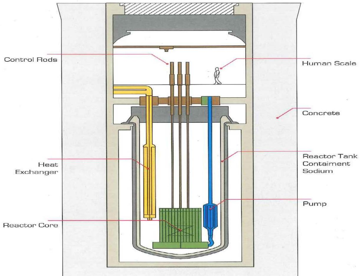
**Figure 2-1 ARC-100 Reactor**
