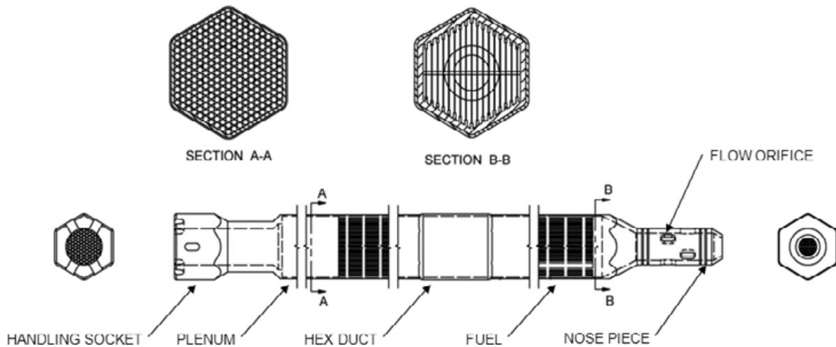
**Figure 3-4 PRISM Fuel Assembly [3-10]**
