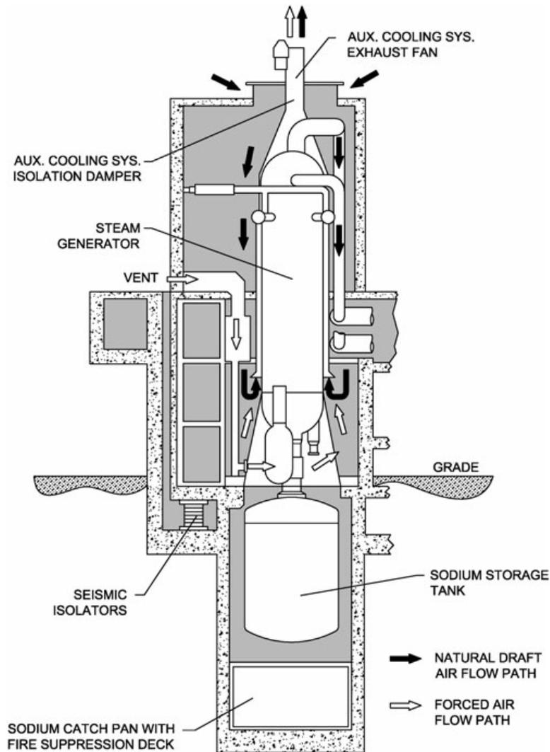
**Figure 3-8 PRISM Auxiliary Cooling System [3-10]**
