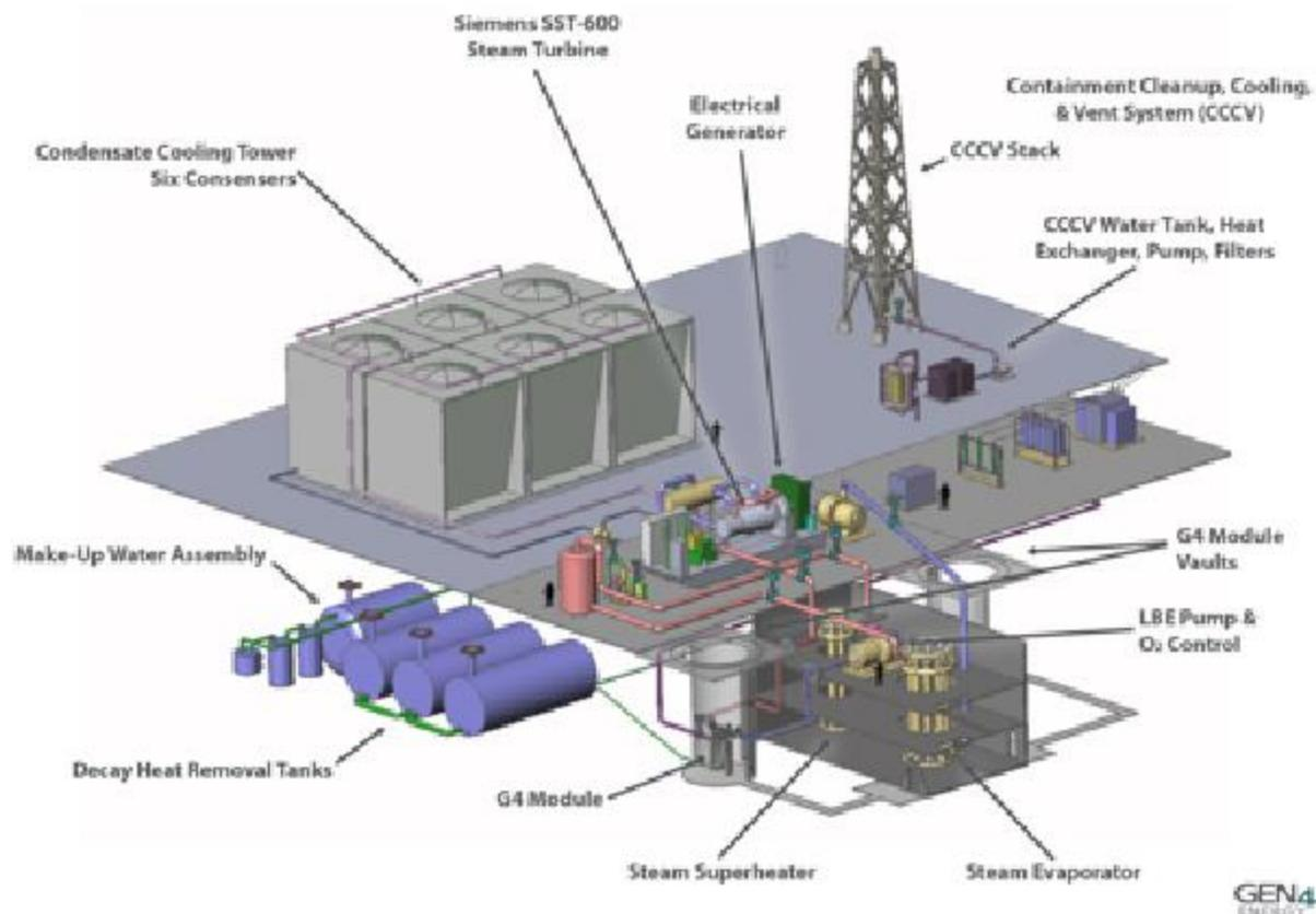
**Figure 2-3 Conceptual Drawing of G4M Plant**
