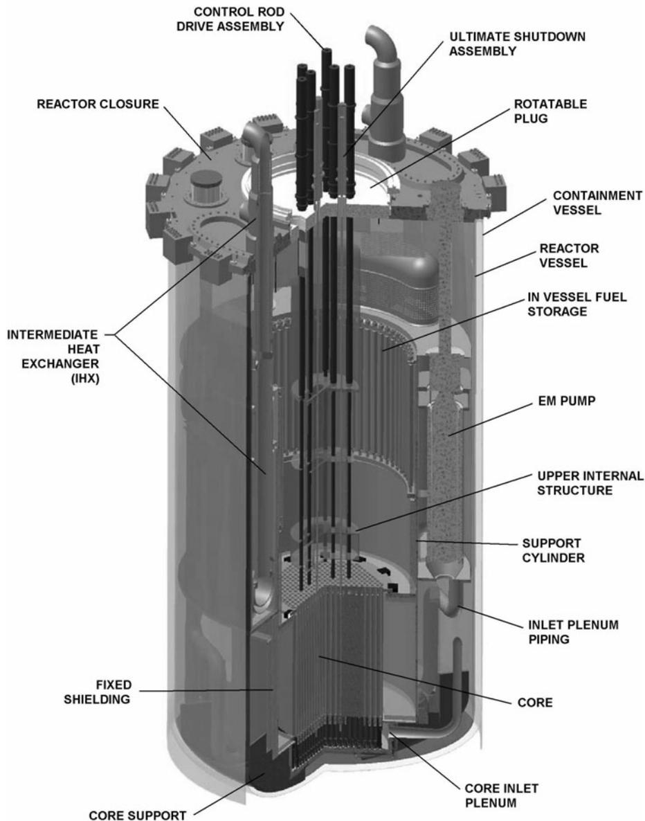
**Figure 3-6 PRISM Reactor Module [3-10]**
