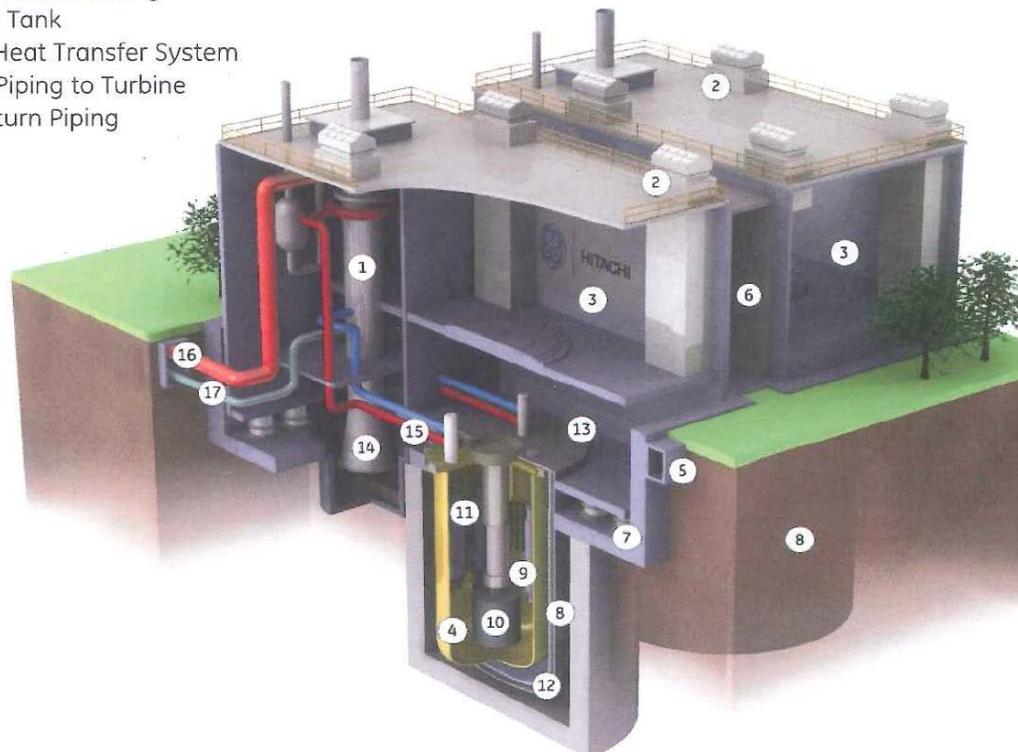
**Figure 2-2 PRISM Power Block**
