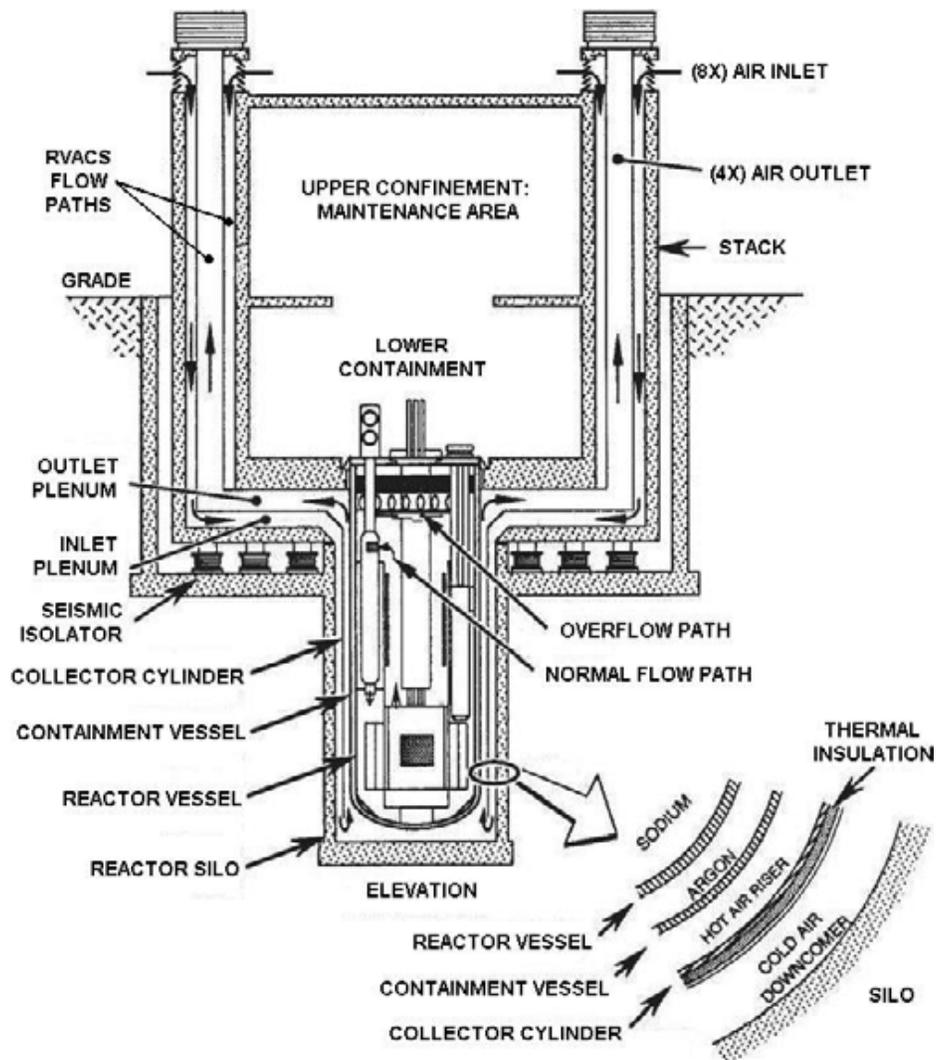
**Figure 3-5 Structural Components of Reactor Module and Containment [3-10]**
