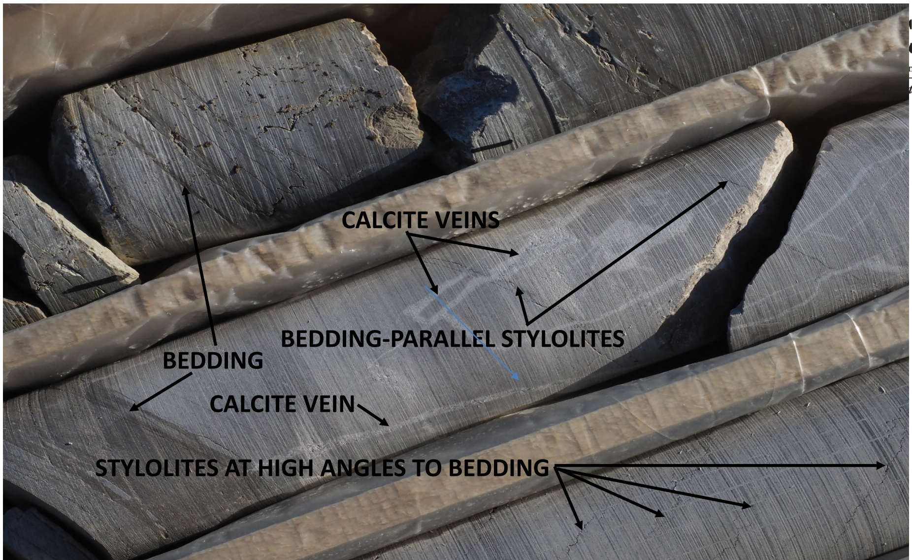
Shear-fracture zone penetrated in borehole MP-101. The stylolites must have developed at two different times because they form essentially perpendicular to the causative stress. (G. Stirewalt image, January 2018)
