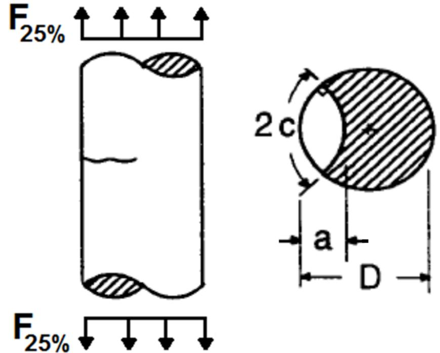
For constant displacement test: 25% load drop ( $F_{25\%}$ ) occurs when crack area equals 25% of original test specimen area.
