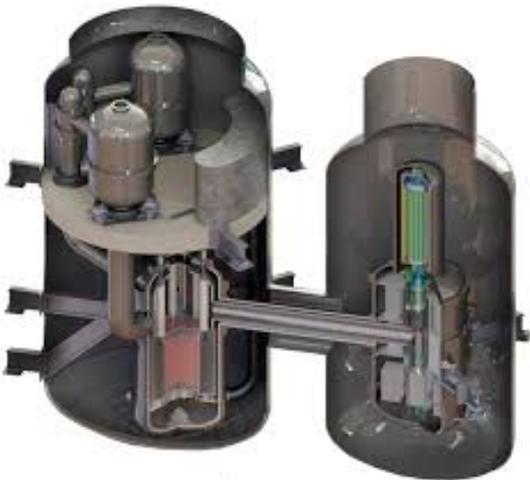
*Lead-Cooled Fast Reactors*
