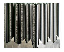
New **accident tolerant fuel (ATF) cladding**, conceived, developed, manufactured, and tested at ORNL, has been manufactured by Global Nuclear Fuels (GNF) into lead test assemblies, and shipped to Southern Nuclear Operating Company for trials in Edwin I Hatch plant. The FeCrAl cladding, called IronClad (see figure), will be the first developed through DOE's Enhanced ATF program to be installed in a commercial nuclear reactor. (February 2018)
