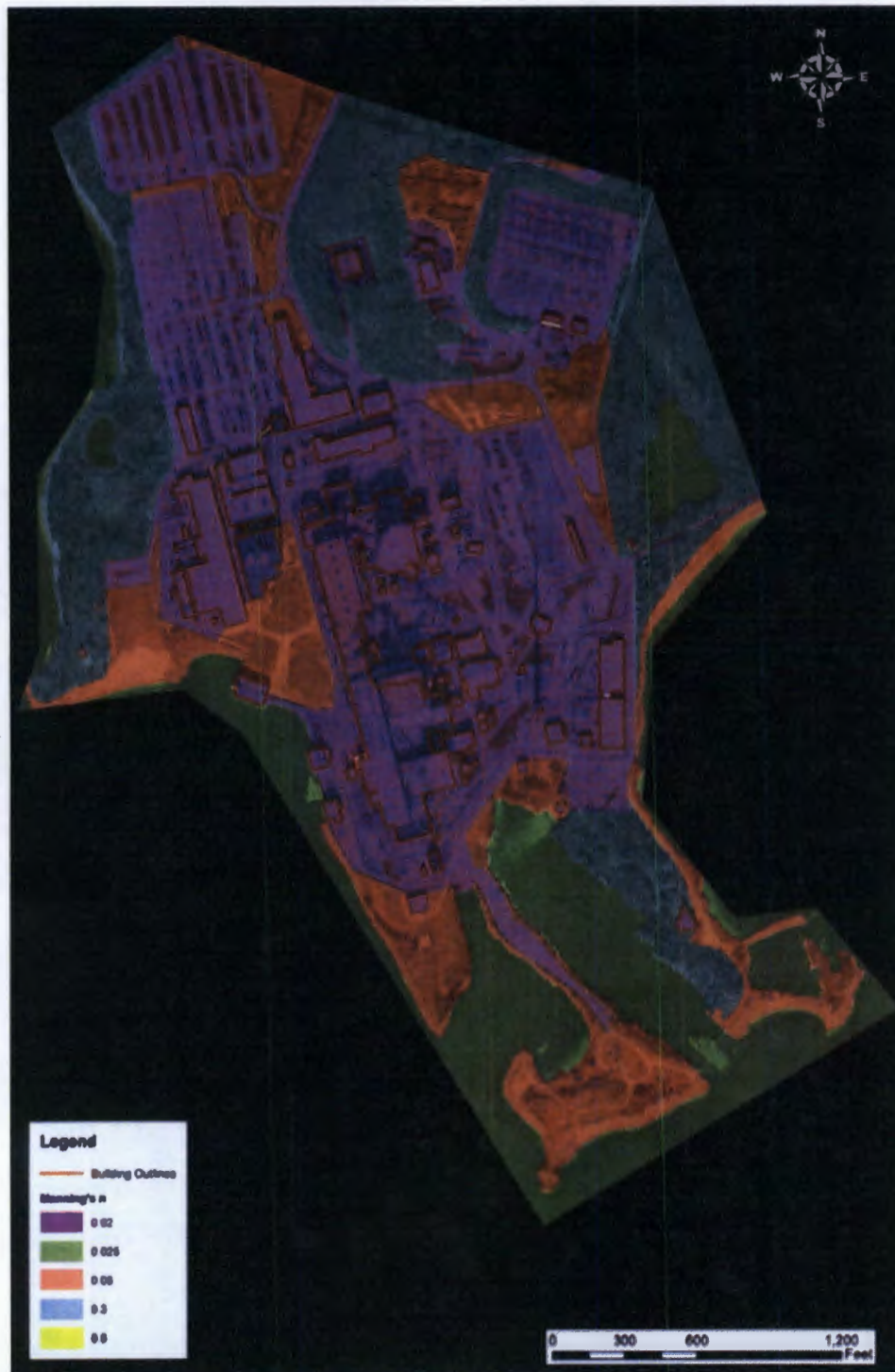
Figure 3.2-2. Manning's n values used in FLO-2D modeling of Millstone Power Station site. (Source: Dominion, 2015, Figure 2.1-4).
