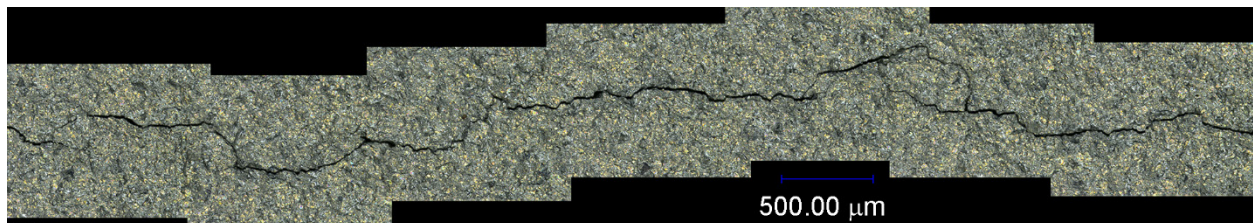
Figure C-1 Crack Segment File with Multiple Photos Stitched Automatically by the Stream Motion Software
