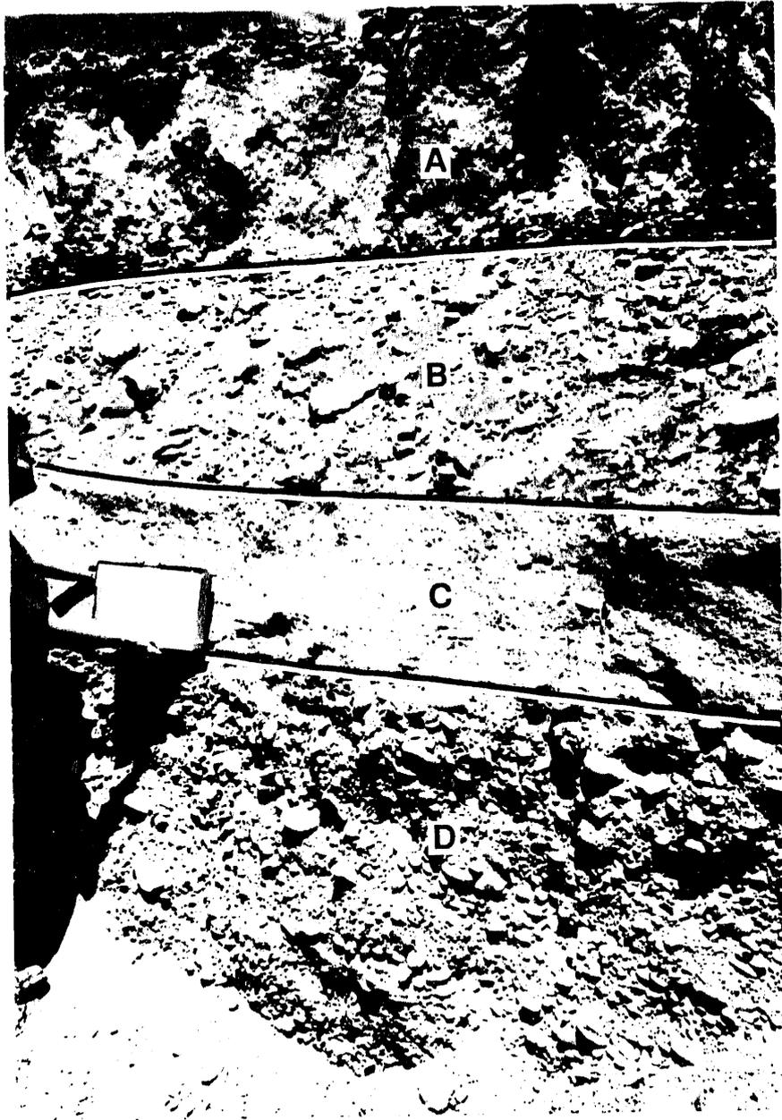
Figure 4.8. Multiple Layers at Pit 29. Two layers of predominantly sand and two layers of predominantly gravel are represented. Silt is locally concentrated along the top of layer D.
